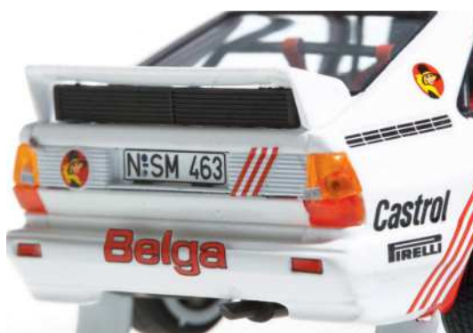
▲ The big radiator under the rear wing was a feature of 1985 Audi's quattro A2.
