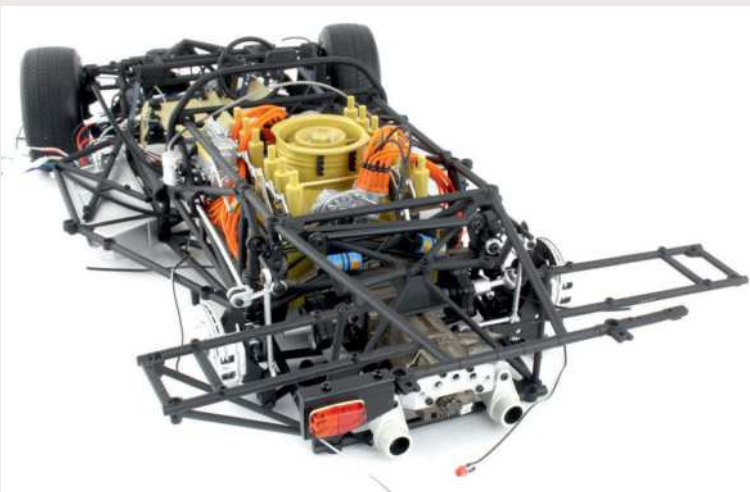
▲ With the engine now fully attached to the rear of the chassis, we've been able to continue building the spaceframe around it, to the point where we now have a rear light lens unit installed, but this is not yet connected to the wiring loom.
