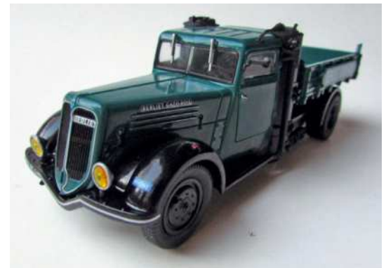
▲ In the thirties, due to a shortage of petroleum products, many vehicles will be converted to wood gas. Berliet will market its own system, "Gazo-bois". This VDANG 16 released in 1939 is equipped with it (issue 32).
