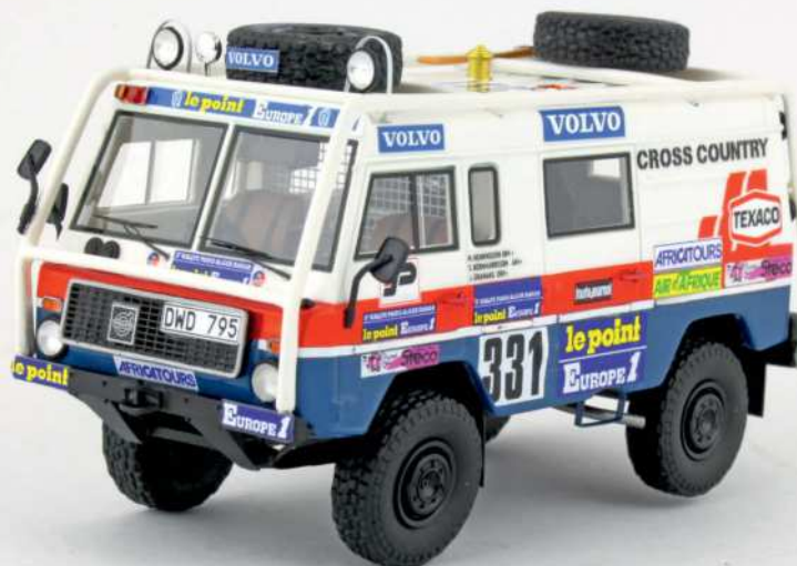
▲ The Volvo C-300 series origins can be clearly seen here, as it only received a few modifications before the event – the most noticeable, apart from the livery, being the roll cage welded to the outside of the body.
