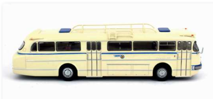
▲ Two sets of 'three-wing' doors denote this as the intercity variant (the suburban version had three sets of doors).
