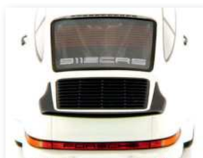
▲ The SC/RS features a black edge to the rear spoiler, helping to tell the two apart.
