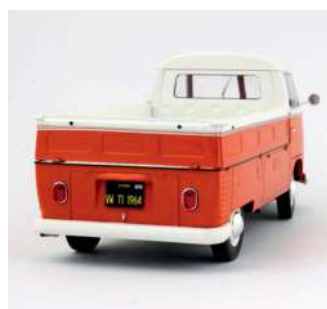
▲ The tailgate hinges down, held in place by retainers to either corner.
