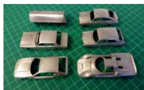
▲ A batch of six Superfasts stripped, buffed and ready for repainting.
