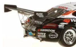
▲ The gigantic rear wing is one of the main features on this racing Cayman, allowed by the Nürburgring 24 hours regulations.
