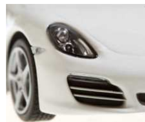
▲ Front air intakes are much bigger on the Boxster MkIII, to feed the radiators.
