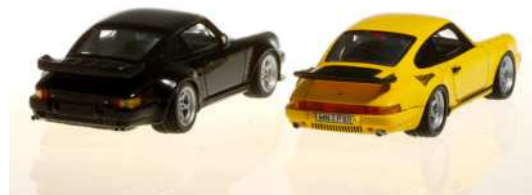
▲ Rear wing was much slimmer and the body narrower on the Yellow Bird, to reduce drag.
