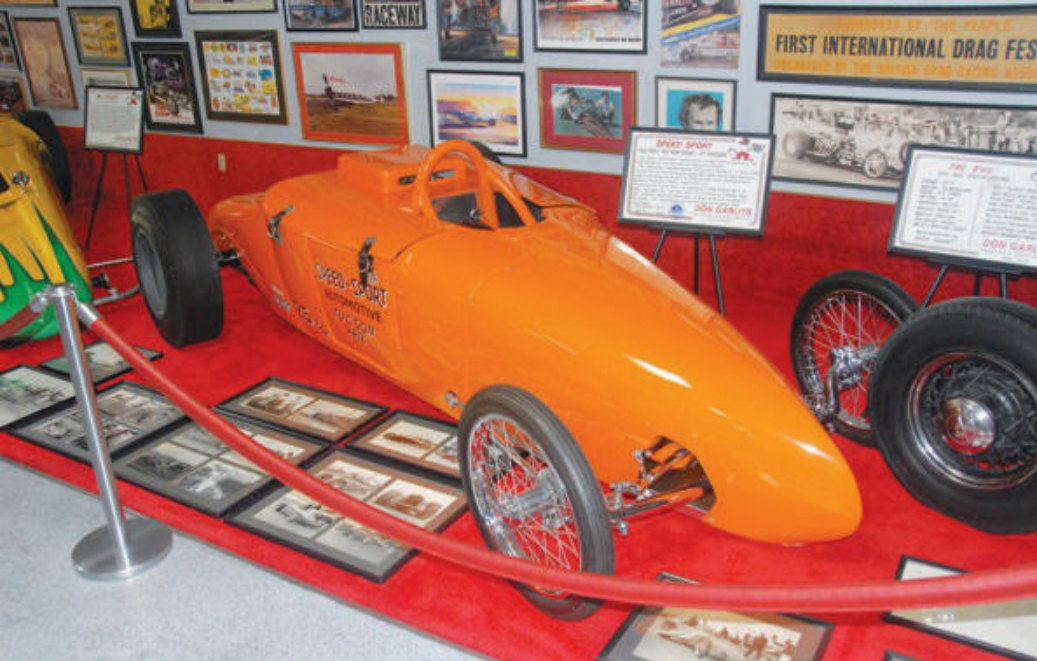
“Red” Greth’s famous Speed Sport Roadster ran in the Modified Roadster class. It was essentially a front-cockpit, short-wheelbase dragster with a Ford ’27T bucket utilized as a part of the bodywork. The car was never beaten in its class and often won Top Eliminator honors when it ran.
