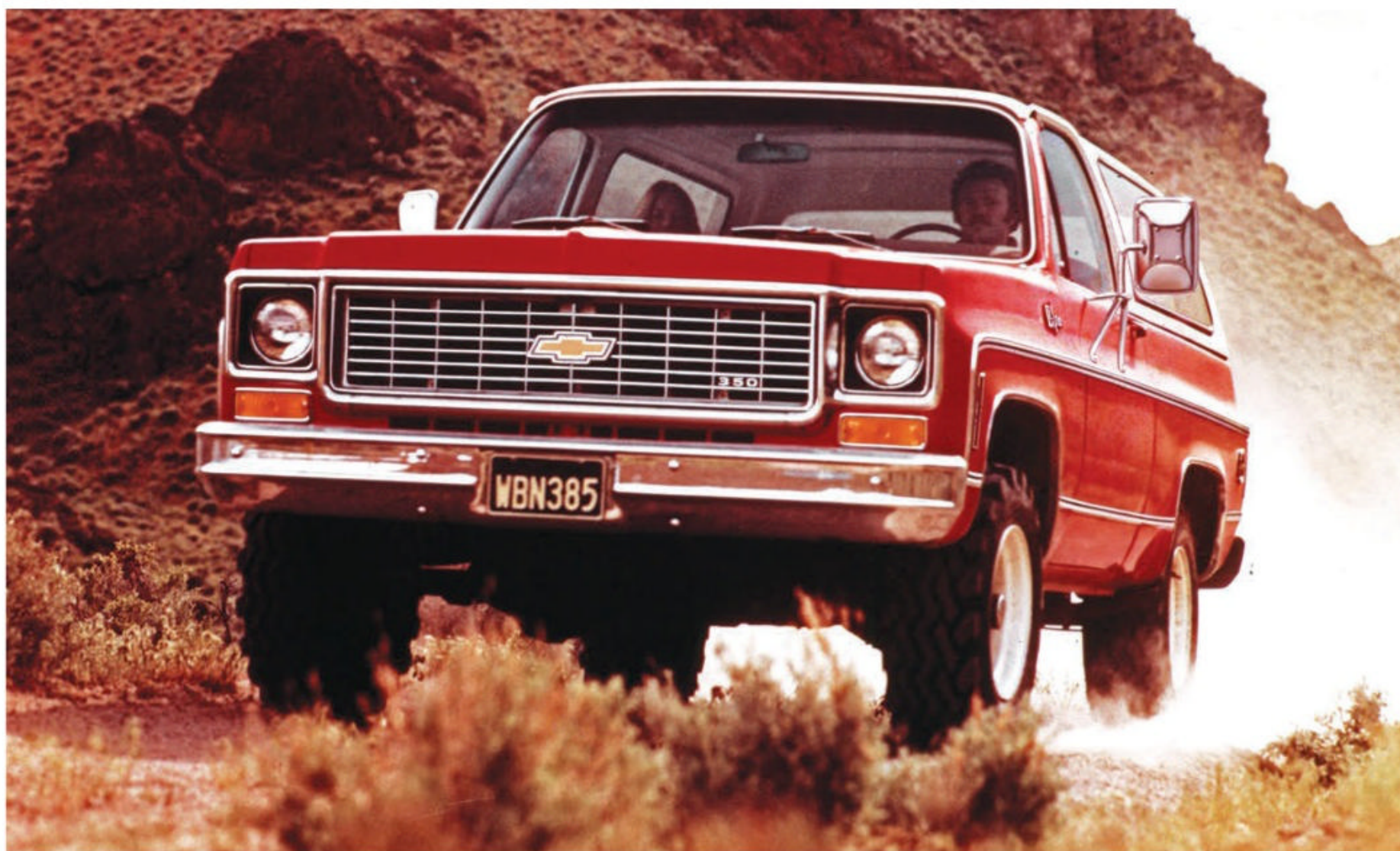
Early "Square Body" Blazers had round headlights and a full-length fiberglass roof. There were also plenty of off-road goodies offered for them like a brush bar, lights, and a winch.
