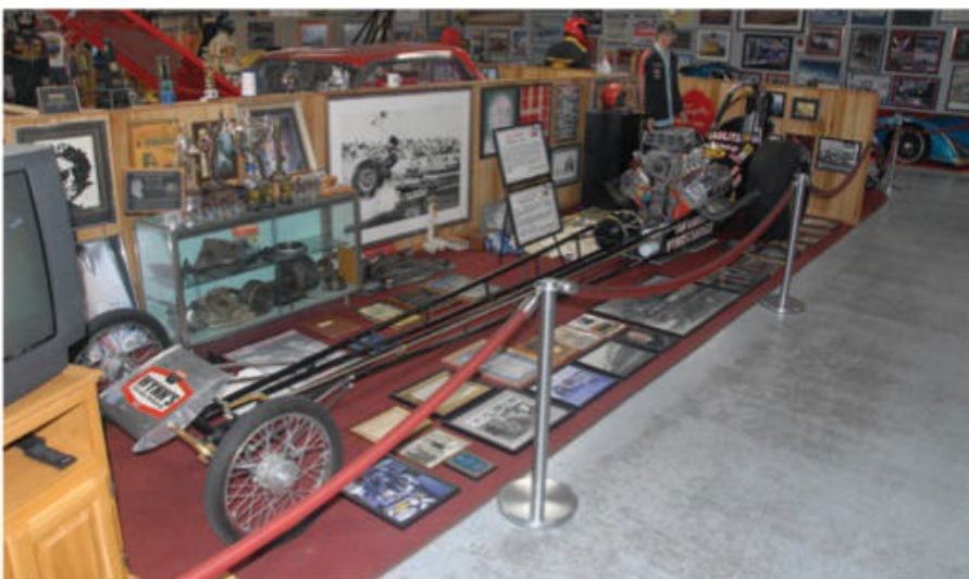
Swamp Rat 13 was the infamous car that blew its transmission on the starting line at Lions Drag Strip in Long Beach, California in 1970, injuring Don and causing him to completely rethink the front-engine "slingshot" design for dragsters.
