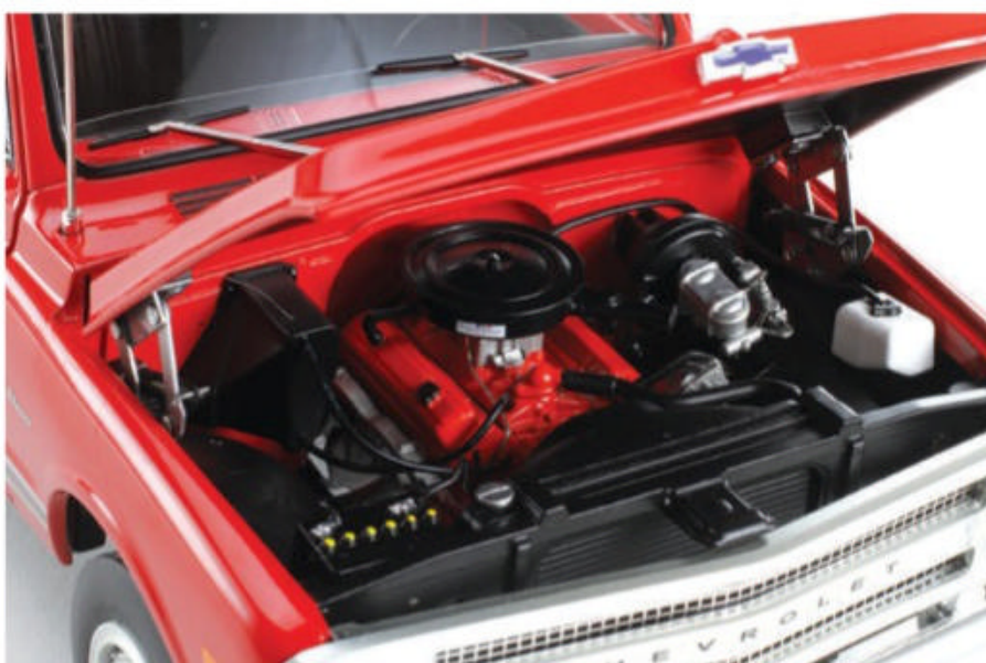
Blazer has the most desirable engine offered in 1969—the 255hp 350 V8. I love the thin-gauge wire used for brake and fuel lines!
