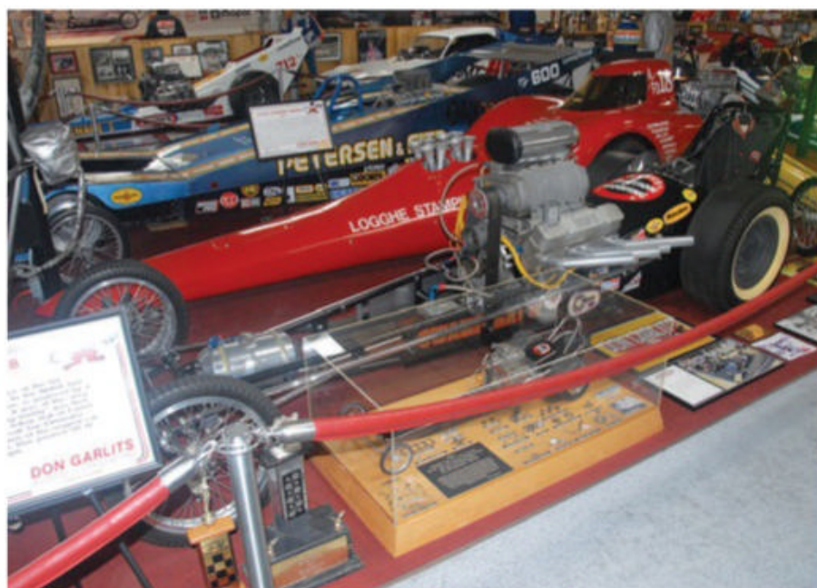
Shown here are Swamp Rat 4B and the Logghe Streamliner. Two iterations of the same design philosophy: light weight. Don's car uses an all-aluminum, blown wedge-head Mopar engine and the Logghe Stamping car uses an injected small-block Chevy. Logghe gained great fame building drag racing chassis and the injected SBC car was incredibly successful, put away much more powerful (and heavy) blown Chrysler-powered competitors.
