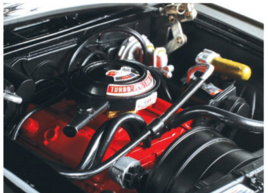
The Monte's big 454 has a couple of cool extras. There is air conditioning and the bronze-colored tube on the left-side fender is the compressor pump for the Automatic Level Control system.
