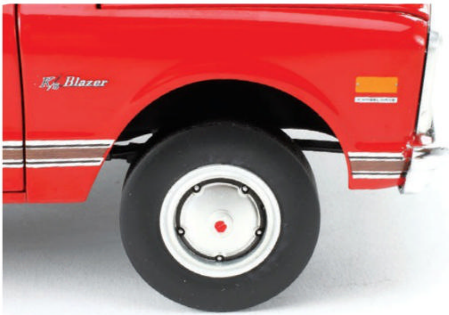
The white-painted steel rims have non-descript P01 wheel covers with the manually locking hubs poking through them.
