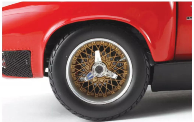
The SVR wears some of the widest tires ever installed on a Lamborghini—345/35-R15 Pirellis on beautiful BBS center-lock wheels.
