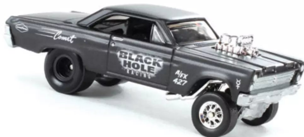
The '65 Mercury Comet Cyclone is a piece of drag-racing history, and the team version sports a formidable blown, injected 427 and cool-looking fender-well headers.
