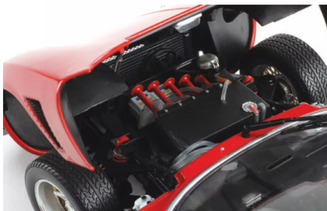
A racing-style fuel cap is cut through the bonnet and it flips up. Under it sits the widened double wishbone suspension, bright red Koni coil-over dampers, and the fuel tank.
