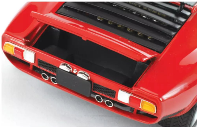
The trunk is shallow, as the racing exhaust takes up most of the space in the rear end.
