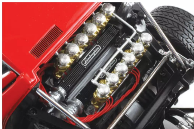
Kyosho does a great job with the extensively modified V12 with its open-throat Weber carbs, tubular exhaust headers, and a host of internal mods.
