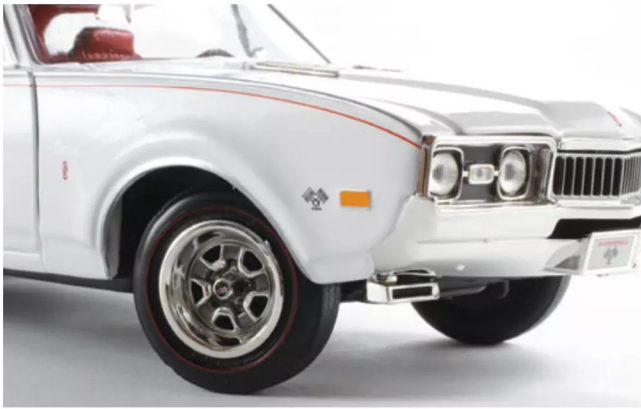
In 1968 the "Ram Rod 350" emblem appeared on the fenders but not on the engine itself. For the '69 model it moved to the air cleaner lid, like on the W-30. The '68 car has the familiar Oldsmobile SSII wheel pattern with redline tires.
