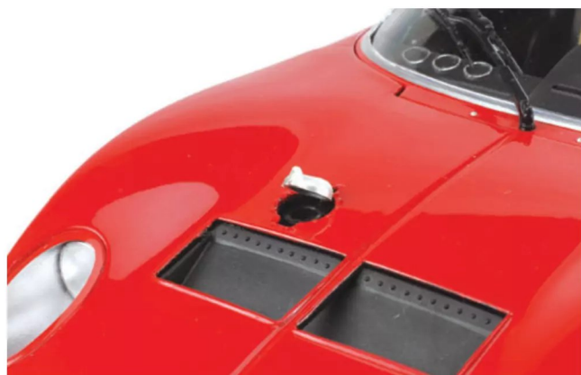
A racing-style fuel cap is cut through the bonnet and it flips up. Under it sits the widened double wishbone suspension, bright red Koni coil-over dampers, and the fuel tank.
