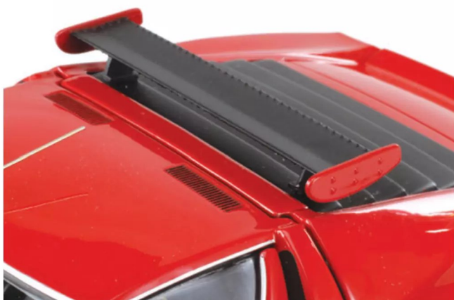
The most conspicuous modification in creating the SVR was the addition of the large wing on the trailing edge of the roof.
