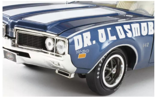
The minor differences between the '68 and '69 styling focus on the grille and headlights. The '69 car pushed the lights together and separated the grille with a center bar. Both model years have the air scoops for the ram-air system mounted under the bumpers.
