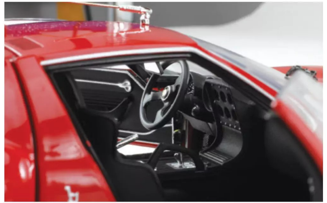
As part of the SVR conversion, special Recaro racing seats were installed with four-point safety harnesses were installed. Kyosho recreates the harnesses with fabric belts and etched metal harnesses.
