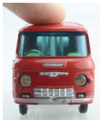
ABOVE The simple but effective Trans-o-lite "flashing" headlamps are operated by covering and uncovering the top of the driver's cab unit.
