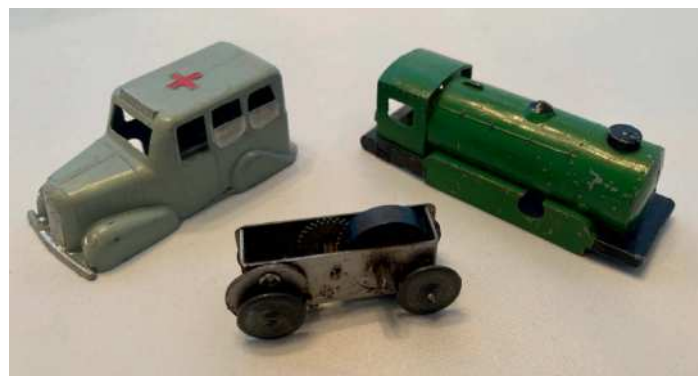
ABOVE Interchangeable clockwork mechanism could be fitted to a Kay locomotive or to a vehicle.
