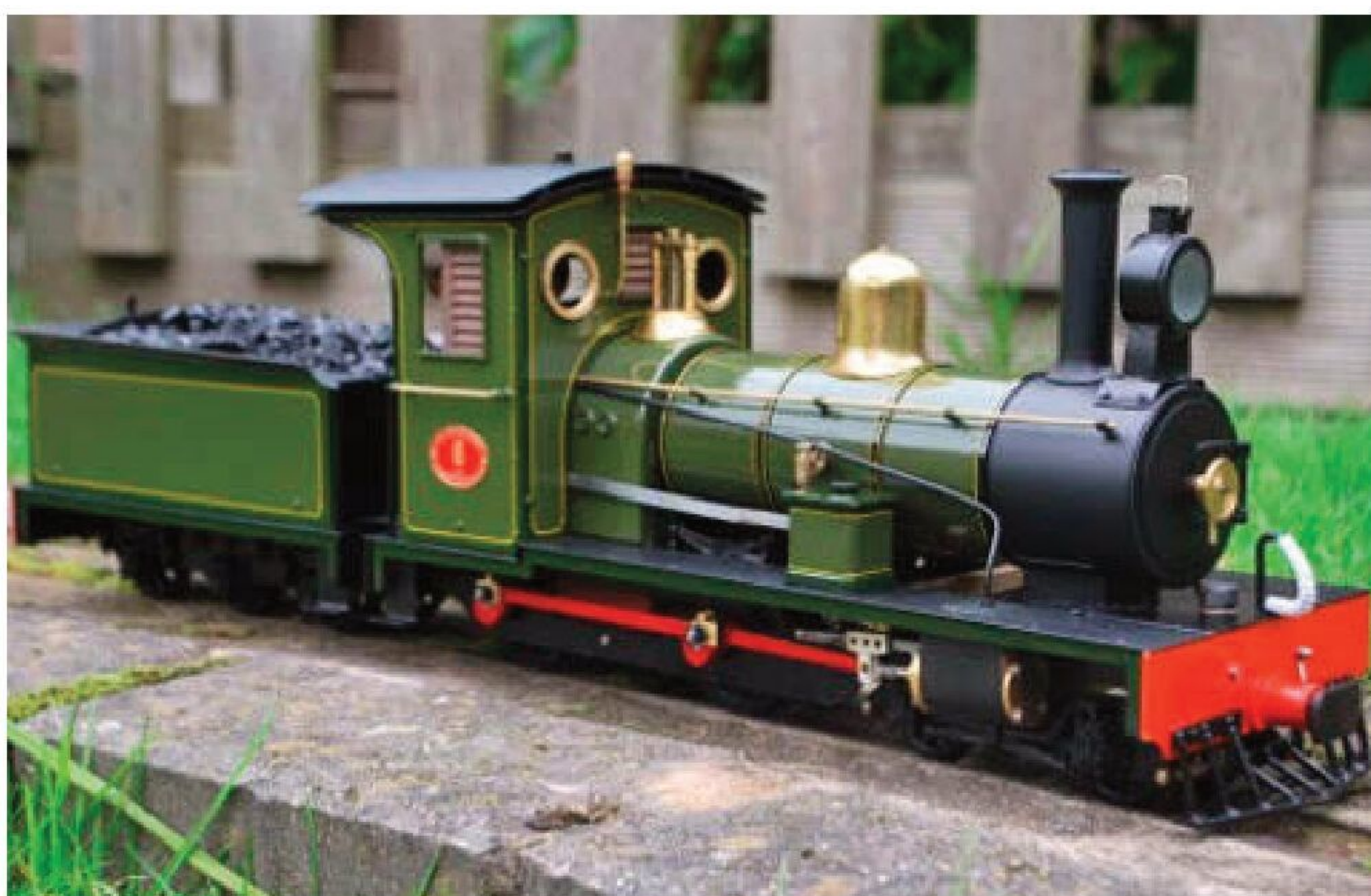
ABOVE Archangel Models NG6 ex-Beira Railway Falcon 4-4-0 tender locomotive, gas fired gauge O with slip eccentric valve gear.
