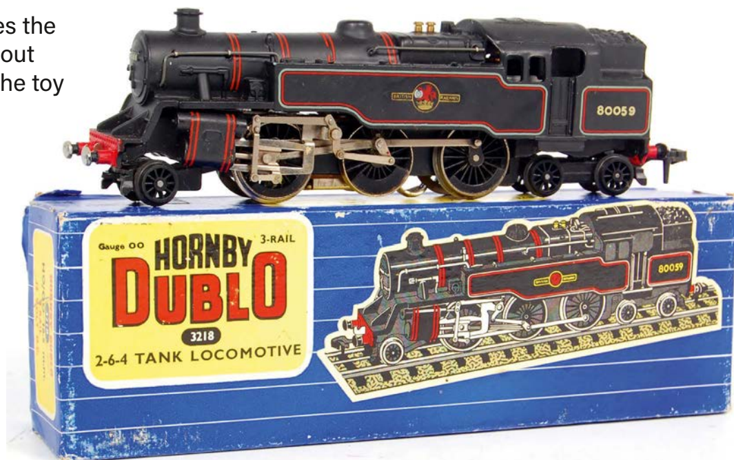
ABOVE The 3 rail version of the BR standard 2-6-4 tank is only distinguishable from the 2 rail 80033 by the number. However the chassis has 3 rail pickups.
