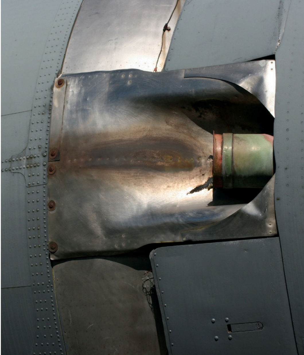
Stainless steel plates do not stay stainless for very long. Note the variety of colours.
