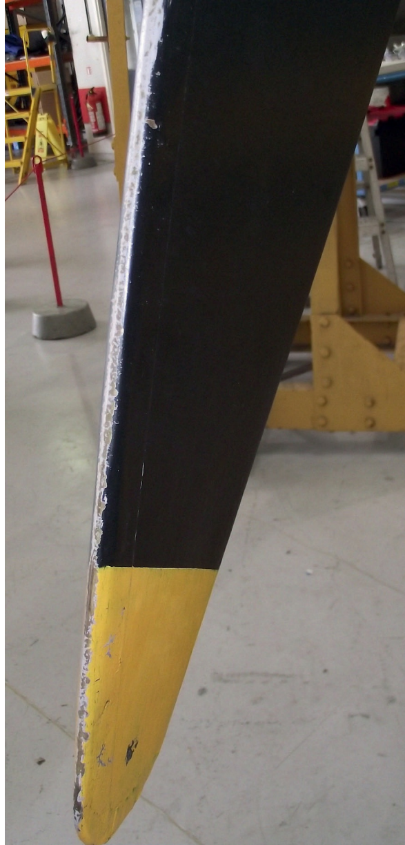
Another propeller with leading-edge erosion and chipped paint.
