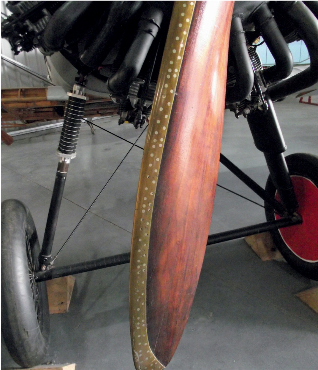
A wooden propeller fitted to a Gloster Gamecock in the Gloucestershire Aviation Collection. Note the brass-sheathed leading edge.
