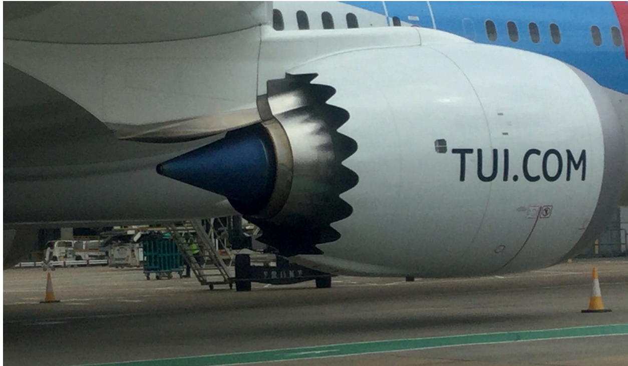
One of the later aircraft engines showing the blue stainless steel cone. These can also have a purple tone to them. IAN BROWN
