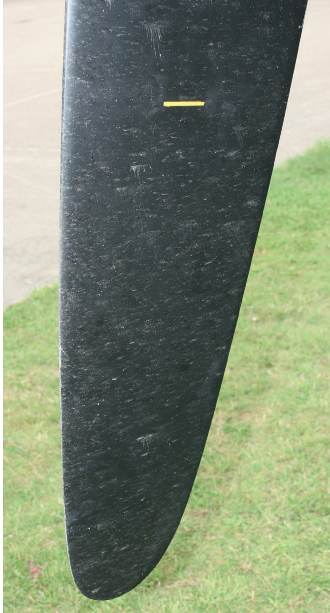
One of the P-40 propeller blades' rear faces, showing erosion on the leading edge and pitting on the rear face. The pitting is caused by small stones and mud picked up off the runway during take-off and landing. There are also a fair number of bug splats amongst the pitting.
