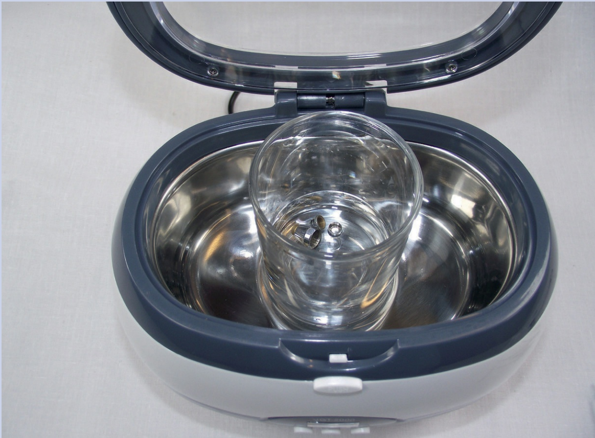
Airbrush parts are in solvent in the glass tumbler, and the tumbler is placed in water in the ultrasonic bath.
