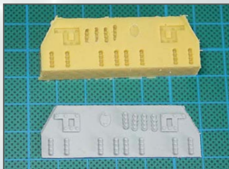
My own silicone moulds and resin copies for the hull mine roller mounting points.
