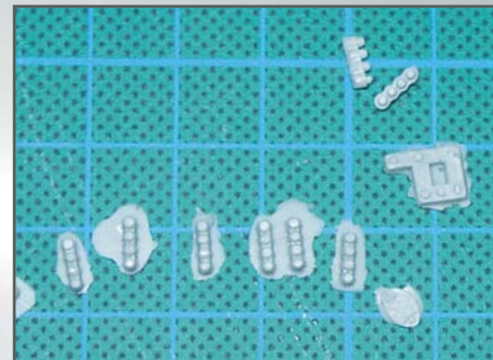
Small parts like this are easy to cast with a basic moulding kit and can be used multiple times.
