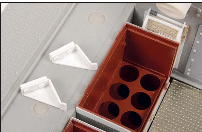
These two brackets sit between the floor ammunition bins and are designed to stow one of the folding two round ammunition crates to maximise ammunition stowage.
