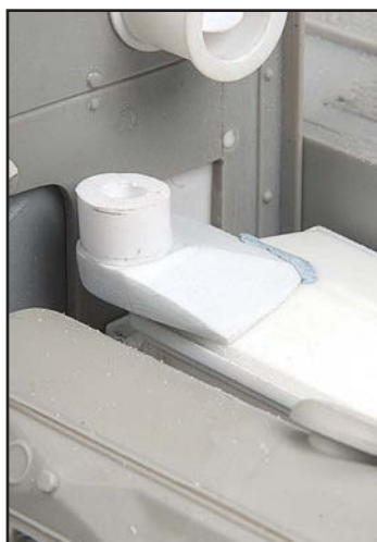
The airfilter connects to the engine via a large diameter pipe, the outlet for this has to be rather awkwardly offset to avoid the crew heater pipe above it. This results in a very complex piece of geometry for the connecting sheet metal.
