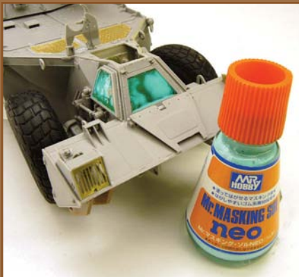
A good coating of Mr. Masking Sol was allowed twenty four hours to dry before airbrushing the base-coat, an old favourite; Humbrol Desert
