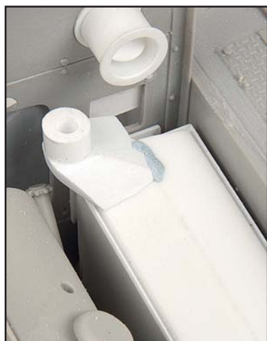
The airfilter connects to the engine via a large diameter pipe, the outlet for this has to be rather awkwardly offset to avoid the crew heater pipe above it. This results in a very complex piece of geometry for the connecting sheet metal.
