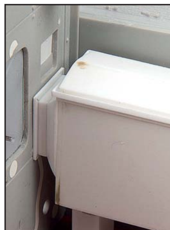
The new trunking fits over the lower of the two vents on the firewall like this.
