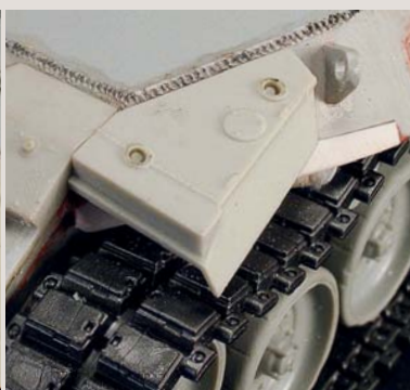
For the Legends conversion set to fit, the kit's fenders need to be removed, just as on the real tank. With the gaps filled, the legends resin nose piece is attached to the hull.
