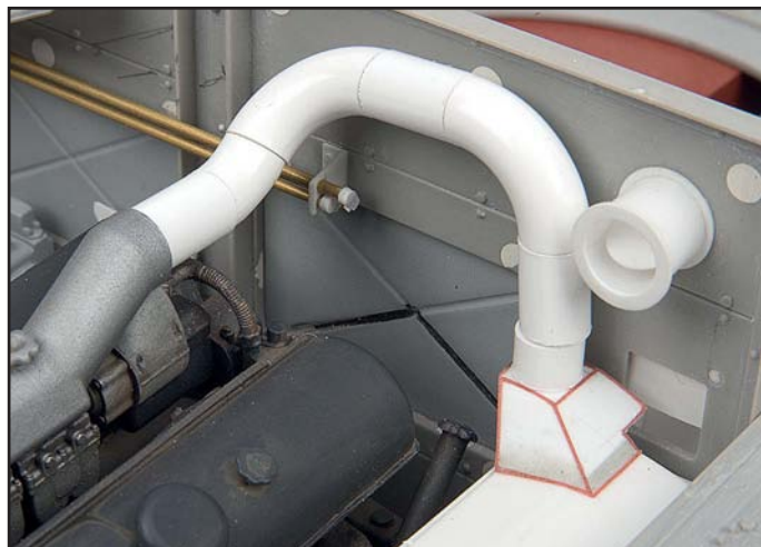
I had difficulty in finding a suitable diameter of rod to make the pipe but eventually I sourced an architectural modelling product which offered the correct diameter and an assortment of different elbow joints which made the process much easier. www.ema-models.co.uk
