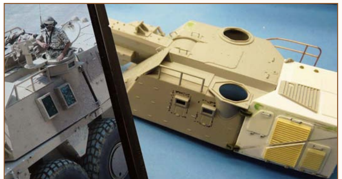
The export model also has larger armoured glass frames on the turret side.
