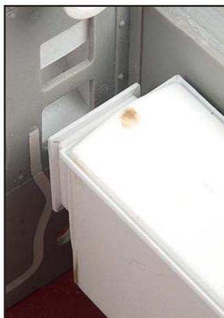
The new trunking fits over the lower of the two vents on the firewall like this.
