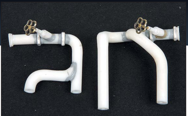
The handwheels were fitted to brass rod shafts and then added to the valves.
