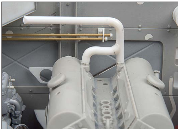
The airfilter pipe has to fit around one of the water pipes connecting the engine to the radiator so the basic shape of this pipe was established in order to check this. The bends in the rod were made by heating the required area over a small candle flame.
