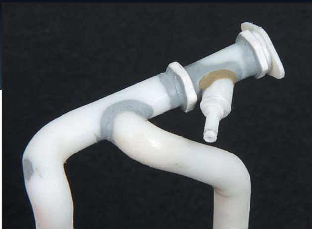
The valves were further detailed with the handle shafts which were drilled in preparation for fitting the handwheels and the valves were glued onto the pipes along with the flange to connect with the radiator, making certain that they fit correctly.
