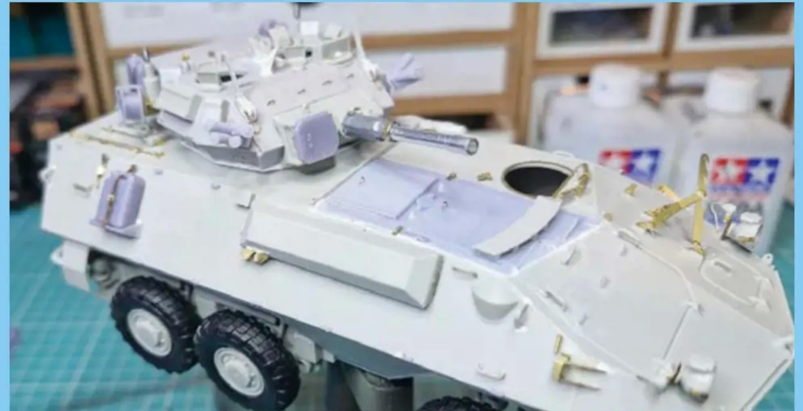
Trackjam engine deck added with a small amount of filler. The new engine means that this differs from the Swiss hull. Turret and kit wheels added. The kit wheels were later replaced with 3D printed ones.
