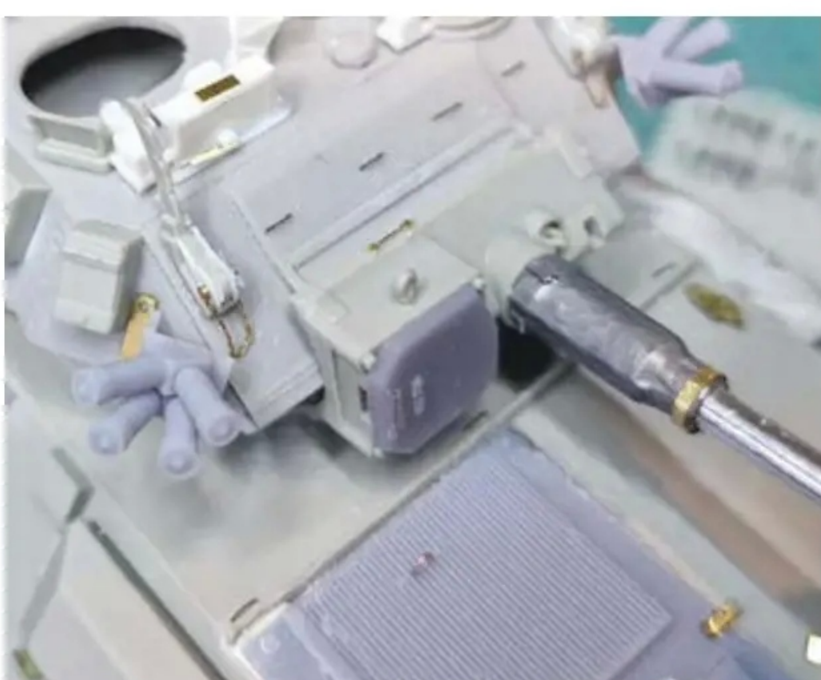
Darker grey parts are all 3D printed. Canvas cover added with lead foil to the lower gun barrel.
