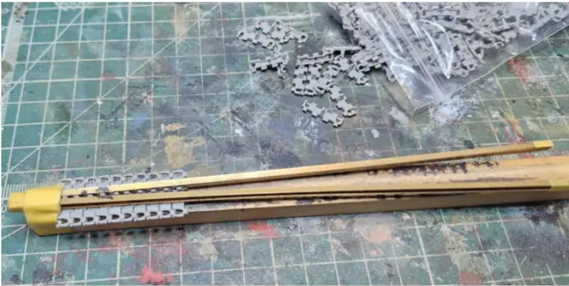
Using my homemade track building tool to put the plastic tracks together
