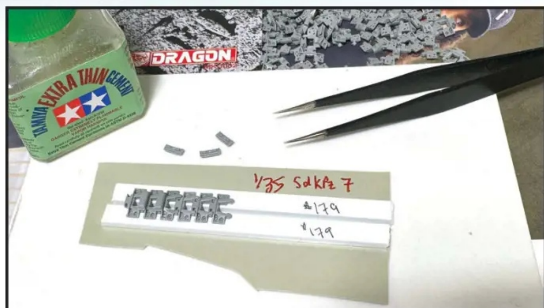
I made my own track guide tool out of Evergreen styrene strips glued to a styrene base, to assist in the assembly of the small fragile Dragon tracks.
