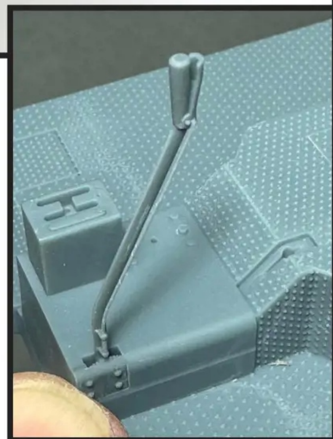
4 The simplified hand brake lever was replaced with my own corrected version along with gear shift.
