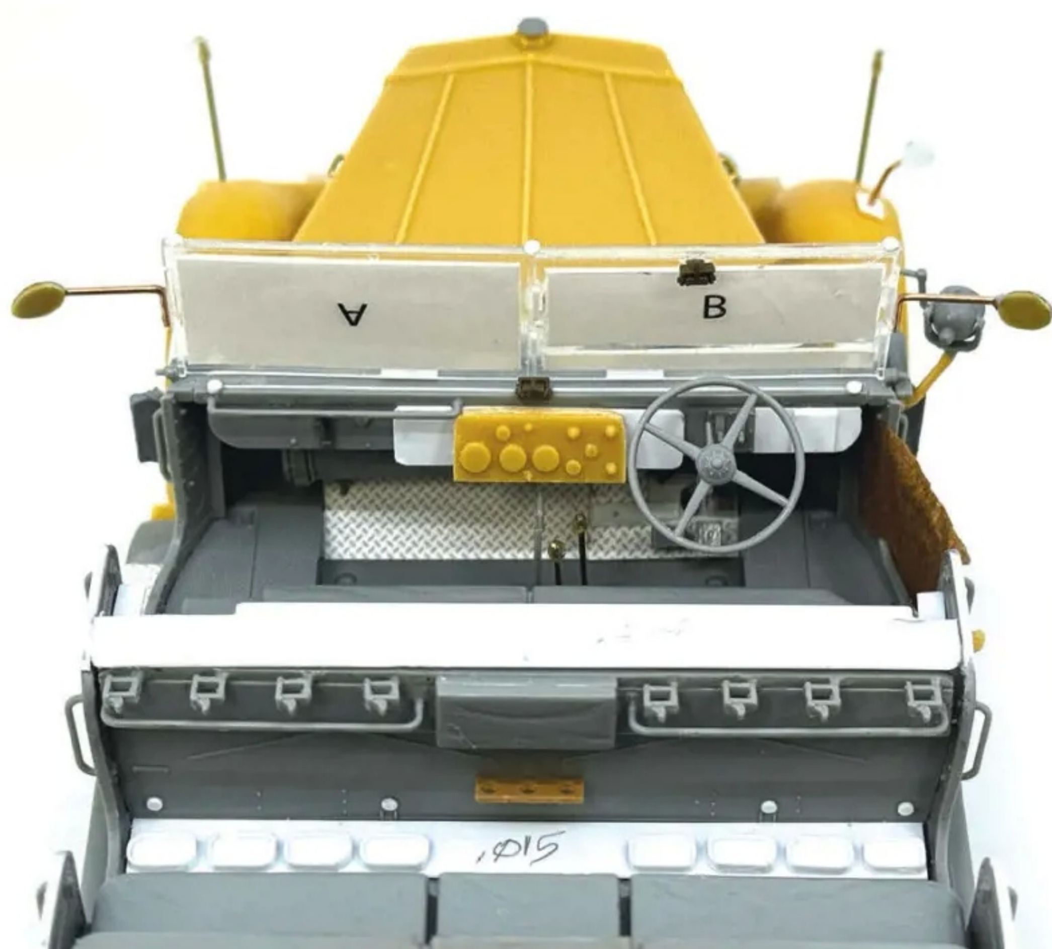
This photo shows all the details in the forward cab area: 1) switch to right-hand drive with old Criel Breda kit instrument panel and some styrene panels added; 2) new shift gear handles using styrene rod and a dab of 5-minute epoxy glue for the knobs; and 3) miscellaneous windshield details.
