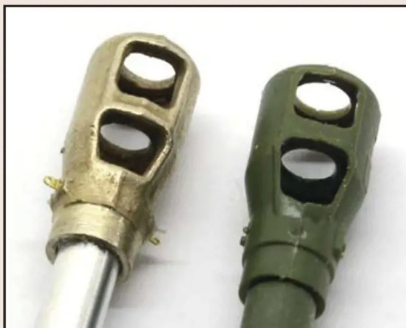
Unfortunately, Zvezda has once again included a longitudinally split muzzle brake in the new kit. The one from ABER is significantly better.
