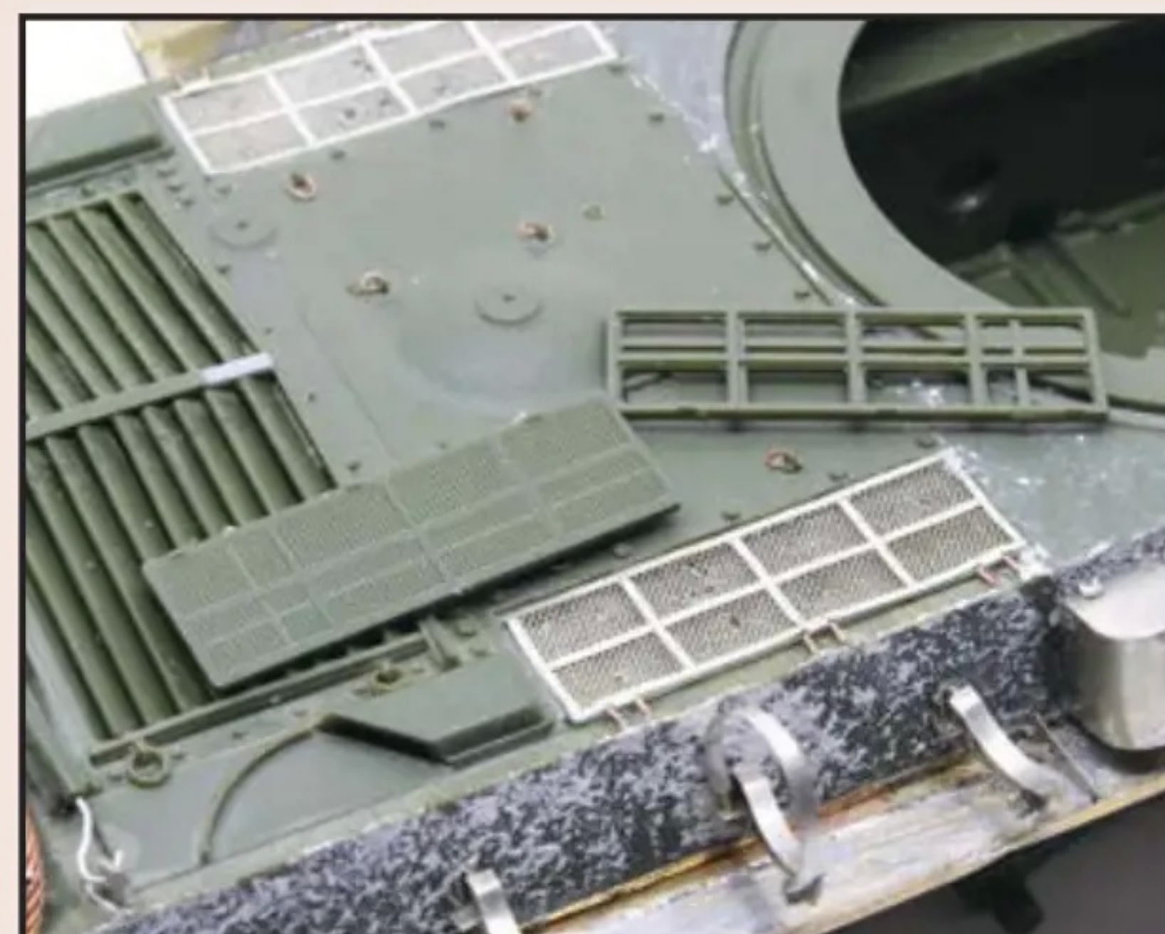
The plastic engine grilles from the kit are unusable. Purchasing photo-etched grilles is unavoidable.
