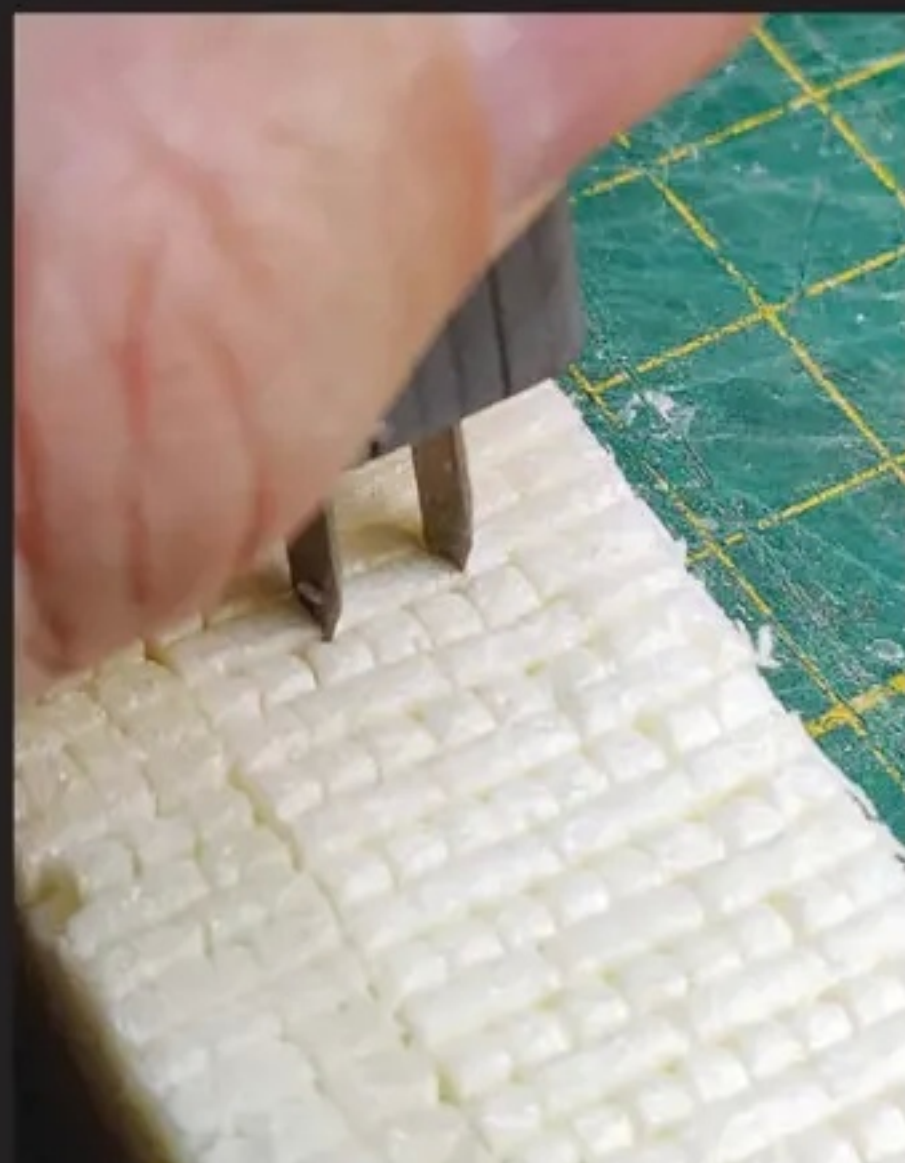
Using the described tool, making brick walls becomes easier. By using different blade distances one can vary the brick sizes.
