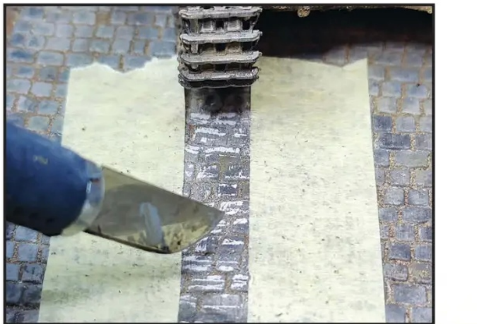
The track traces on the street a simply done by scraping the surface with a scalpel blade, an advantage from using modelling clay.
