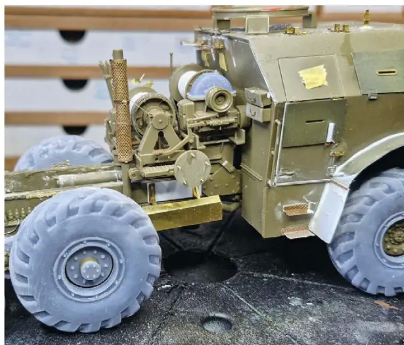
The spare tyre was left off as per the reference images, so threaded bolts had to be added.
