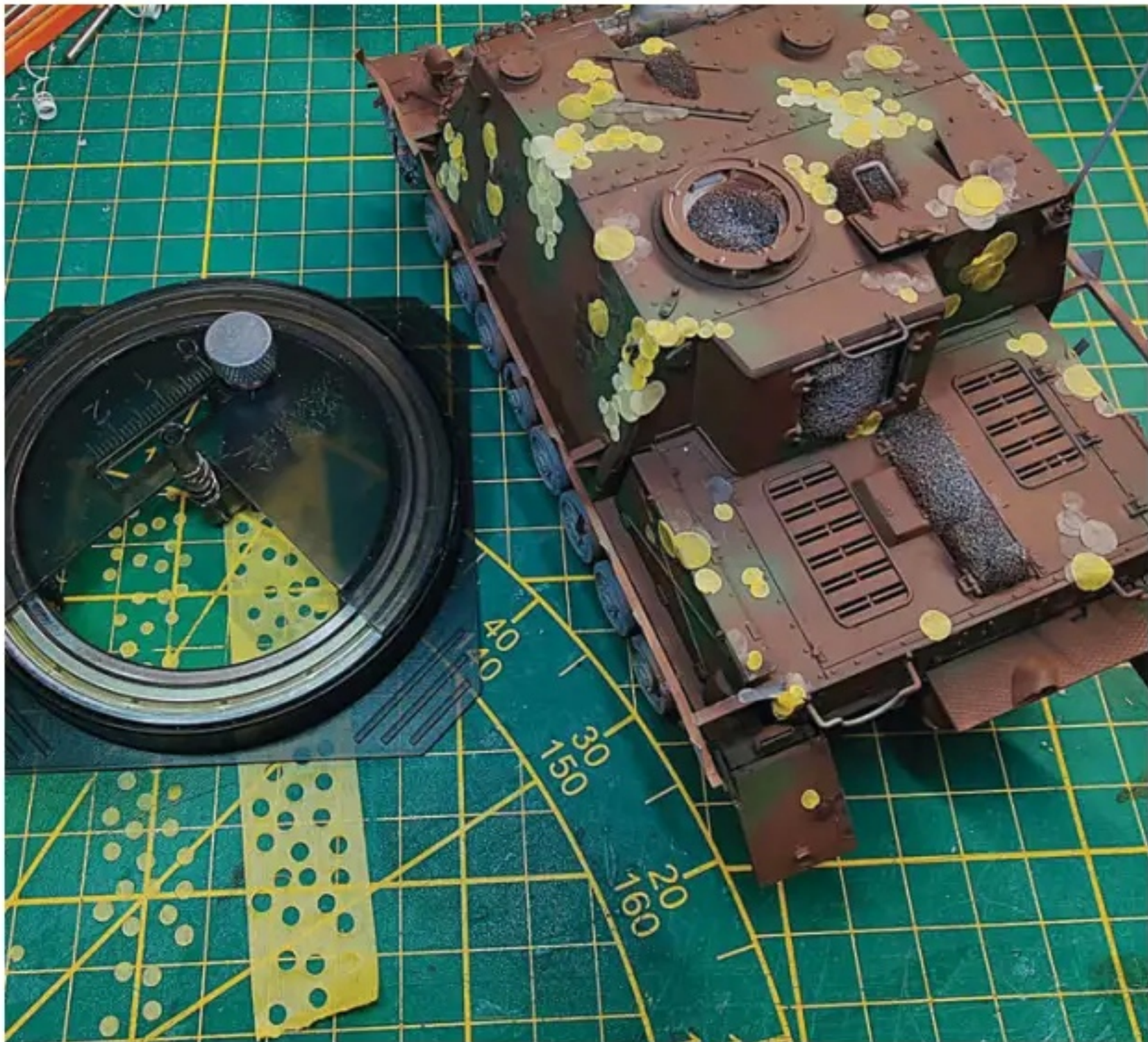
Cutting discs in different sizes with a circle cutter is easier.
