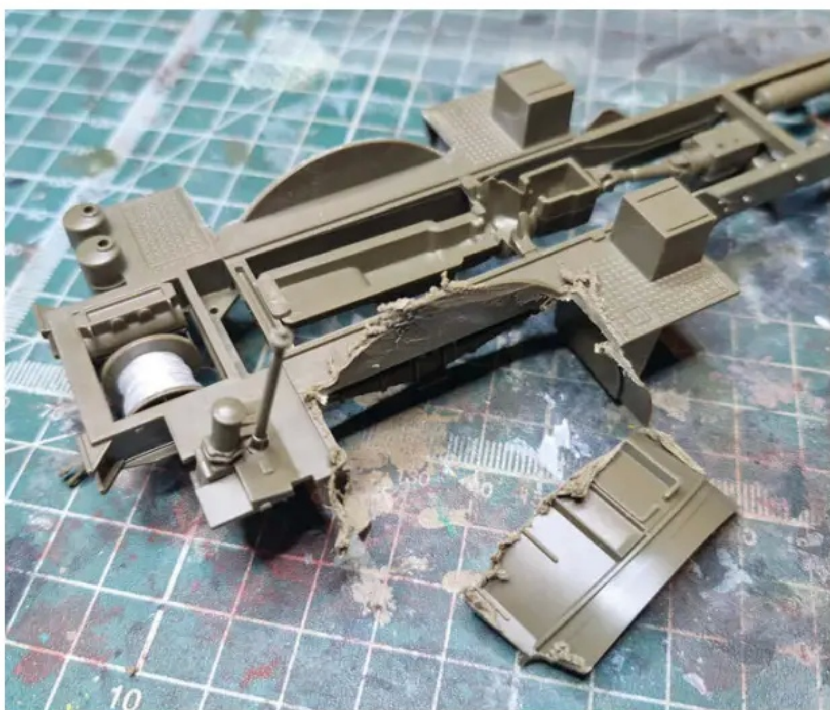
First cuts! Removing the sides of the fenders.
