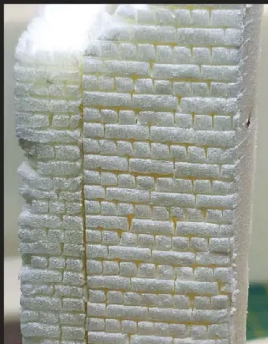
Using the described tool, making brick walls becomes easier. By using different blade distances one can vary the brick sizes.
