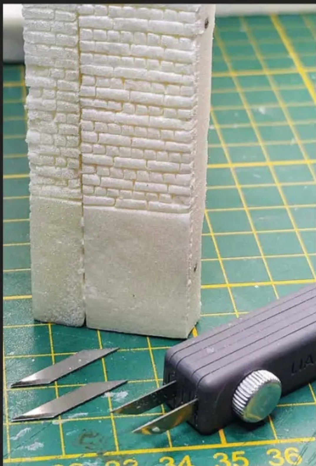
Using the described tool, making brick walls becomes easier. By using different blade distances one can vary the brick sizes.
