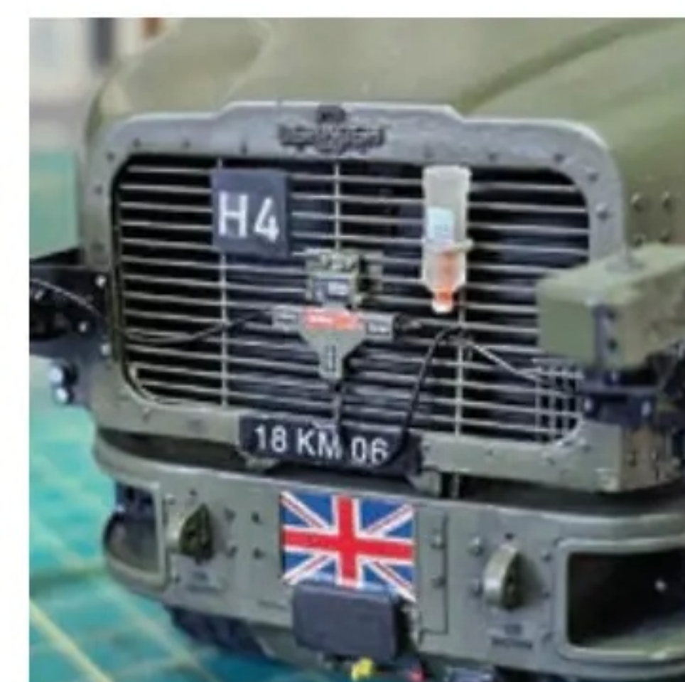
Front end detail. The clear plastic bottled carried a glowstick for night time identification.
