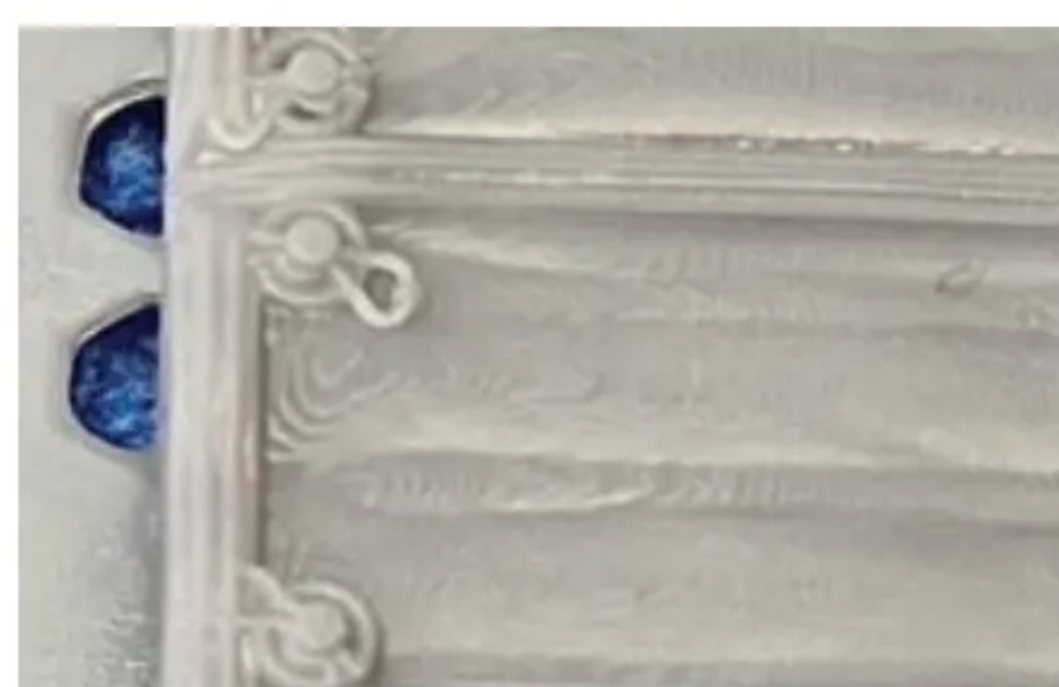
The detail achievable with 3D printing is amazing, but here you can also see the layers from the printing. This can be tidied with light sanding.
