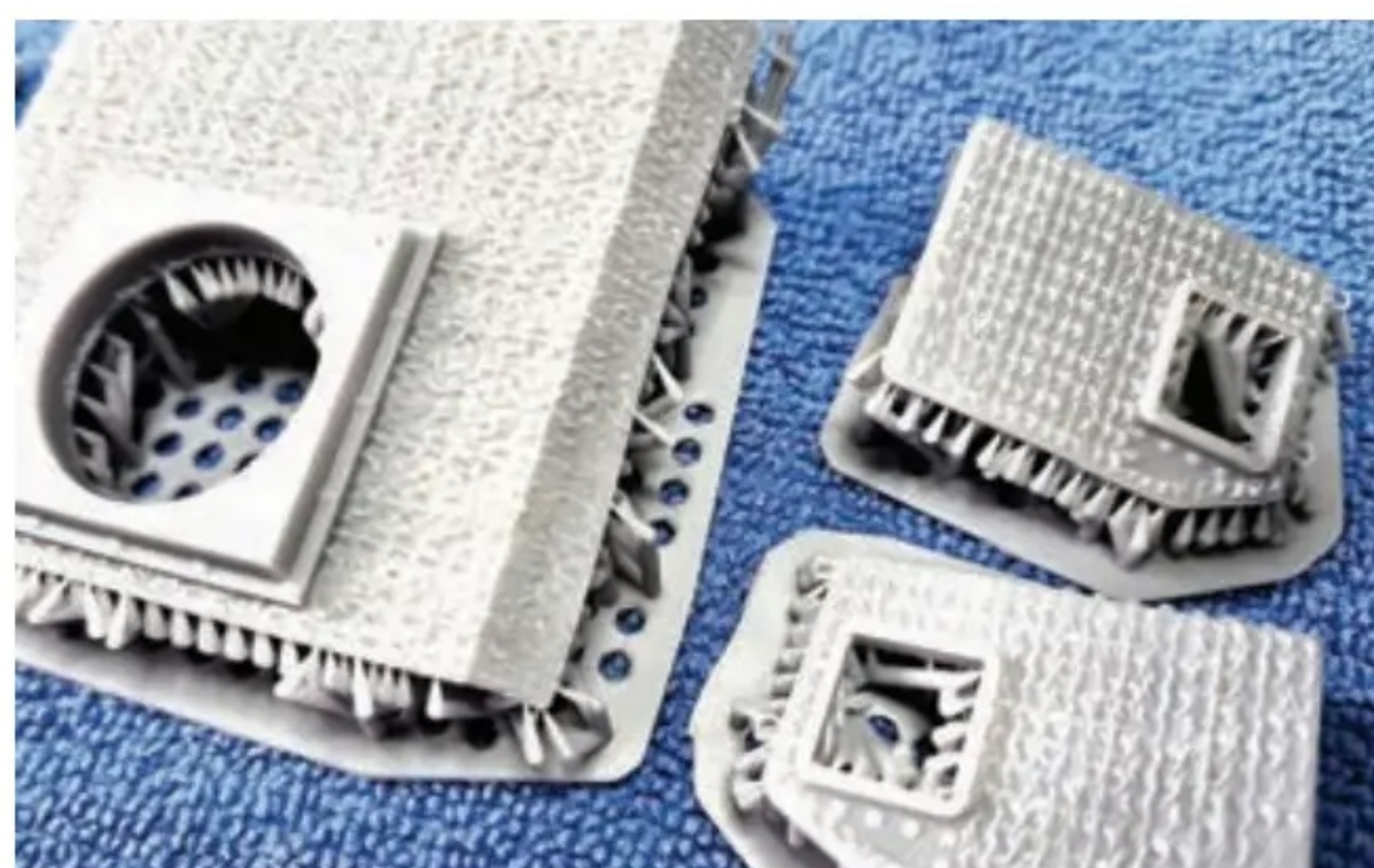
3D Printed cab top and doors
