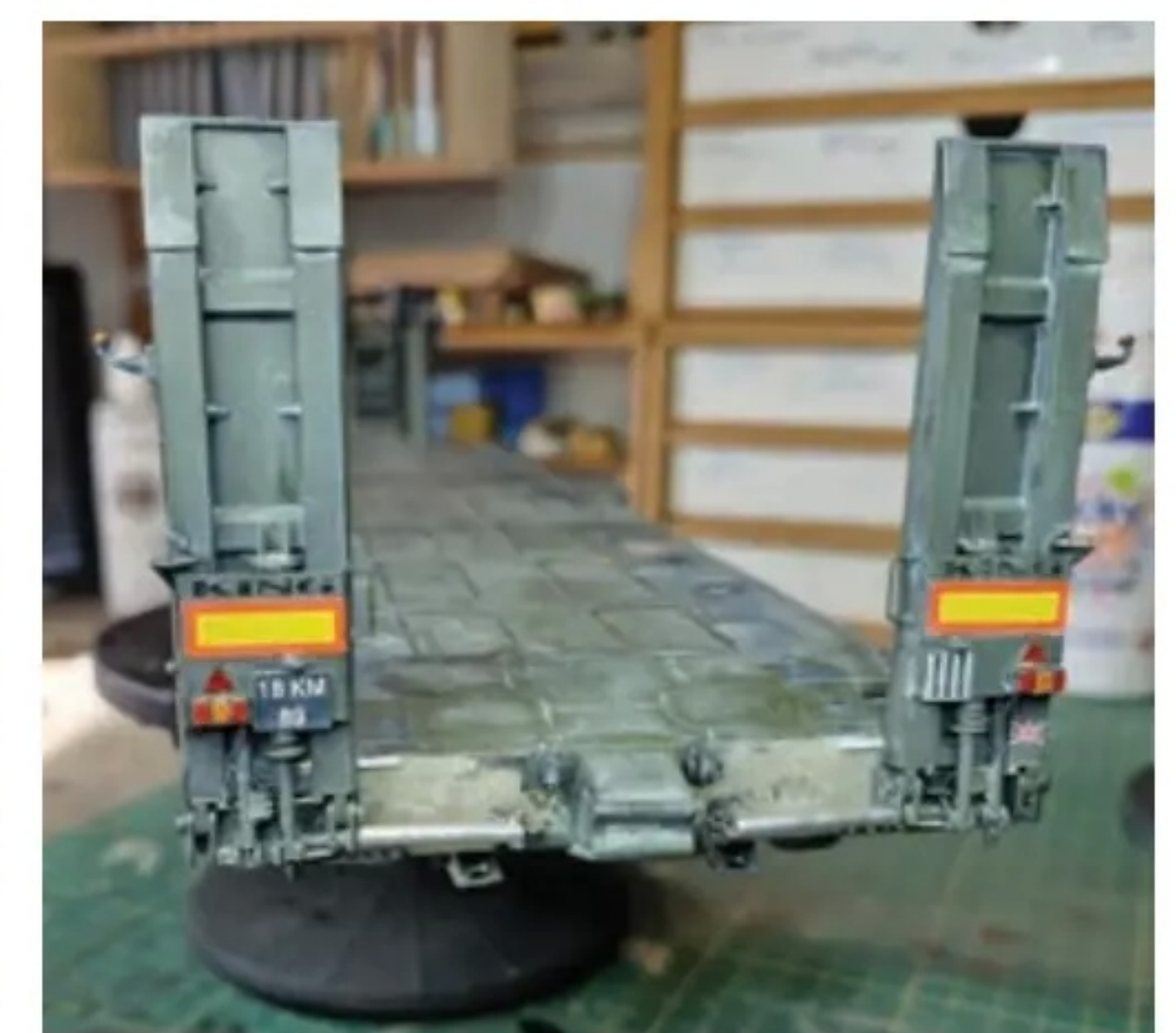
After test fitting I discovered that the ramps needed to be placed in their wide positions
