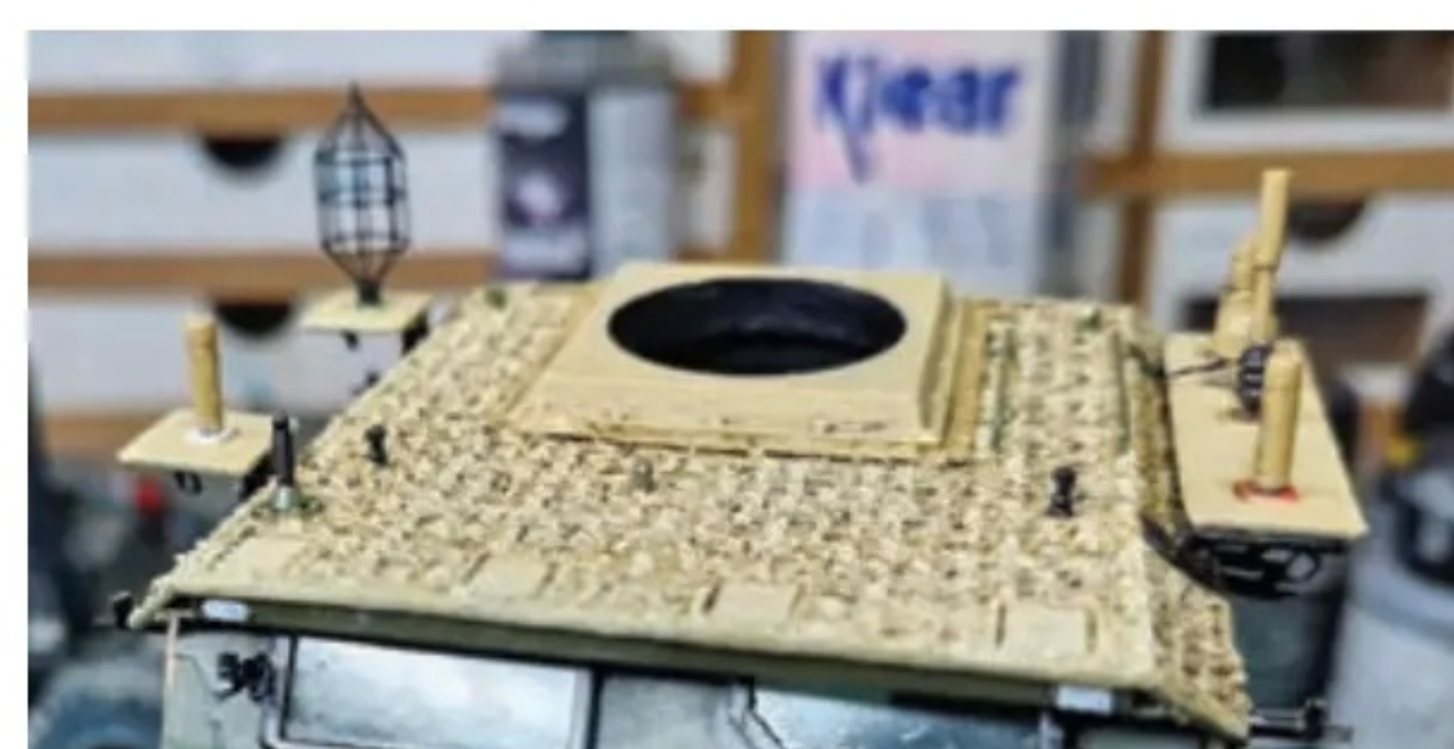
Bulkhead detail. Note the coloured hoses. Cab top detail. Note the different ECM antennas and fixture for mounting the turret.
