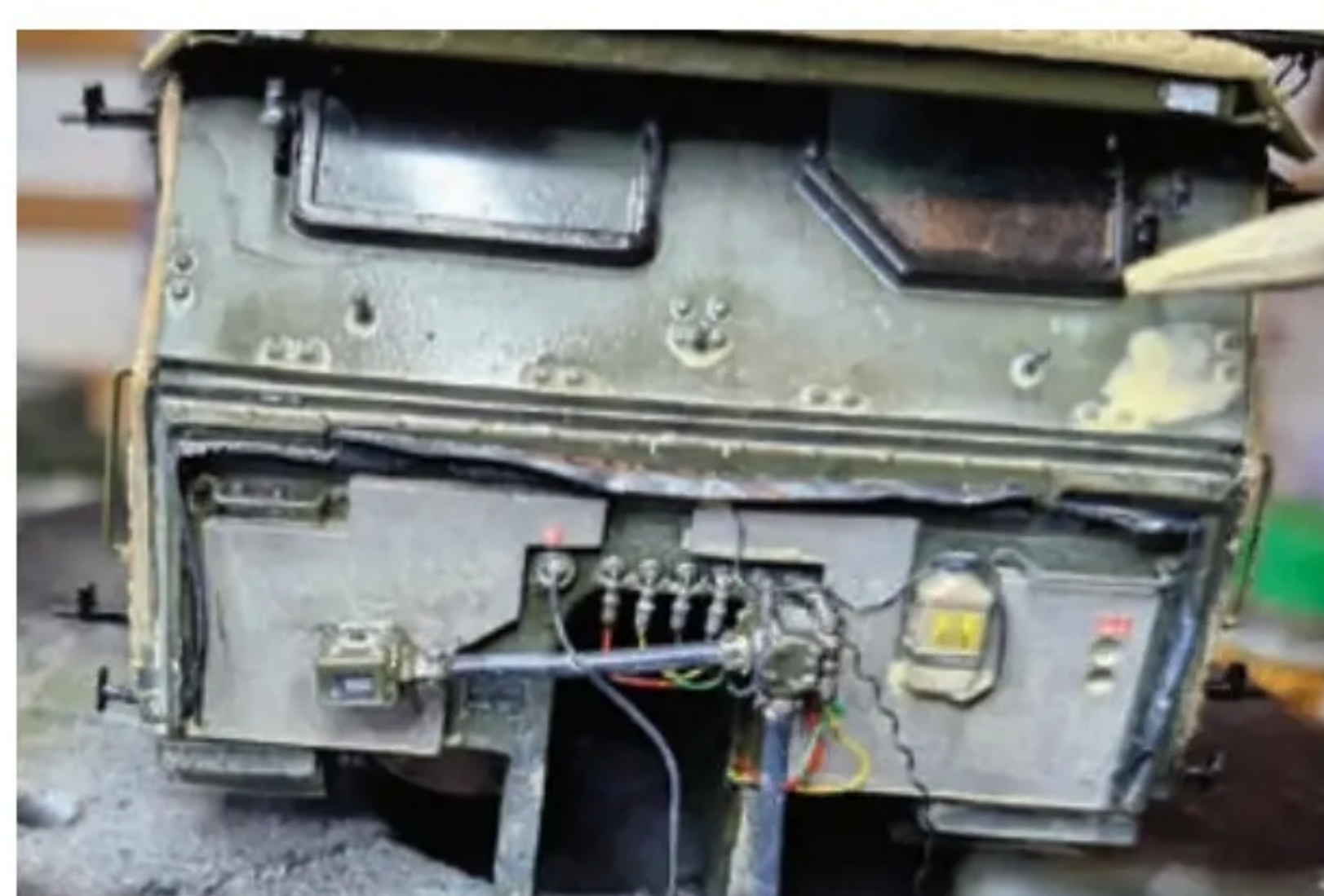
The detail achievable with 3D printing is amazing, but here you can also see the layers from the printing. This can be tidied with light sanding.
