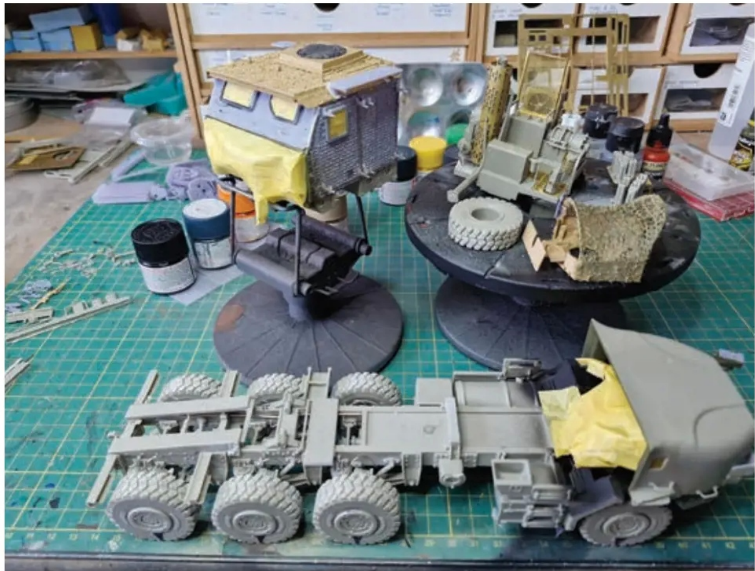
Rebuilding the front ECM brackets from plastic stock as the 3D printed items were too small.
