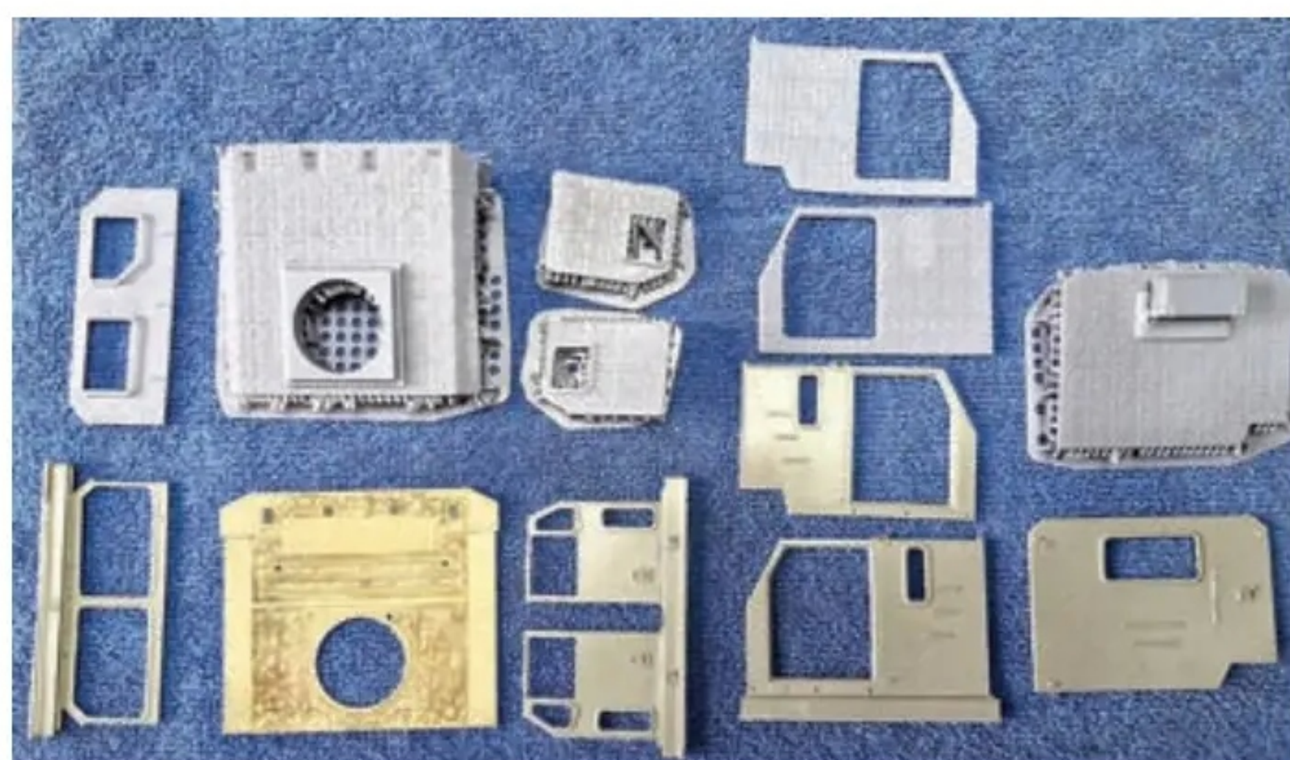
Kit parts were used as reference to redesign the uparmoured parts
