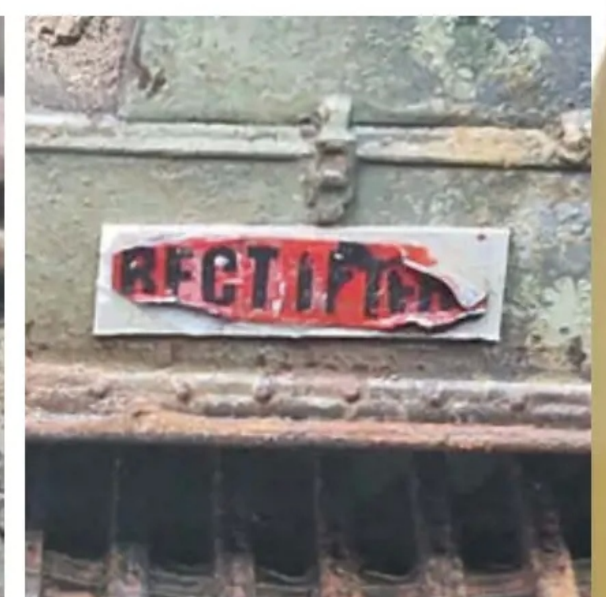
RECTIFIER name plate, made up with lead foil and leftover decals.
