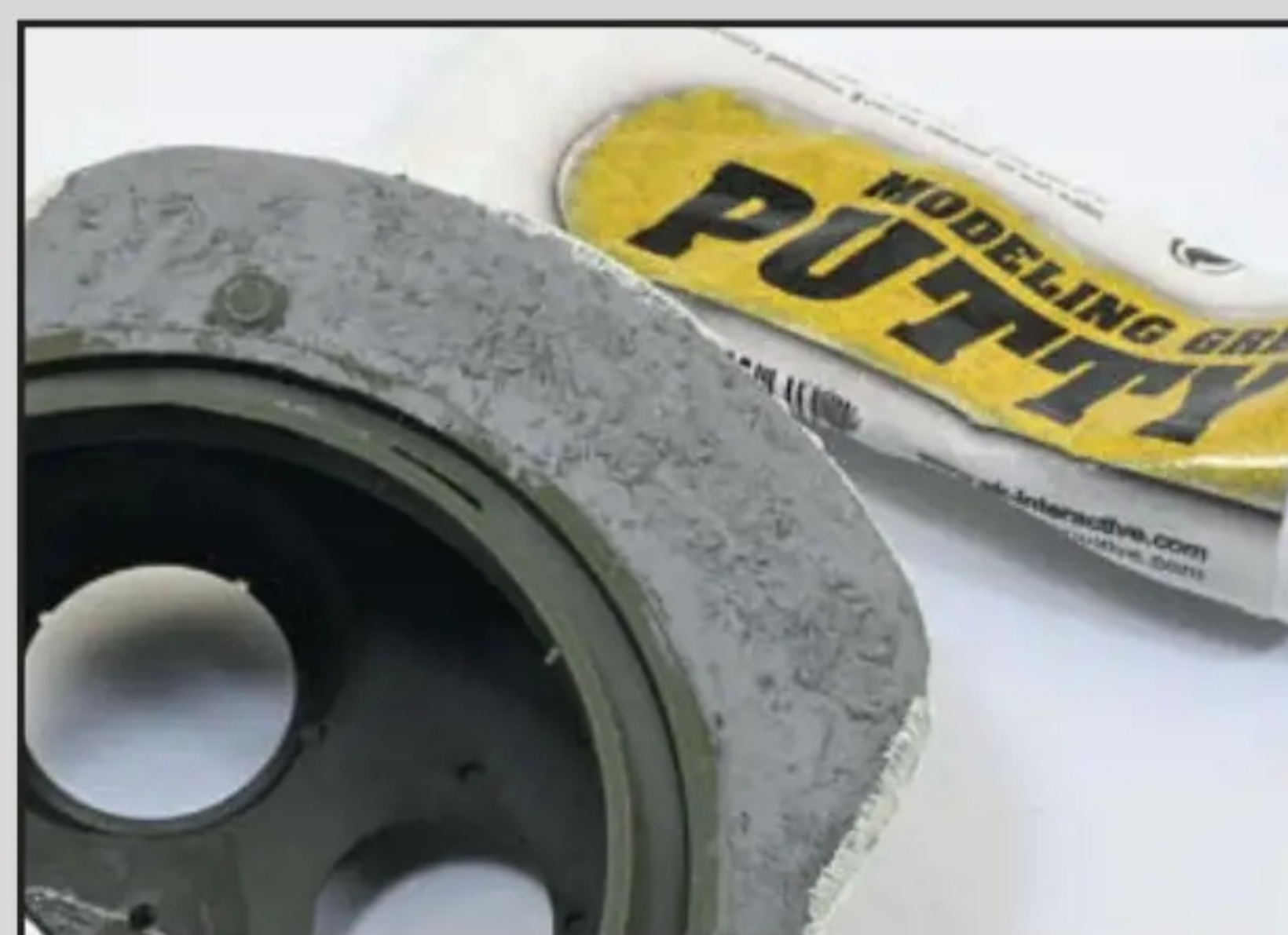
I applied modelling gray putty to the entire previously prepared surface, trying to do it in a random way but controlling the entire process.
