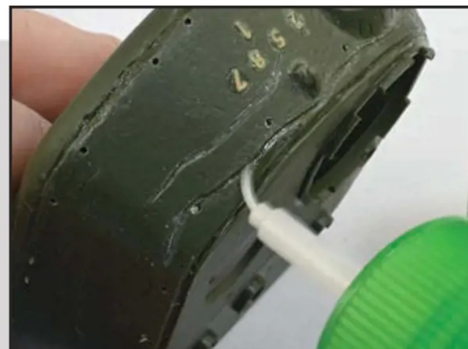
All the grooves were rubbed with thin glue to get rid of plastic particles created during work and to soften the edges of the cuts.
