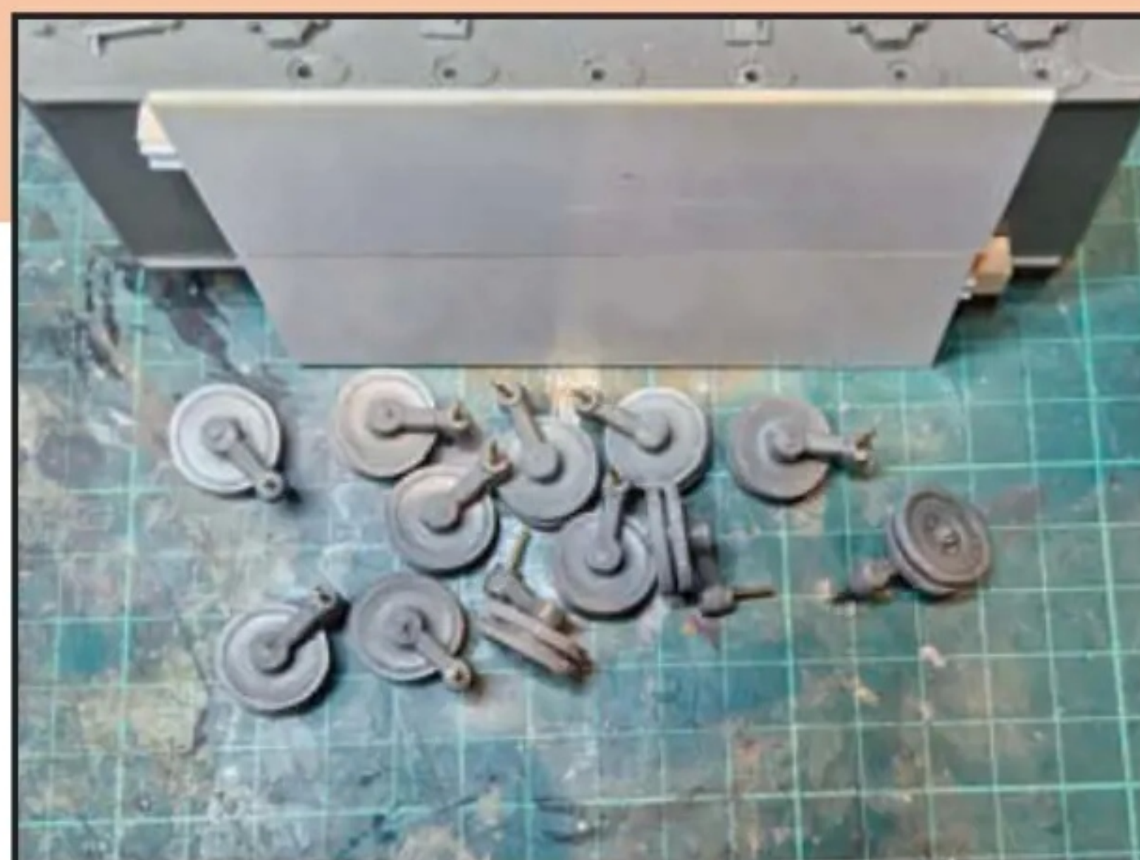
Roadwheel arms with brass rods added for strength. Also note the jig added to the hull bottom to ensure the correct ride height
