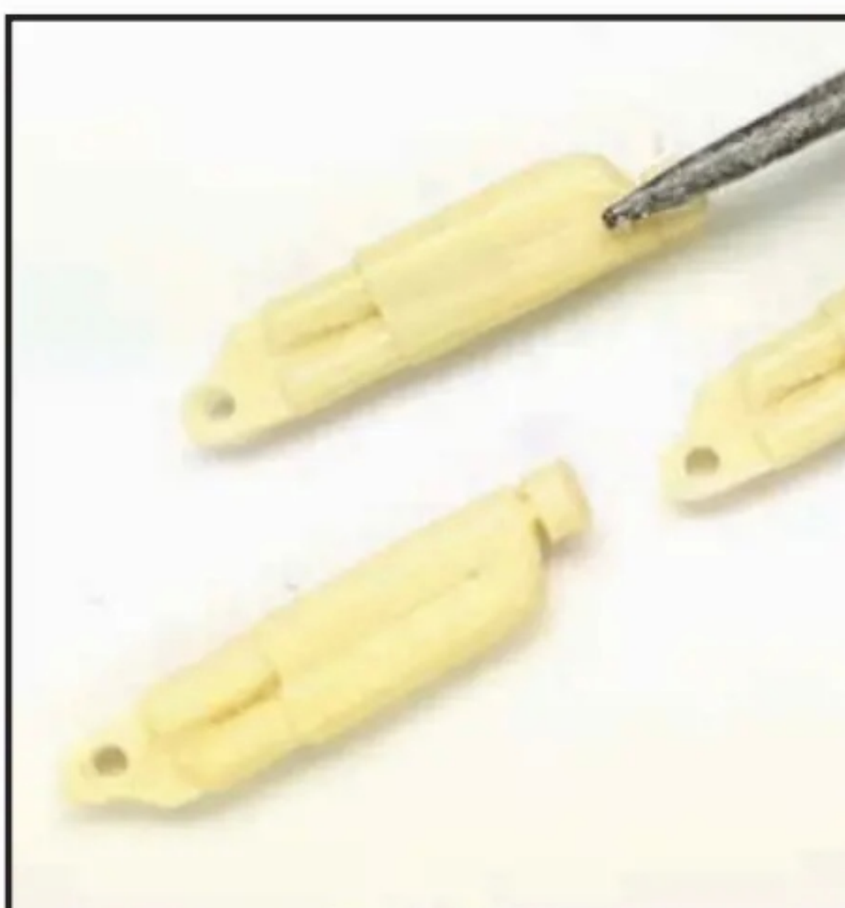
Flat shoulders of the shock absorbers were shaped to replicate my reference images
