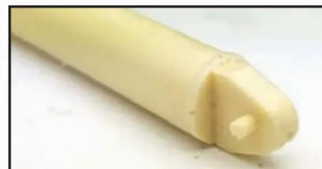
In the box I found a fundamentally shorter tube intended for a barrel so had to make a new one. Undoubtedly the producer's biggest mistake but fortunately I found a quick solution. I bought quite cheap electrician's plastic pipe of 16mm diameter and a proper thickness of the barrel I depicted with a short piece of inserted steel pipe. Inner of the steel pipe was turned out to 11.6mm which corresponds with the calibre 406mm in 1:35 scale. The same steel pipe section with a wooden dowel (like a mandrel) I used to fix the barrel into the resin breech block.
