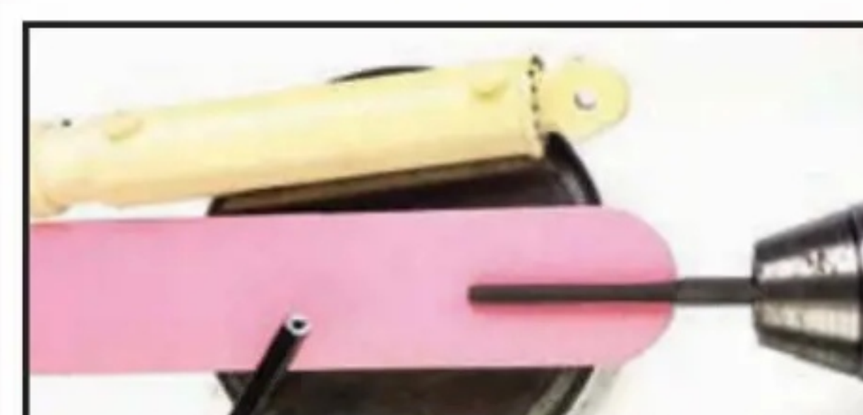
Equilibrators adjustment required a new hollow pin connector, a missing groove and adding the missing screw heads. Hollow connectors and the groove I did by means of a hand drilling machine.
