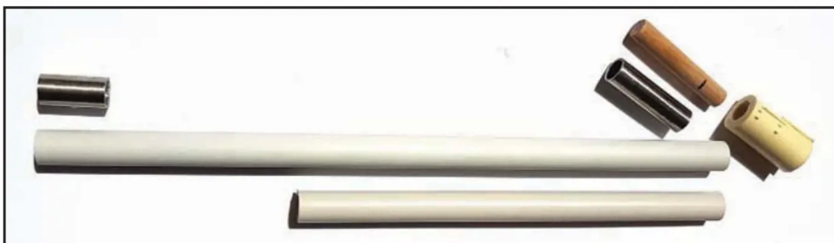
In the box I found a fundamentally shorter tube intended for a barrel so had to make a new one. Undoubtedly the producer's biggest mistake but fortunately I found a quick solution. I bought quite cheap electrician's plastic pipe of 16mm diameter and a proper thickness of the barrel I depicted with a short piece of inserted steel pipe. Inner of the steel pipe was turned out to 11.6mm which corresponds with the calibre 406mm in 1:35 scale. The same steel pipe section with a wooden dowel (like a mandrel) I used to fix the barrel into the resin breech block.
