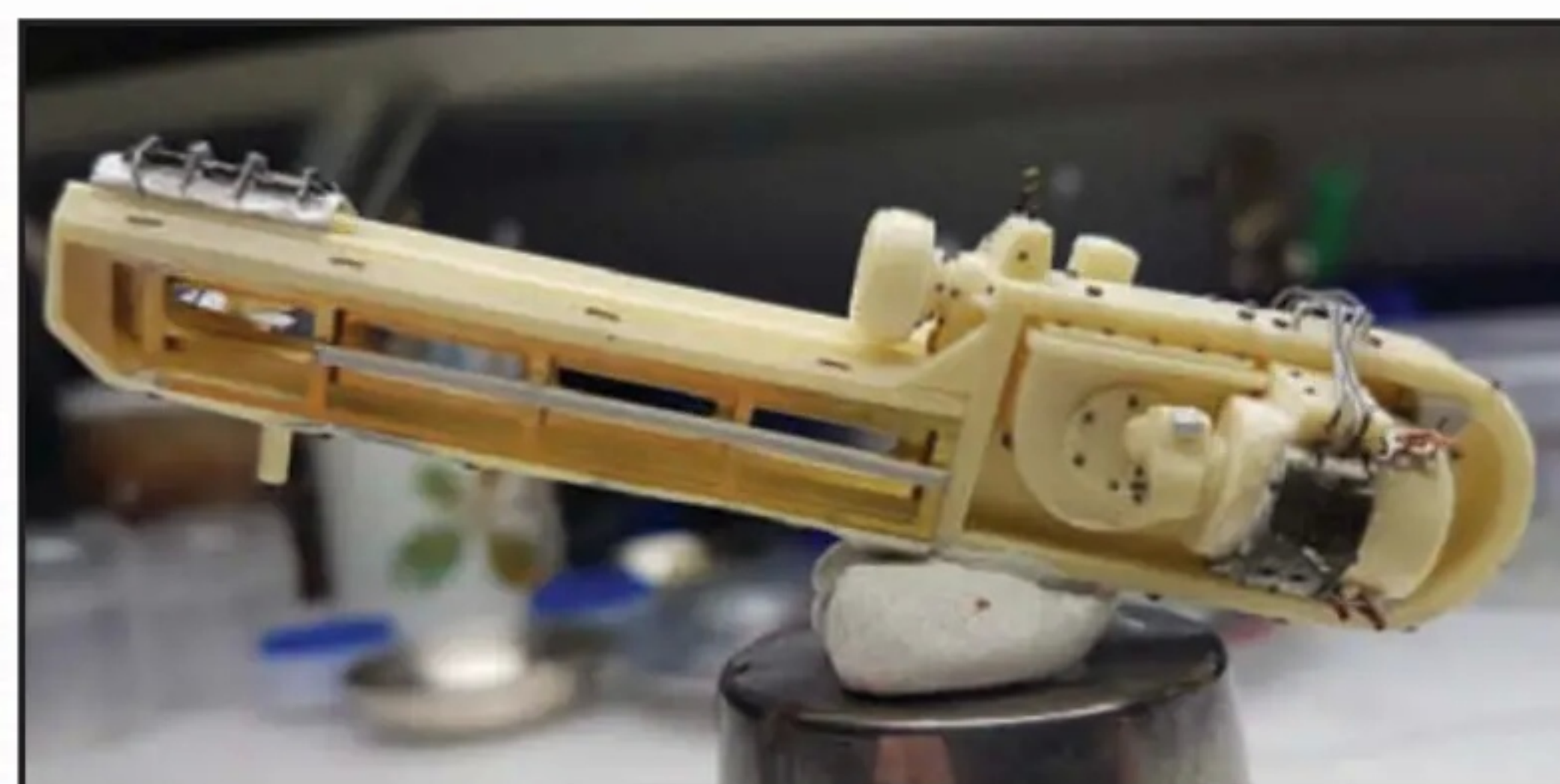
Equilibrators adjustment required a new hollow pin connector, a missing groove and adding the missing screw heads. Hollow connectors and the groove I did by means of a hand drilling machine.
