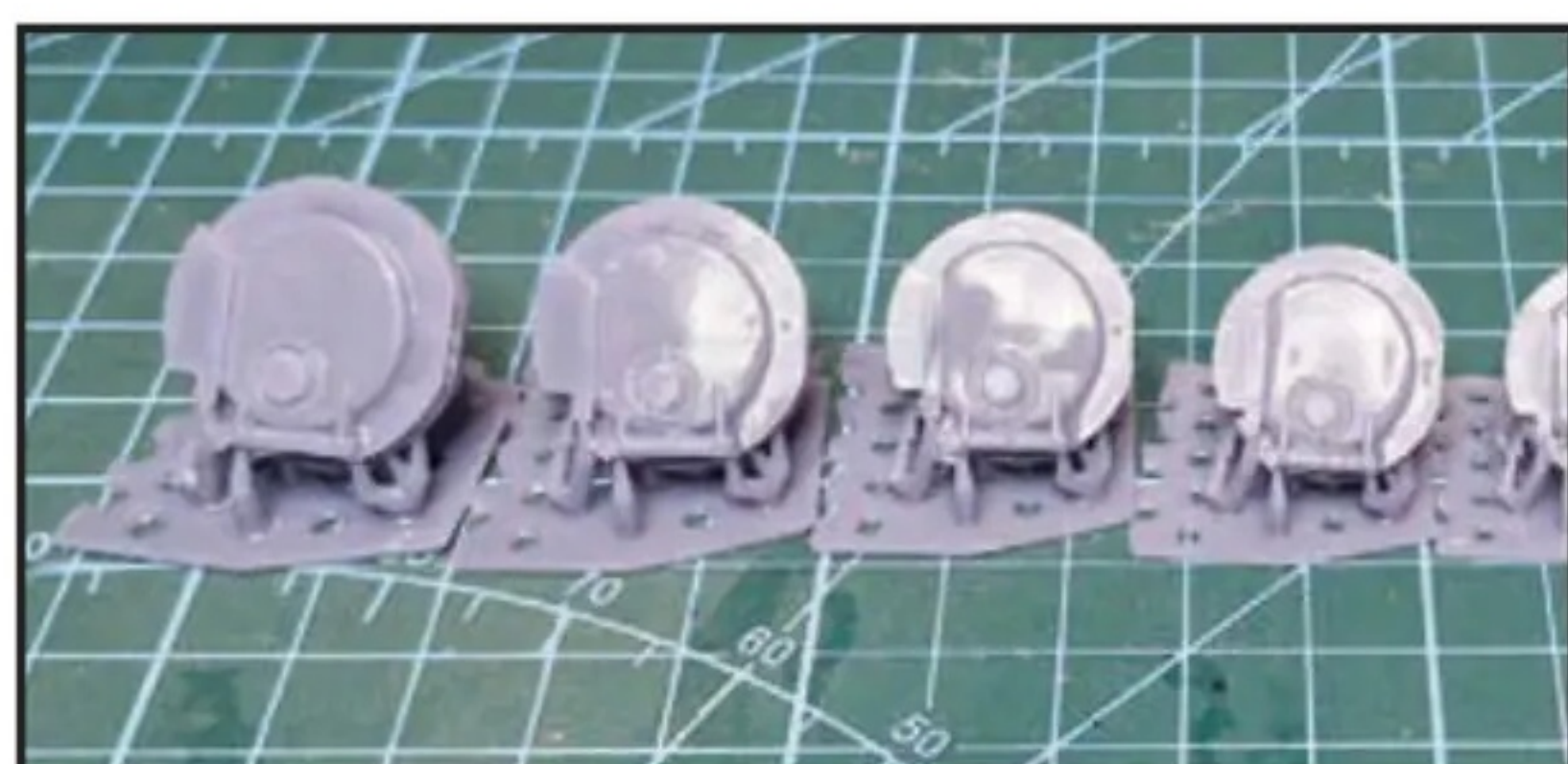
My model was missing the commanders cupola. I used a free 3D print file to print off various sizes to ensure the correct fit
