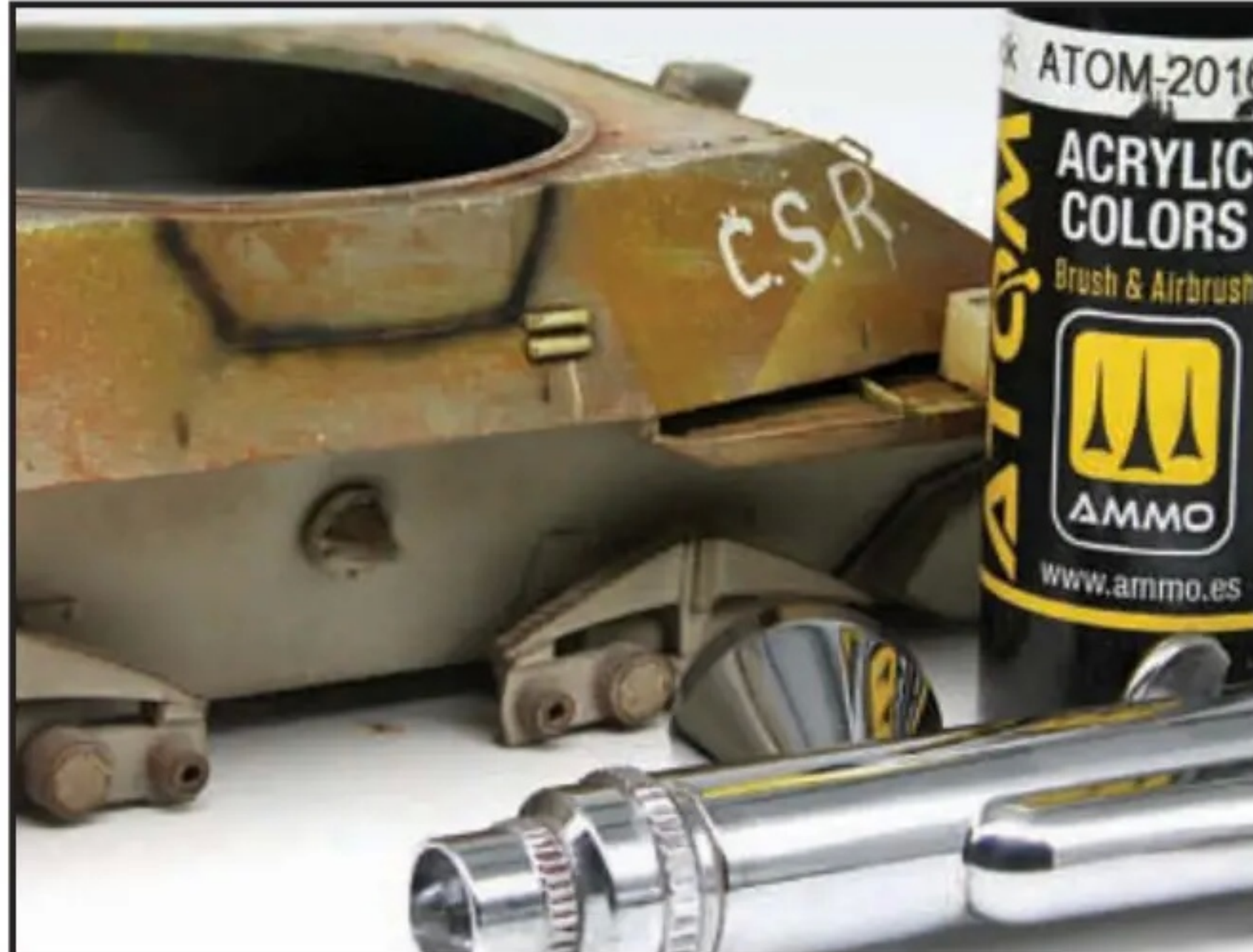
Weld beads around the bulges on the sides were first airbrushed with matt black
