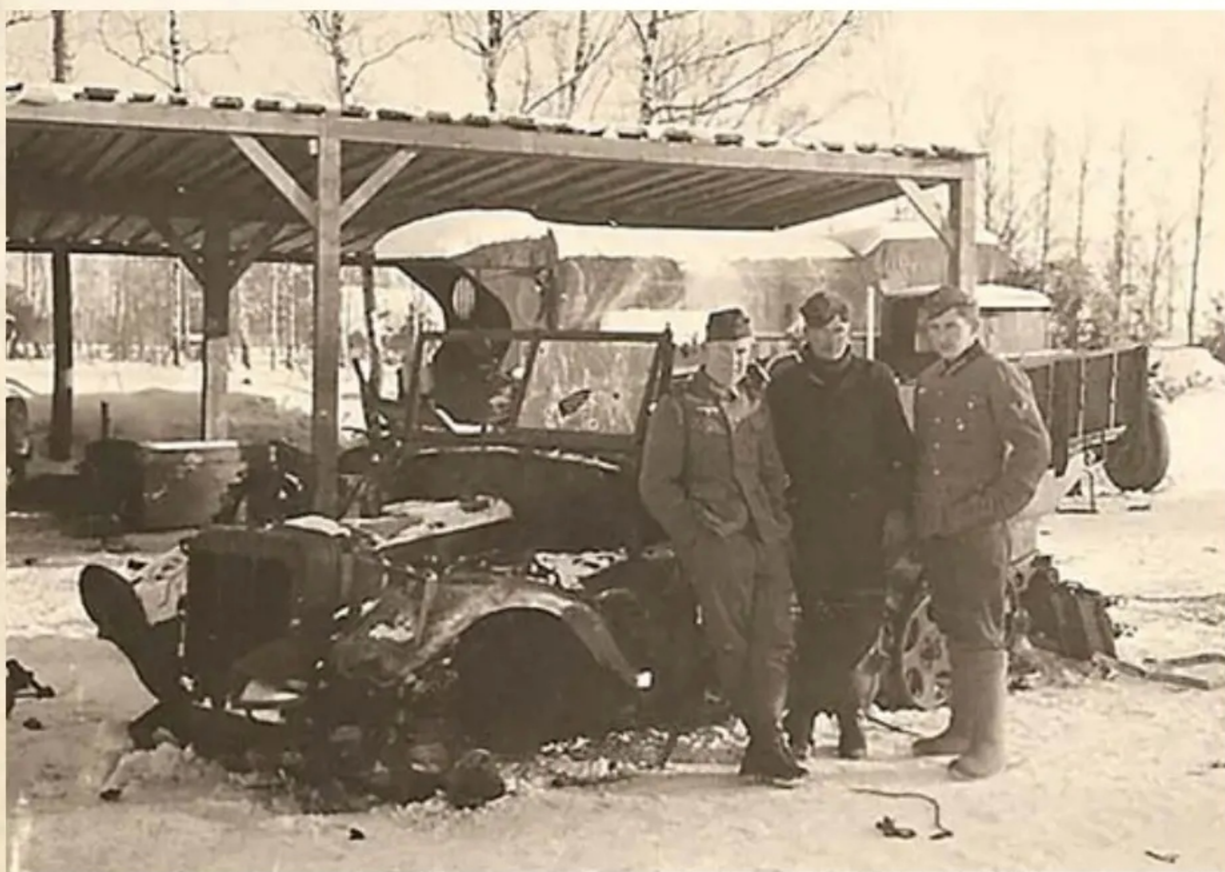
Here we see a badly damaged Sd.Kfz 10/4 or 10/5; I can't tell which as the gun has been removed already is seen back at the home barracks of Luftwaffe Flak regiment 6 in Hamburg. The vehicle that had been assessed a repairable but beyond the capabilities of the unit's field based maintenance troop has been returned to Hamburg for full repairs. Its gun removed and no doubt being part of the channel defences as the photo was taken on November 1st 1940.
