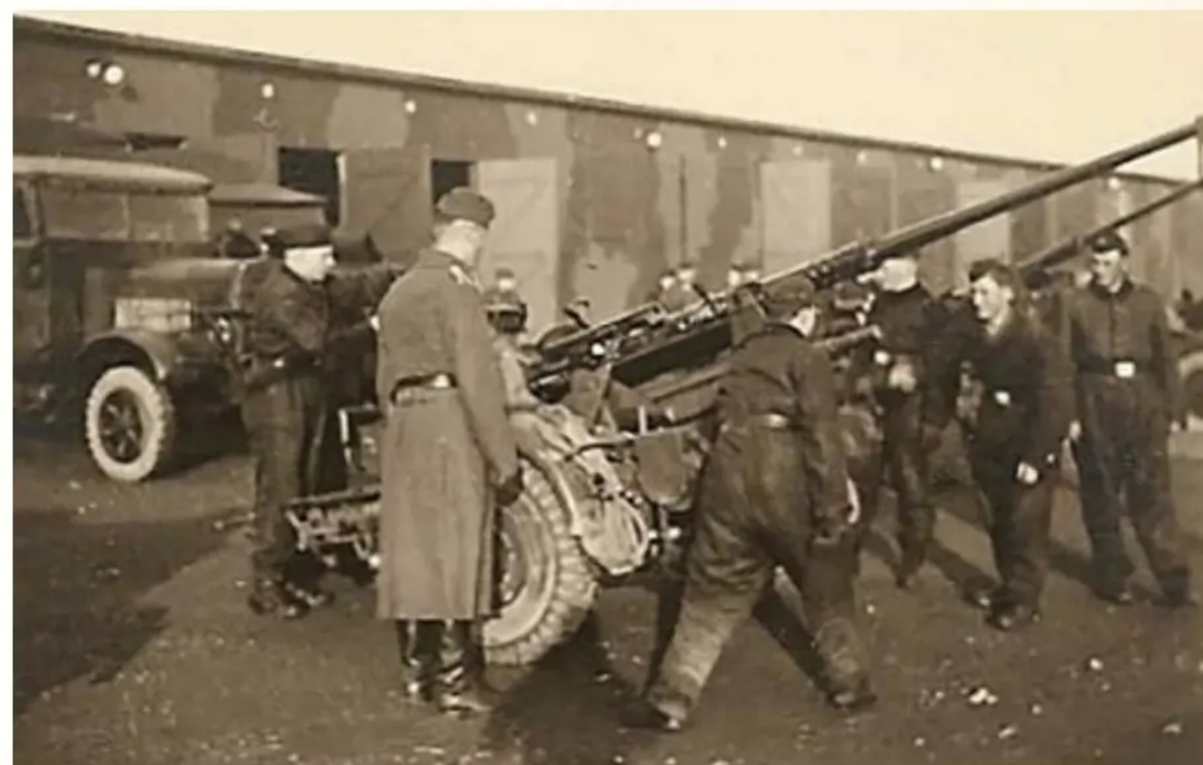
Taken in the Panzer hall yard (Garage area) of Luftwaffe Flak regiment 6 Hamburg barrack's in the summer of 1940, this photograph shows gun crew preparing for an imminent inspection. Note the 20mm Flak30 still attached to their transportation trailers (Sd.Anh 51's), the trucks in the background are Henschel D33's
