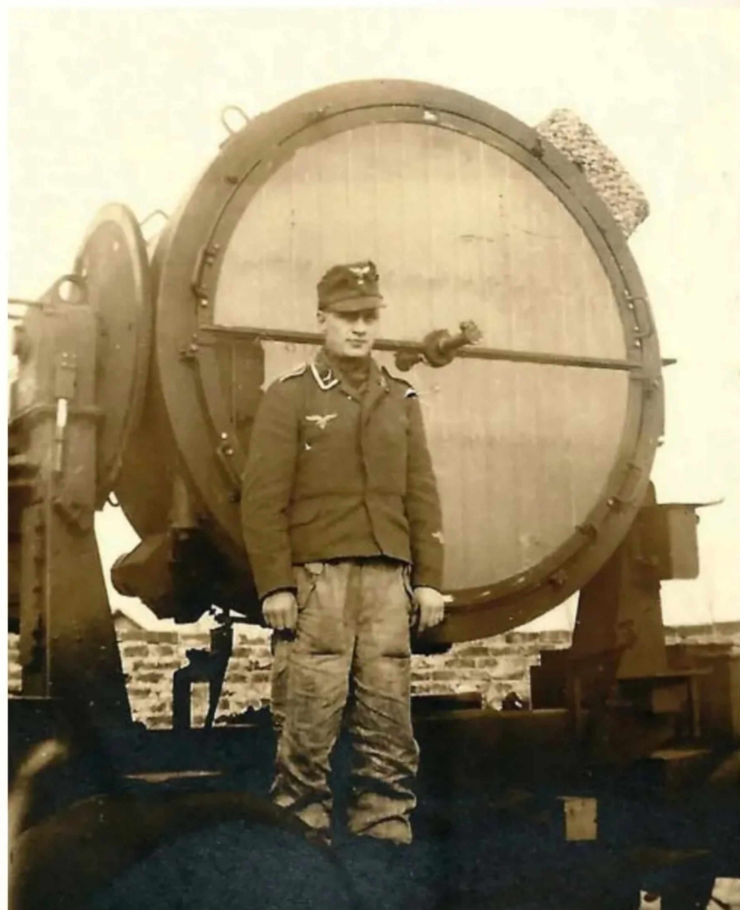
Here we have a 150 cm Sw. 34. In its early production format, it was mounted on a rectangular platform with four wheels and a levelling jack mounted on a steel tubular fold-down frame in each corner. This same four-wheeled base frame was used to mount some early Würzburg radars and even a few 20 Flak Vierling, as evidenced by photographs in my own collection. The photograph is of a searchlight in a brick culvert on the Rhine river bank in the Demag factory complex in Duisburg, Germany. This factory searchlight unit was manned by Luftwaffe auxiliaries who worked in the factory. The photo was taken in January 1944.
