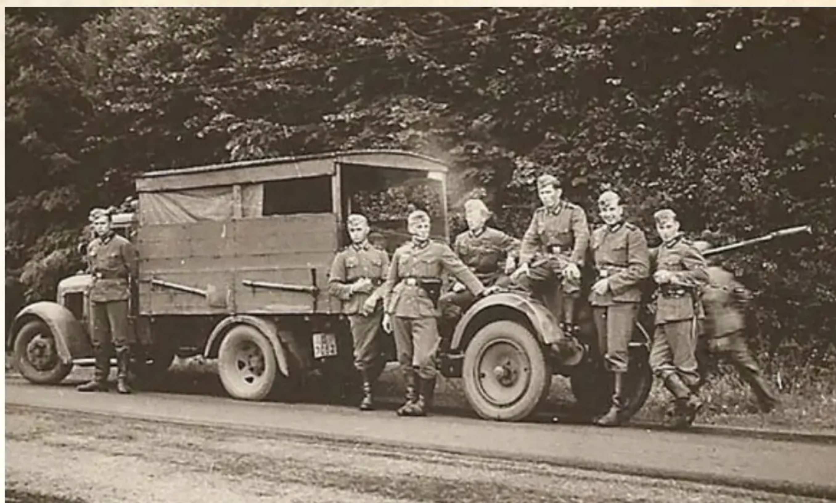
This gun and crew from Luftwaffe Flak regiment 6. Are seen in transit from Belgium to their next assignment around the Pas de Calais area of Northern France, on June 28th 1940. The truck is a 1934 pattern 2.5 ton Mercedes and the gun it is towing is a 20mm Flak 30.
