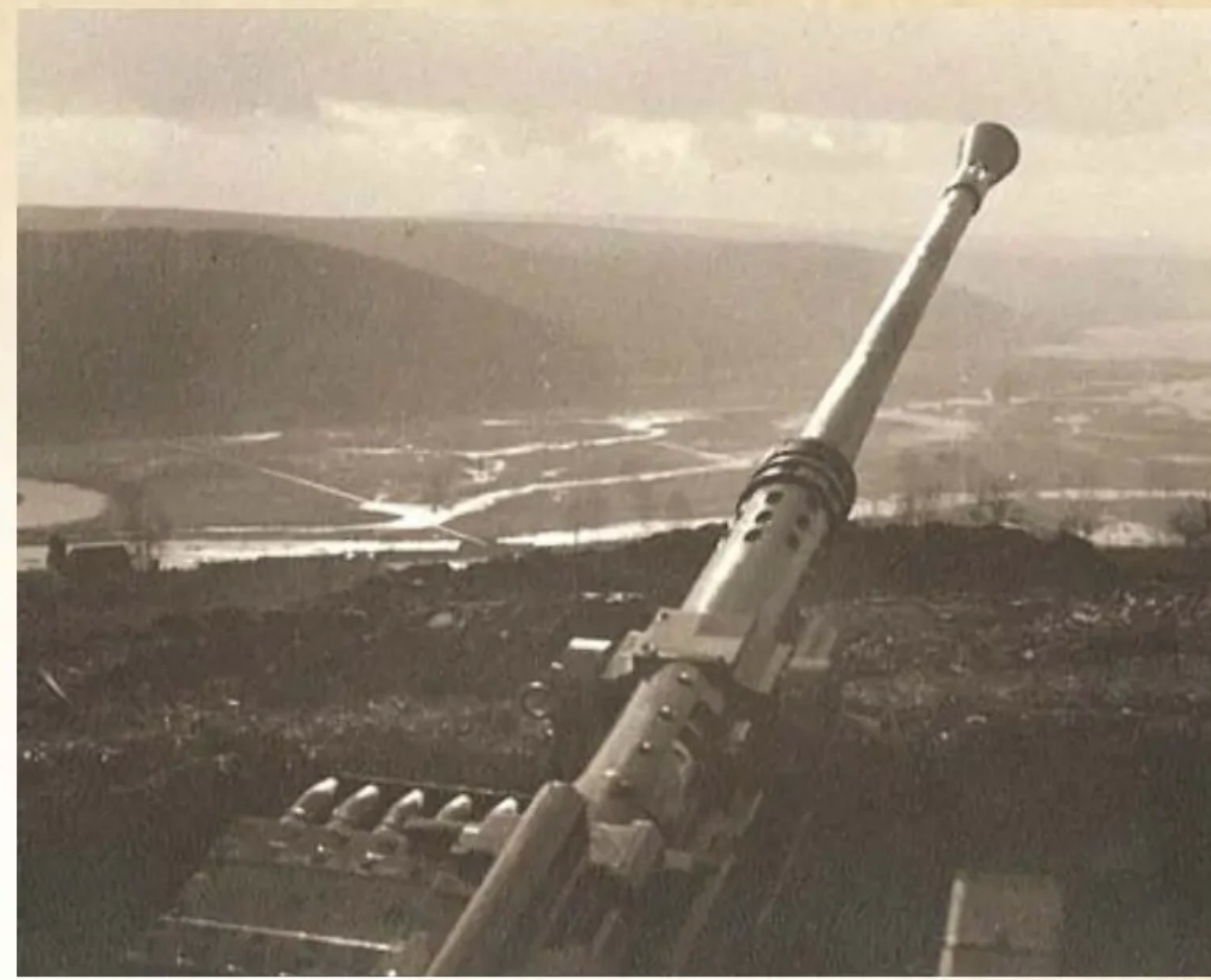
This photo, taken somewhere on the coast of Denmark, gives us a good look at the top of the 37mm Flak 36. We can see the top of the gun sight at the right bottom of the photo, then the cocking spring housing on top of the gun's breech and lastly the ammunition feed tray, here loaded with a full clip of six HE Flak rounds. Note the sixth round is already loaded in the weapon's breech.
