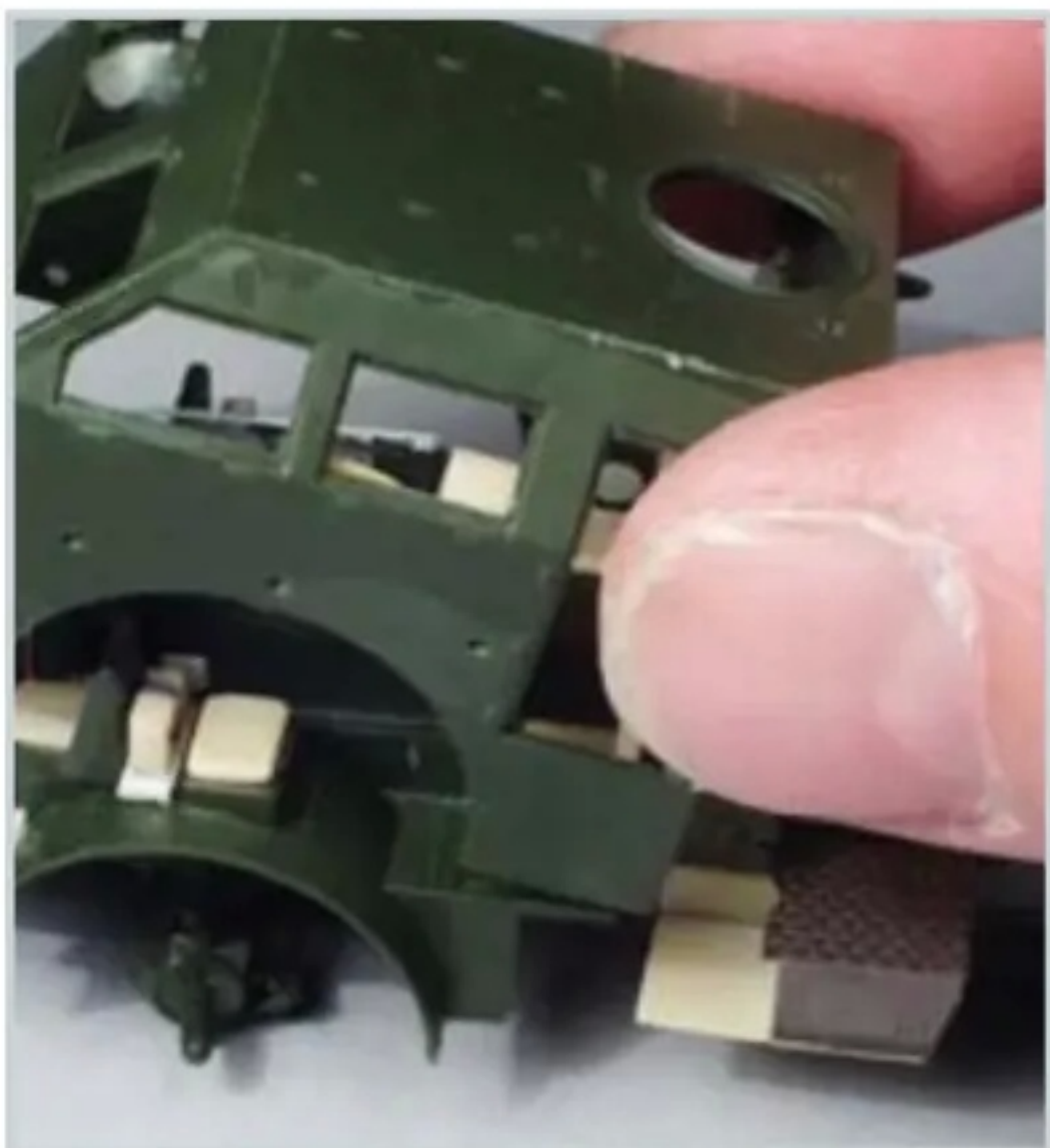
The armored cabin of the Dragon Wagon is particular: sharp and angled, it gives the vehicle an unmistakable look. I think that Academy has rendered this part at its best: even if a little thick, it has the stops of the various armored doors of the windows that are completely absent in the Planet Models kit, a rather serious error in my opinion.
