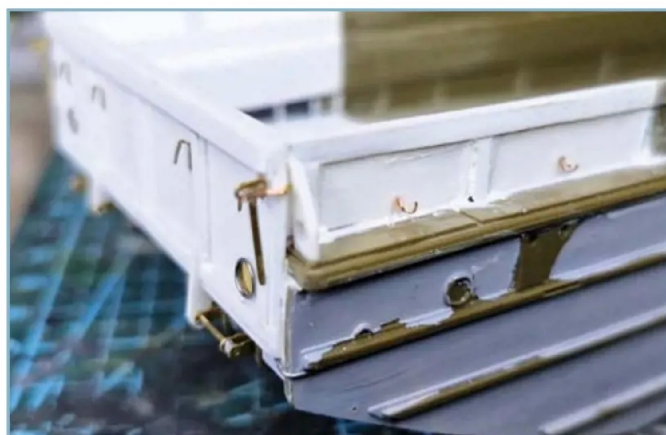
Details added to the ramp such as handles and tie downs.
