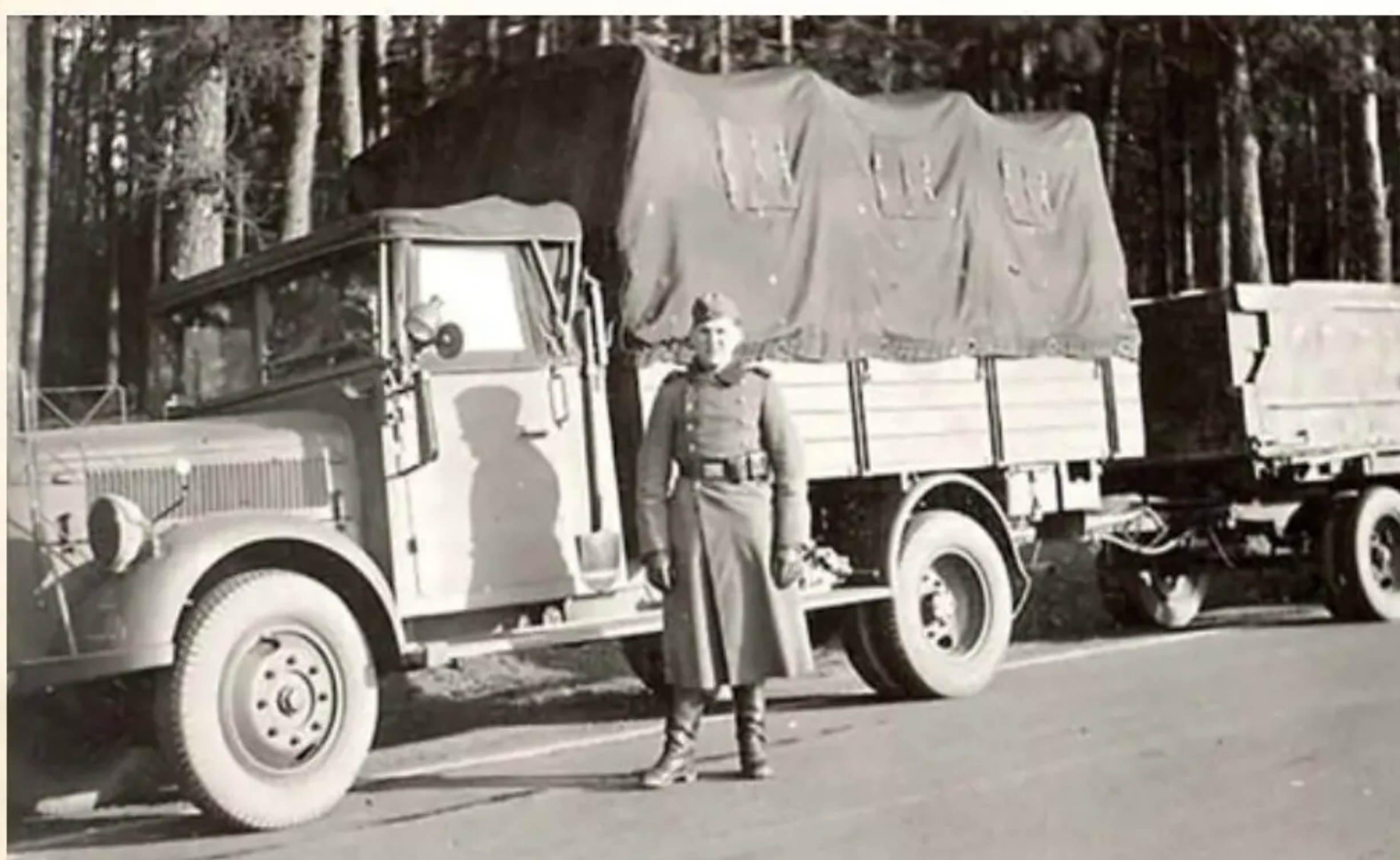
A Borgward 3 ton truck belonging to a German pioneer/engineering unit was photographed somewhere in Latvia in the late summer of 1941 during operation Barbarossa, it is seen to be towing part of a field engineering pontoon bridge section on its bespoke trailer.
