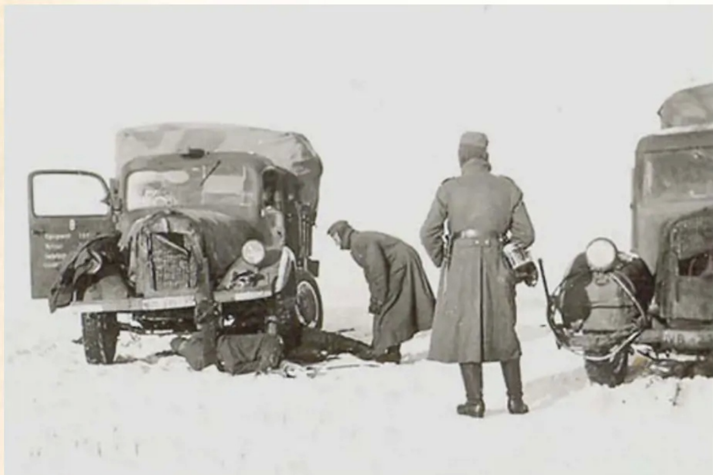
Here we have on the lefthand side of the photograph seen with a crew member lying under the front assessing the damage to the front steering linkage that has become unattached is a Borgward 1.5ton truck whilst on the right is a Mercedes 3 ton L3000 truck, both photographed during the winter of 1941/42 somewhere on the Russian step.
