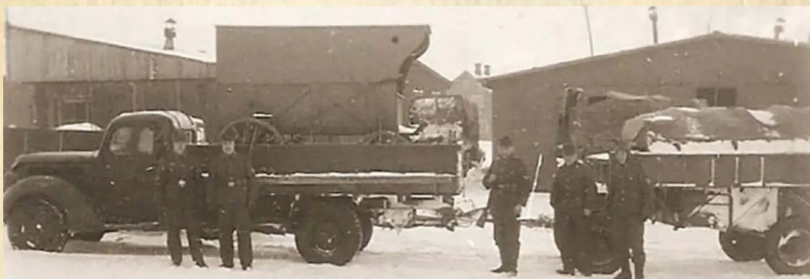
This 1938 Ford 3 ton truck with an extended rear load bed platform (a factory civilian option) & also towing a factory option 3 ton trailer as well was photographed in the winter of 1938/39 in the barracks complex located in Leipzig, Germany. Note the WW1 vintage ammunition wagon loaded on to the flat bed of the truck and many wooden ammunition boxes loaded on to the trailer.
