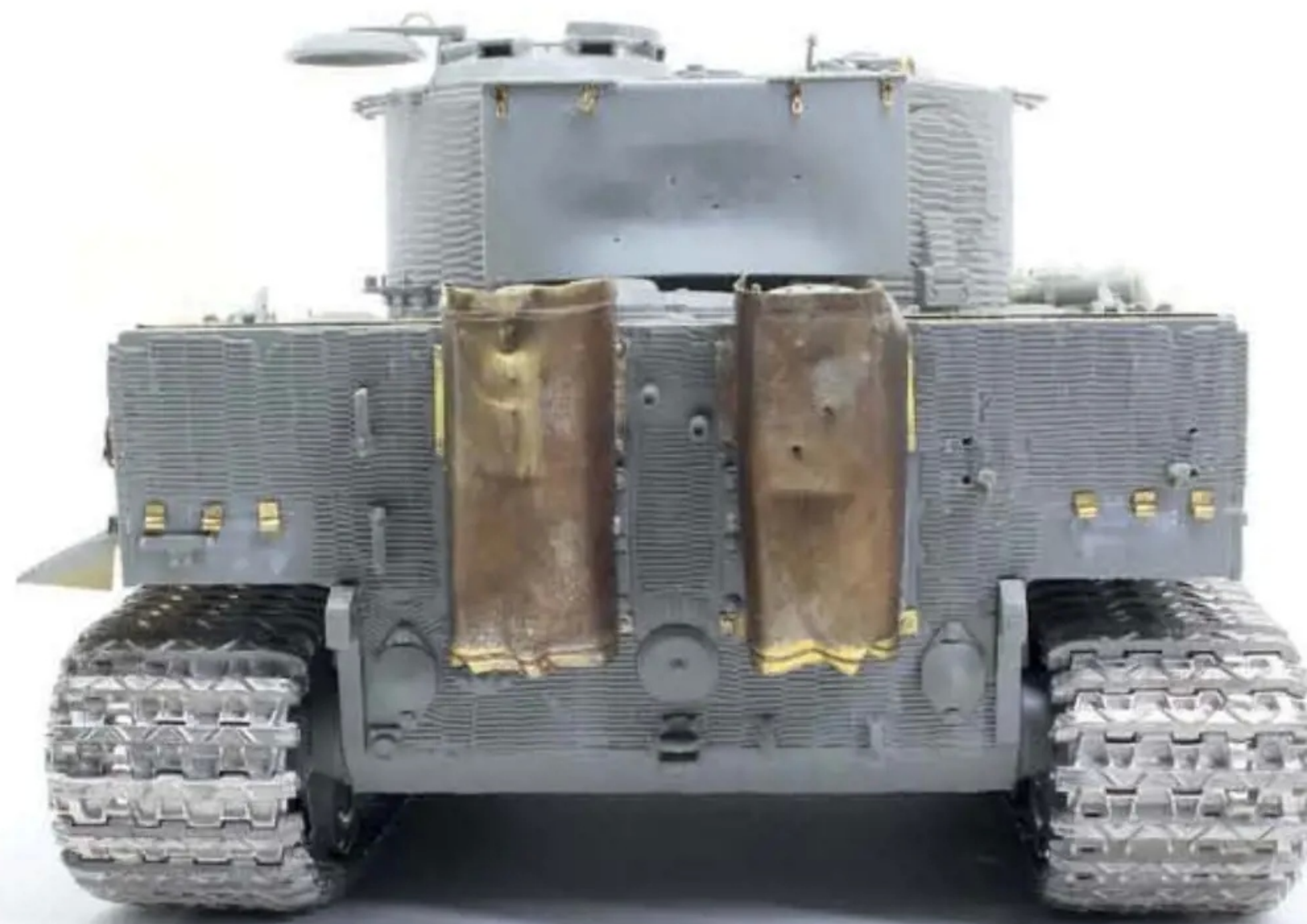
Note the damage to the stowage bin and exhaust shields.
