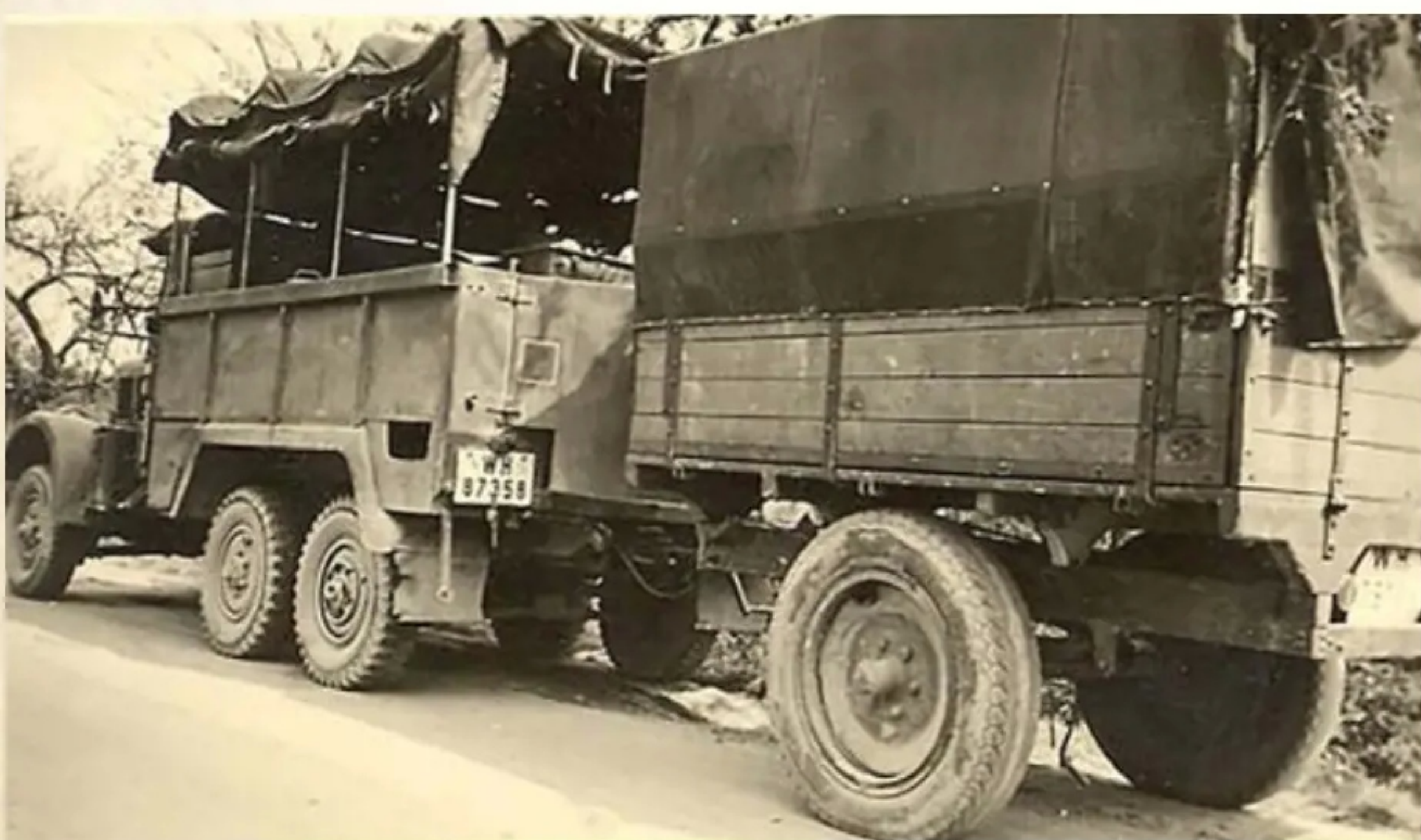
This Universal Diesel complete with its unit workshop built trailer made from a cut up wrecked French trucks rear load bed. The photograph was taken in the Aalst area of Belgium during March of 1941.
