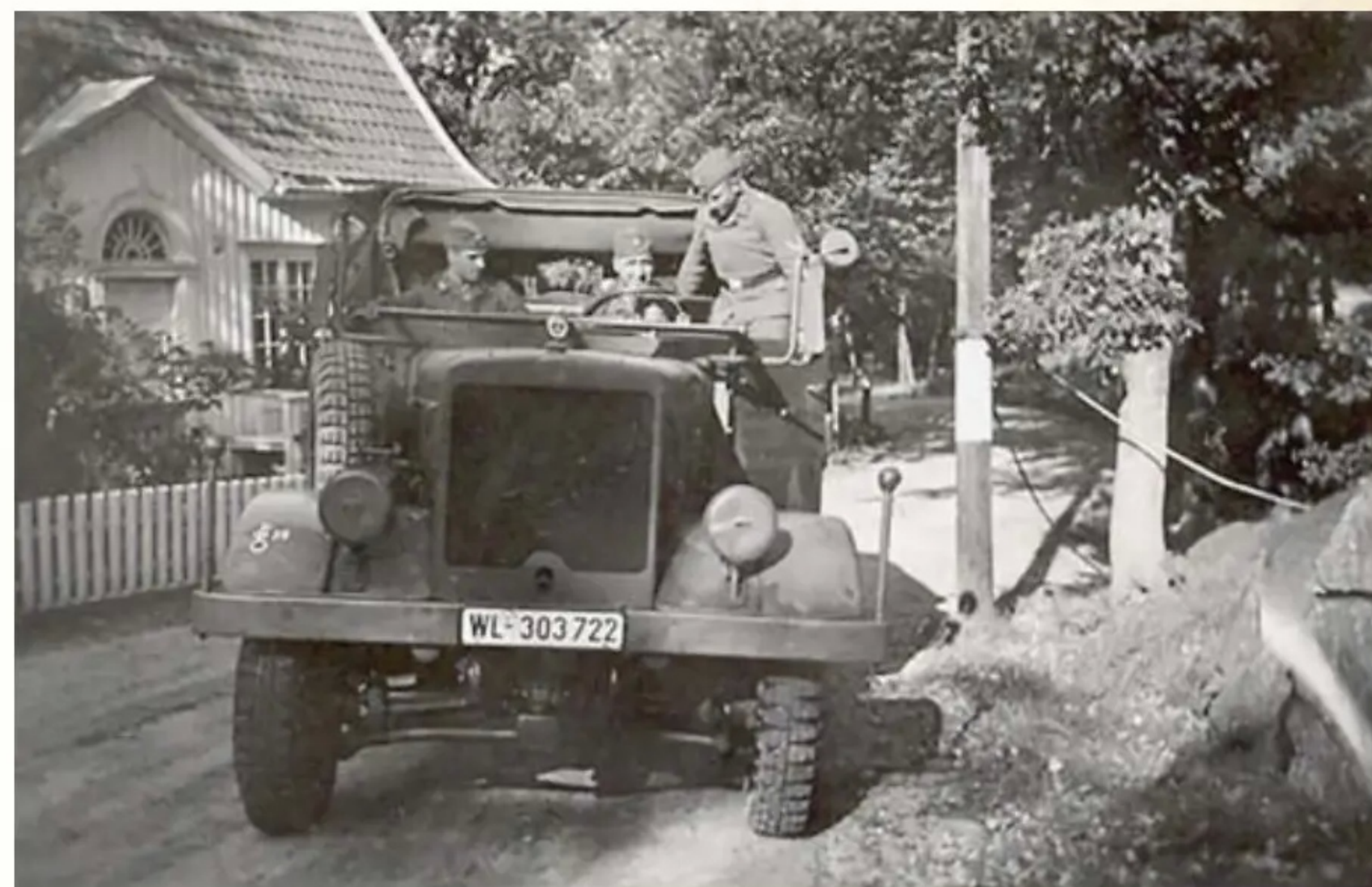
This high quality photograph shows a Luftwaffe mobile signal unit's Einheits-Diesel moving through a picturesque village somewhere in Luxemburg. Unusually, due to the clarity of this photograph on the original print, the manufacturer's logo can be identified – this truck was produced by Faun and is in as new condition.
