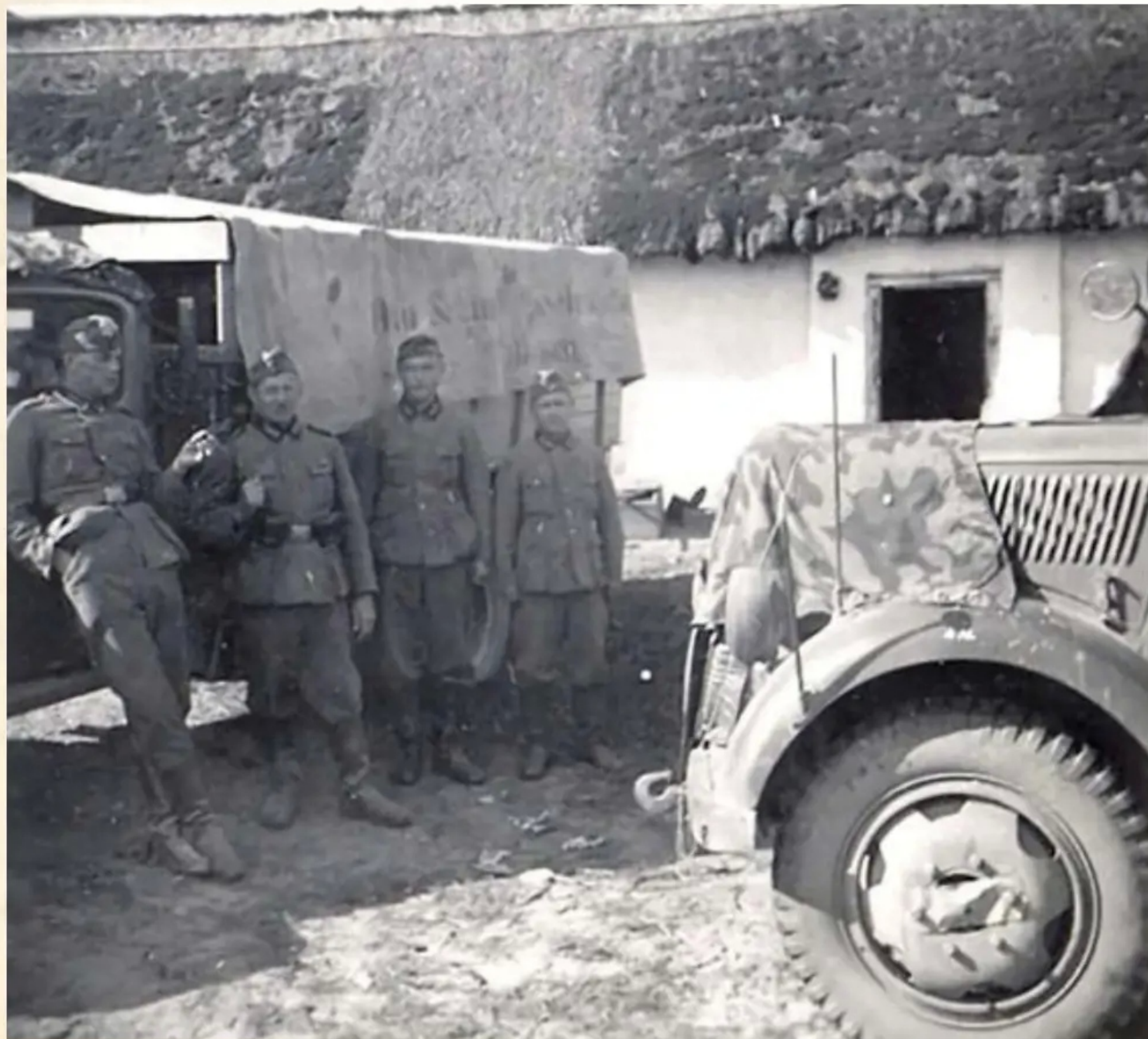
These two trucks are parked outside a Ukrainian farm house somewhere on the Crimean peninsula in July 1942. Note the truck with its front in the foreground is a 3 ton Opel Blitz Sd.Kfz 304, painted in overall Dark Yellow (Dunkel Gelb) with a camouflaged poncho draped over the radiator grill probably just to dry out as it does not appear to be attached to the truck in anyway.
