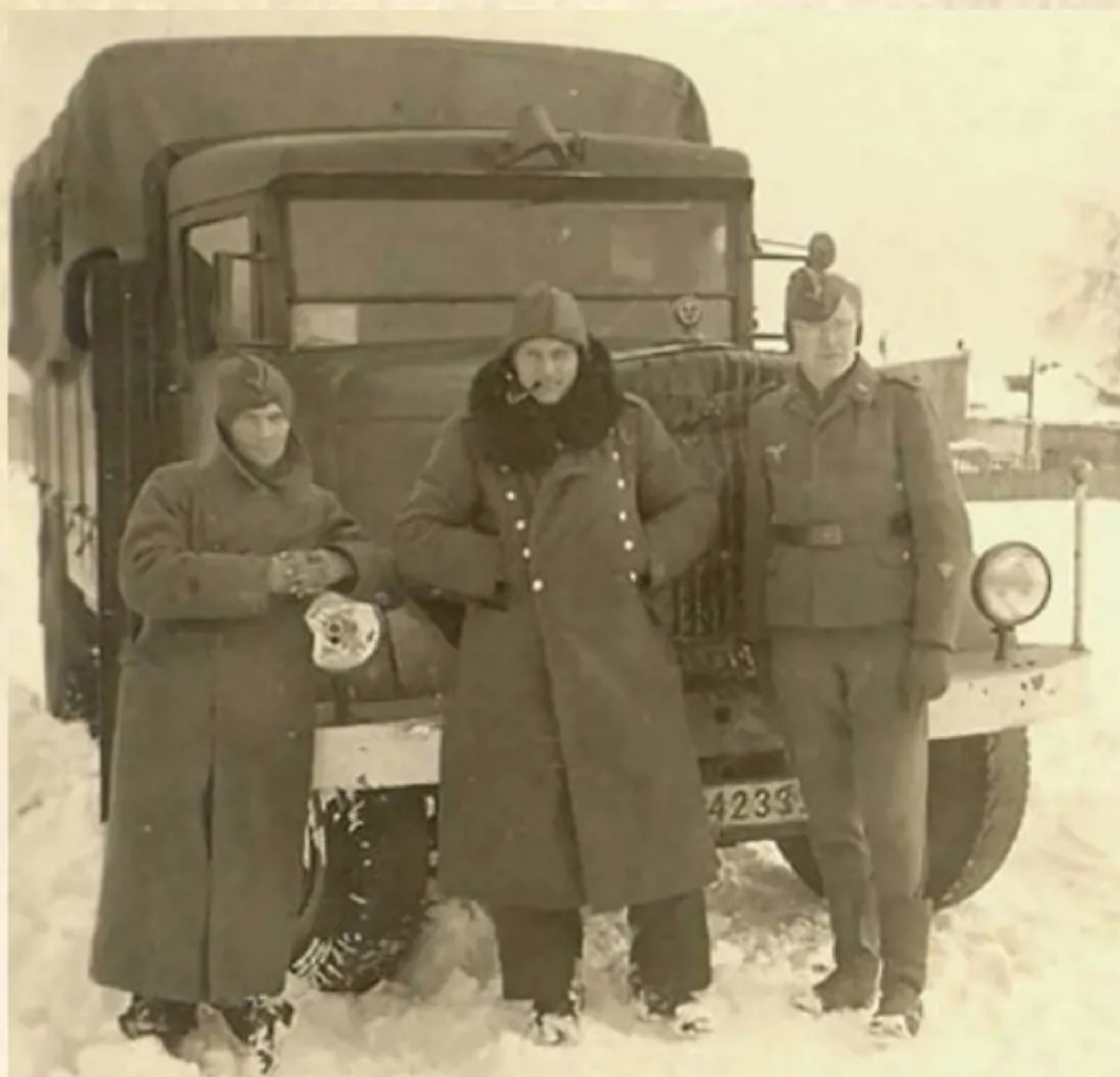
This pre-war ex civilian Man Type F-4 4 ton truck was pictured in Vilnius, Lithuania, on the 25th of December 1942. Of note is the unusual style of the towing indicator triangle on the roof of the cab and the uncovered headlights lenses.
