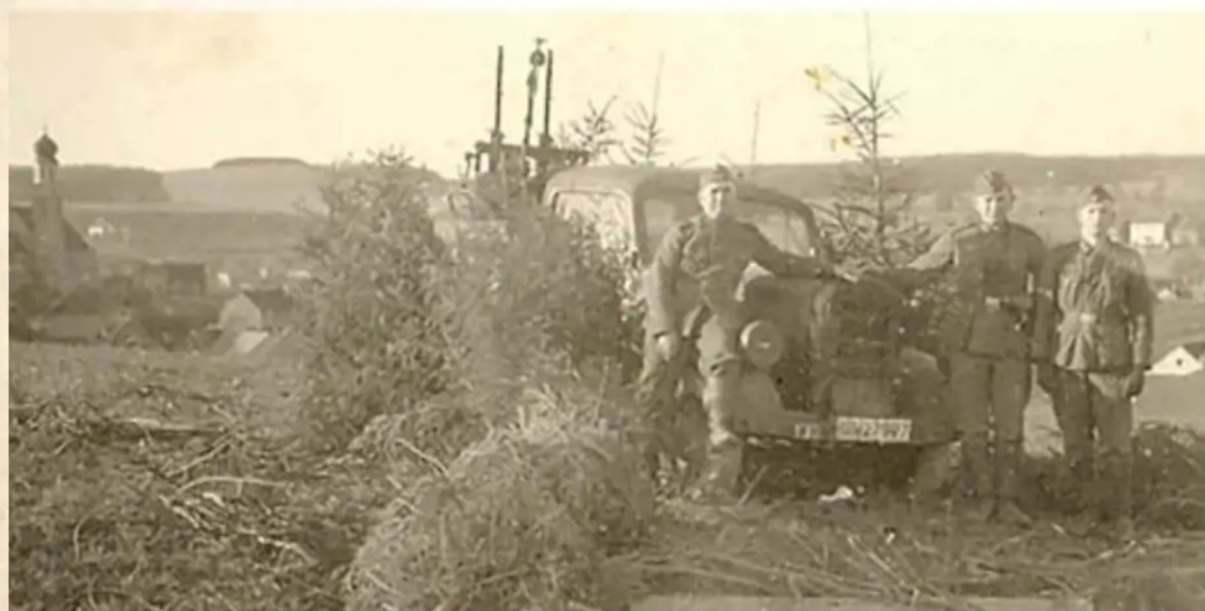
This field-converted flak truck is made up of an Opel Blitz 1.5 ton truck with a Zwillingssockel 36 pedestal mount type 36 for twin MG34 machine guns mounted in truck's load bed. The gun mount was probably removed from a previously horse-drawn infantry support wagon. As trucks became available in larger quantities after the capture of the BEF's and French army's serviceable transport stock, many infantry units were upgraded from horse-drawn to motorized and this type of conversion became common place. The photo is taken just inland of the coast somewhere within the Pas-de-Calais, France, in June 1940.
