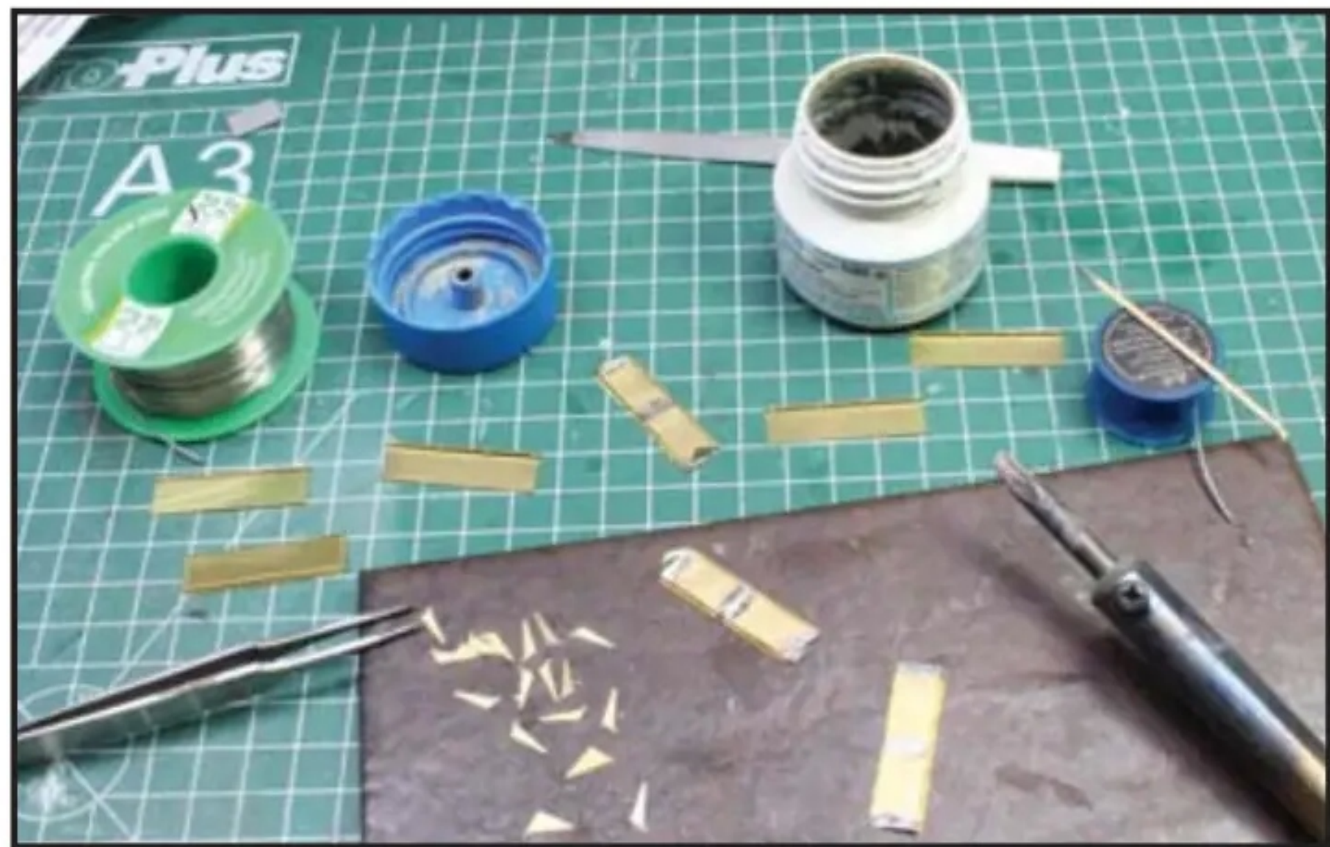
Soldered etched fenders can be bent easily. With superglue, however, everything would fall apart.
