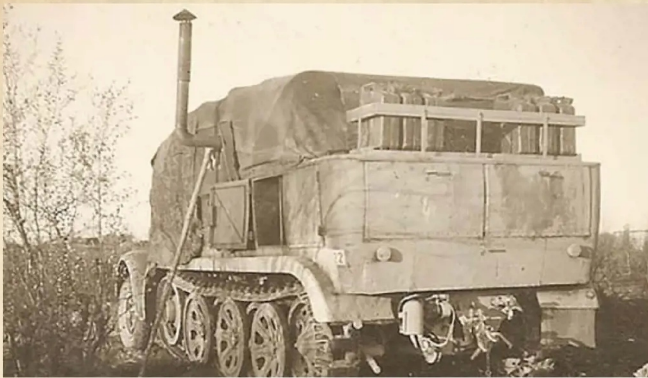
This is an interesting view of a Sd. Kfz. 7, a vehicle in Russia in the early summer of 1942. Of note is the installation of a wood-burning stove in the rearmost seating area, not an approved or standard addition but I bet the crew were very grateful for it during the winter that had just passed. Note the starting engine heater mounted on the rear bulkhead of the chassis, with its gas tube wrapped around the tow cable rollers.
