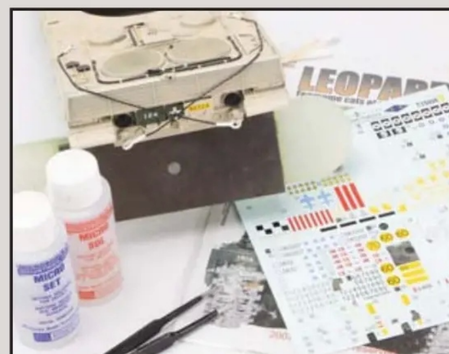
Echelon's decal sheet T35008 provided the markings required. The Micro Set / Sol helps to soften and set the markings in place.
