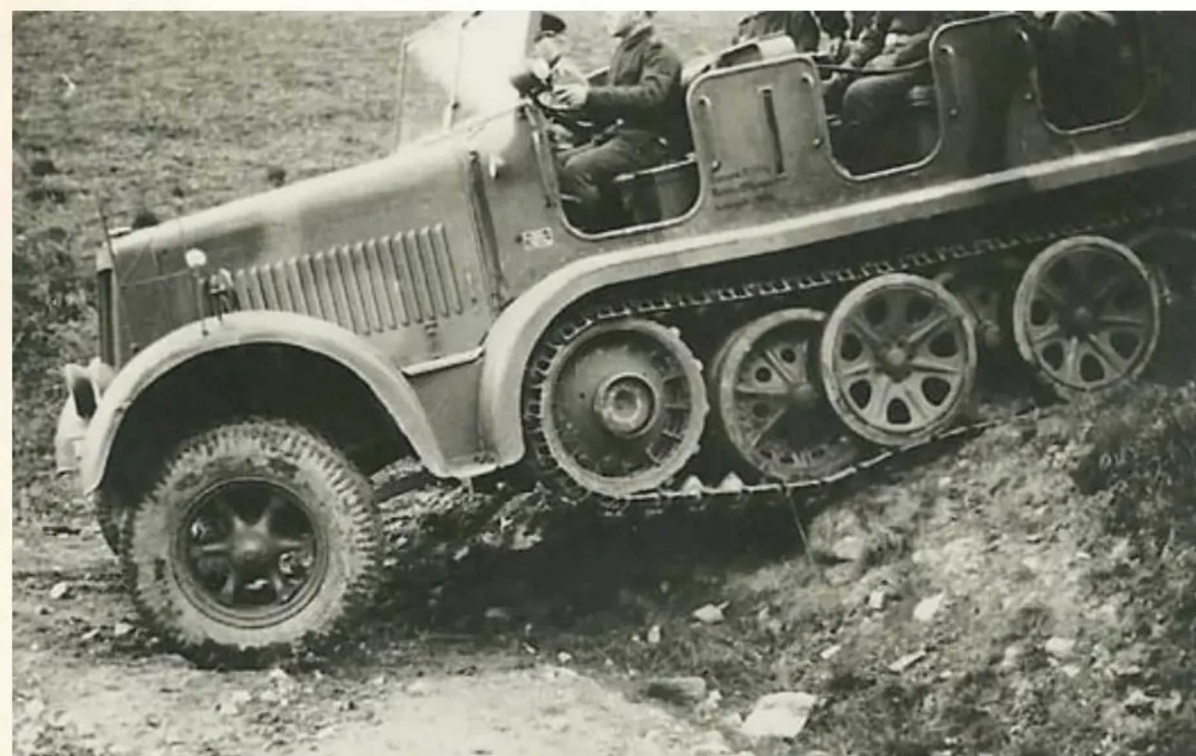
In this clear side view of an Sd.Kfz. 7 KM m 11 that is seen climbing down from an embankment at the side of a road we can see the maker's plate that is located on the firewall covering panel above the main drive wheel, also visible is the stencilled-on shipping data on the side panel just behind the driver
