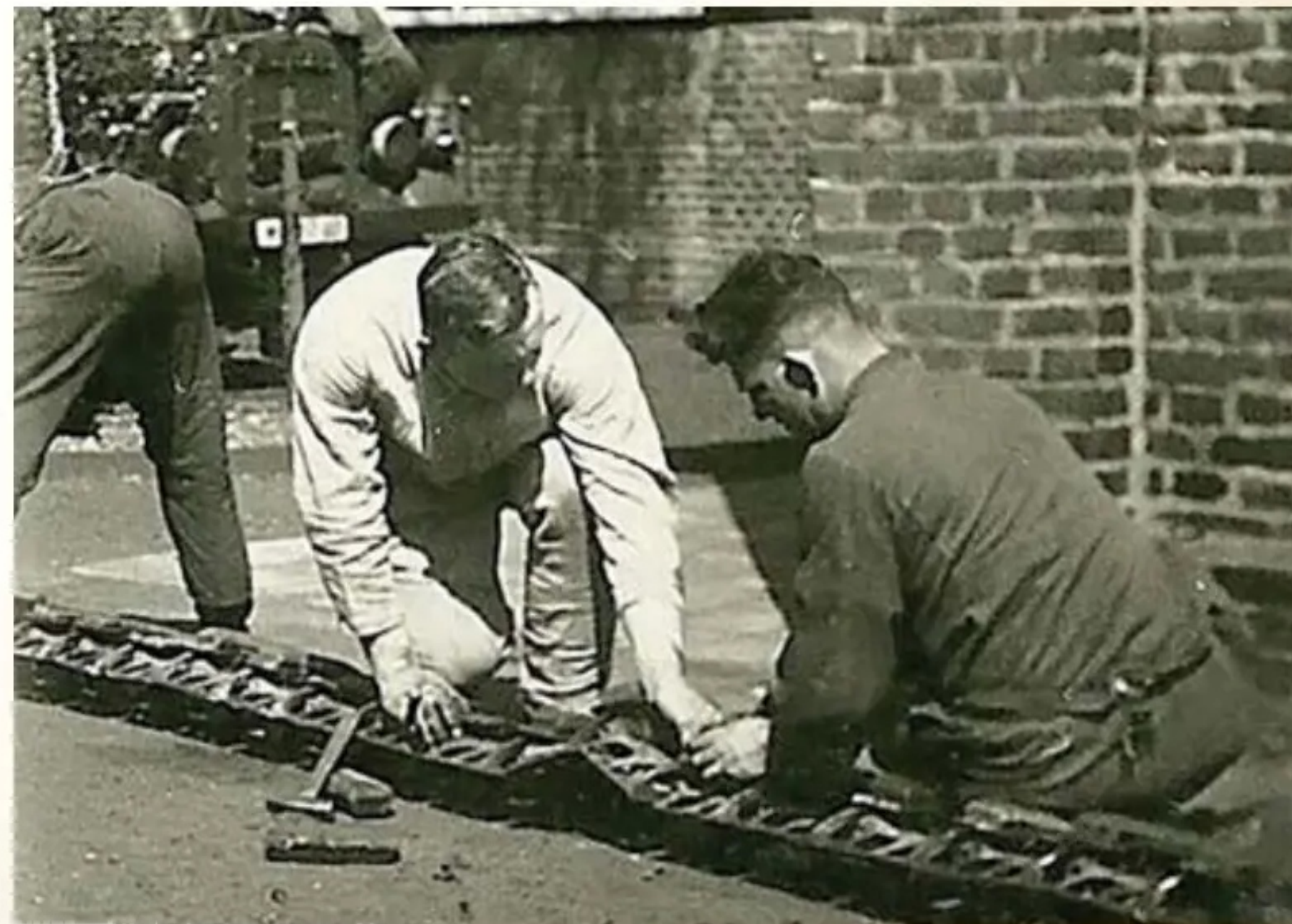
In the same commandeered French farm yard as mentioned earlier on this page we see maintenance crew giving the tracks of an Sd.Kfz 7 a thorough going over no doubt cleaning the tracks replacing all the damaged Greece nozzles and lubricating all the as required this took quite a while and was the most time consuming regular maintenance task on the normal crew task list and was rarely carried out with as much diligence as it should have been hence scenes like this.
