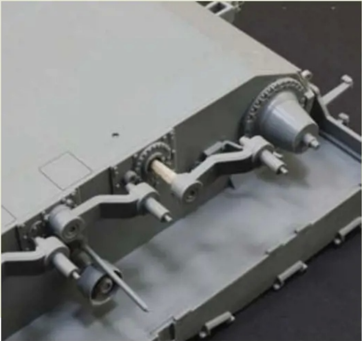
To facilitate the proper positioning of the chassis elements, I removed the limiting pins and thus each swing arm could be freely positioned on uneven ground. To be sure, I glued a piece of toothpick into each trailing arm which stabilized their mounting in the holes in the hull.
