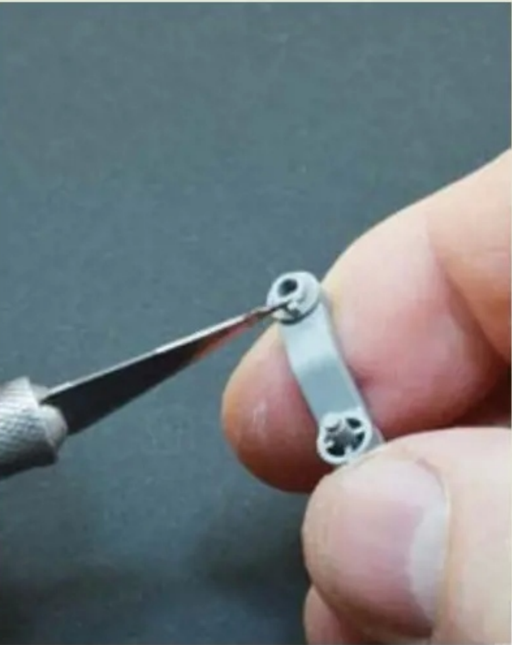
To facilitate the proper positioning of the chassis elements, I removed the limiting pins and thus each swing arm could be freely positioned on uneven ground. To be sure, I glued a piece of toothpick into each trailing arm which stabilized their mounting in the holes in the hull.
