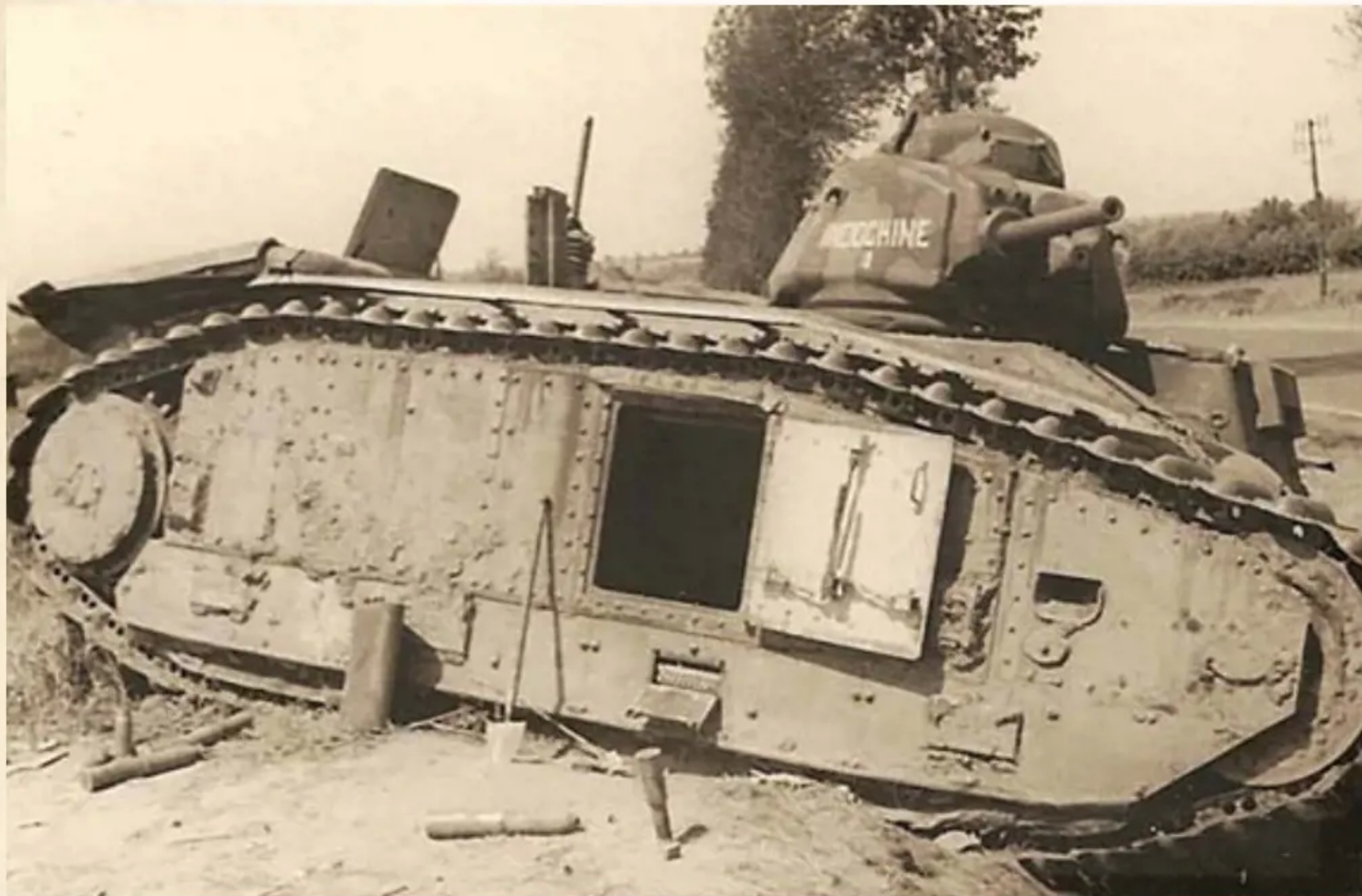
(Right) Torn apart by a single hit from a German 88 Flak 18 that hit this Char B1bis on the top side of the left-hand side track and splitting it apart the shot then glanced through the mud guard into the turret ring and exited the tank through the turrets right-hand side. This Char B1bis formally belonged to the 46th BCC and was another of the casualties of the fighting on the 28th of May north of Huppy; the 88mm gun was positioned behind cover afforded by Mont de Caubert.
