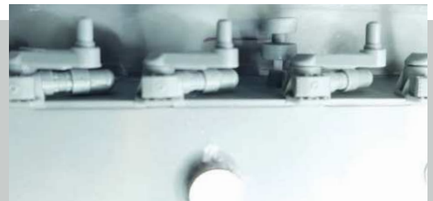
Suspension struts are mounted onto nub type fixings, ensuring alignment. Note the magnet glued to the hull bottom for use with the RP Toolz handle
