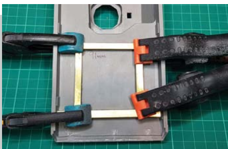
The first step is to reinforce the engine deck. Mine had a noticeable sag that I got rid of by bracing the inside with brass profile pieces.
