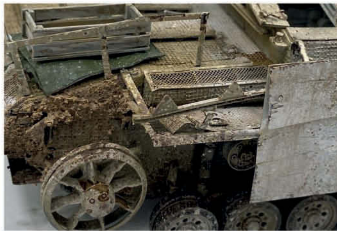
Note the heavy build-up of mud due to the missing section of fender.
