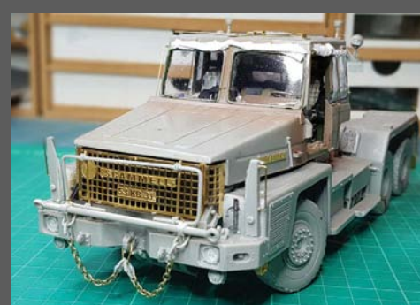
Test fit of the main component parts. Folded window screens are made from paper shaped with VMS Paper Shaper.
