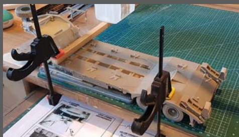
Once built I noticed that the trailer had a slight twist to it, so I clamped it in place and added weights to 'untwist' it. It was left like this for a week.
