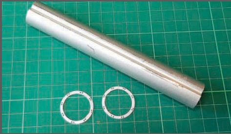
The trackway was manufactured from a metal tube with plastic bobbin ends.
