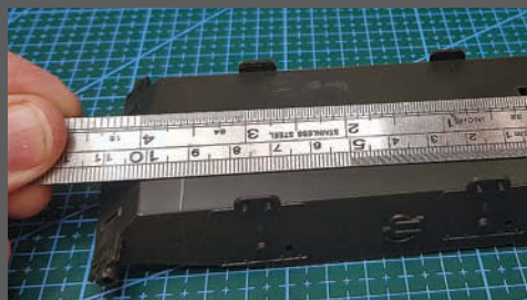
Measurements are provided to cut the front and rear from the Tamiya kit.
