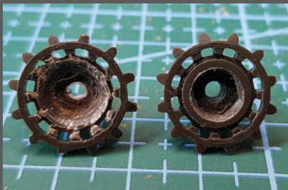
The Tamiya final drive sprockets need a bit of adjustment to fit on the conversion kit mounts.
