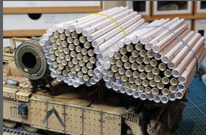
75 pipes per bundle. The inner pipes are paper straws supplied in exact 14cm lengths - perfect!
