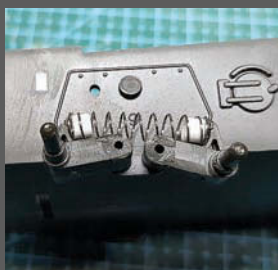
Suspension in place without cover fitted.
