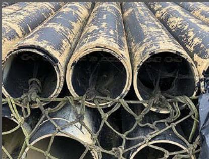
Note that 9 out of the outer pipes are reinforced with an inner pipe. Copyright Michael Osbourn.
