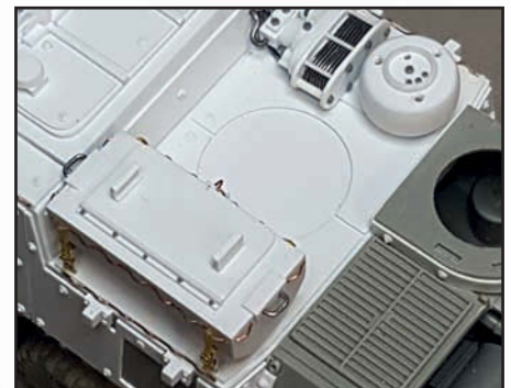
A drip tray was usually carried on the MRT and LAV as the Detroit Diesel was notorious for seeping oil. It was generally slung on the spare
