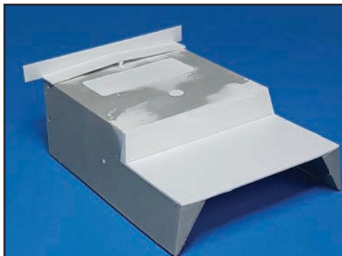
The surgery and amputations are done. The crane deck and rear compartment roof are roughed in. The air spotter hatch will butt up against the angled portion of the roof.
