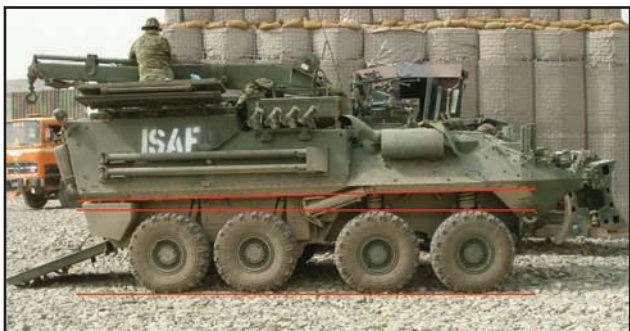
A good illustration of how the suspension is compressed on a Bison MRT, largely because of the additional weight of the crane. Photo credit: Anthony Sowards
