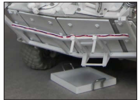
A drip tray was usually carried on the MRT and LAV as the Detroit Diesel was notorious for seeping oil. It was generally slung on the spare
