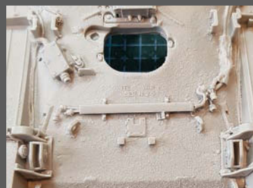
Casting number detail on the front hull.
