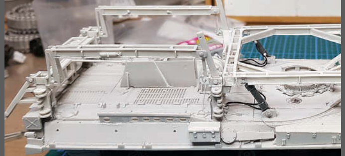
The rear frame is manually raised. The centre and front frames are hydraulically operated.
