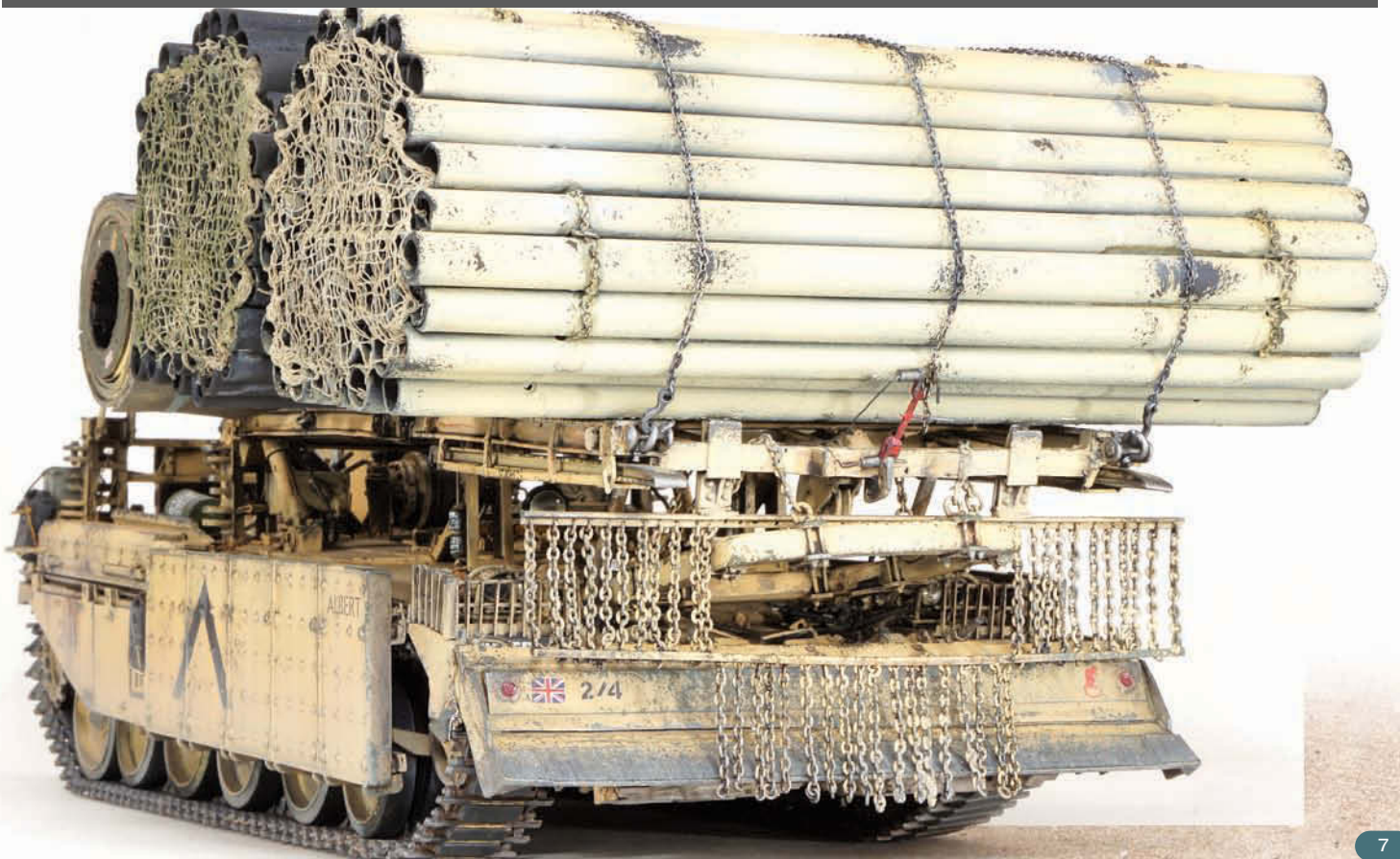
Note that 9 out of the outer pipes are reinforced with an inner pipe. Copyright Michael Osbourn.
