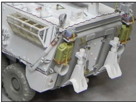
The rear of the hull is taking shape with new jerry can holders, detail added to the man door in the ramp, spade anchors and armoured covers for the rear lights. Visible on the roof is the rear fairlead for the winch and an equipment tie down strip.
