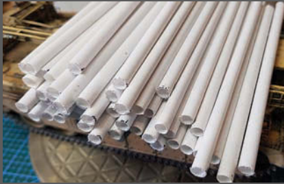
6mm tubes used for the fascine outer pipes.
