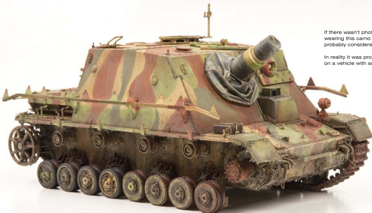
The brutish side-profile of the Sturmpanzer IV showing off the 'Late' production features of simplified upper hull, StuG III cupola and steel rimmed road wheels the most
