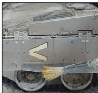
Again, I used a mix of weathering paint on the upper hull to apply some dust to the places least frequented by the crew. Also thanks to these paints I can build a contrast on the model. Note the nut and bolt used as a handle and fixing method for the turret.
