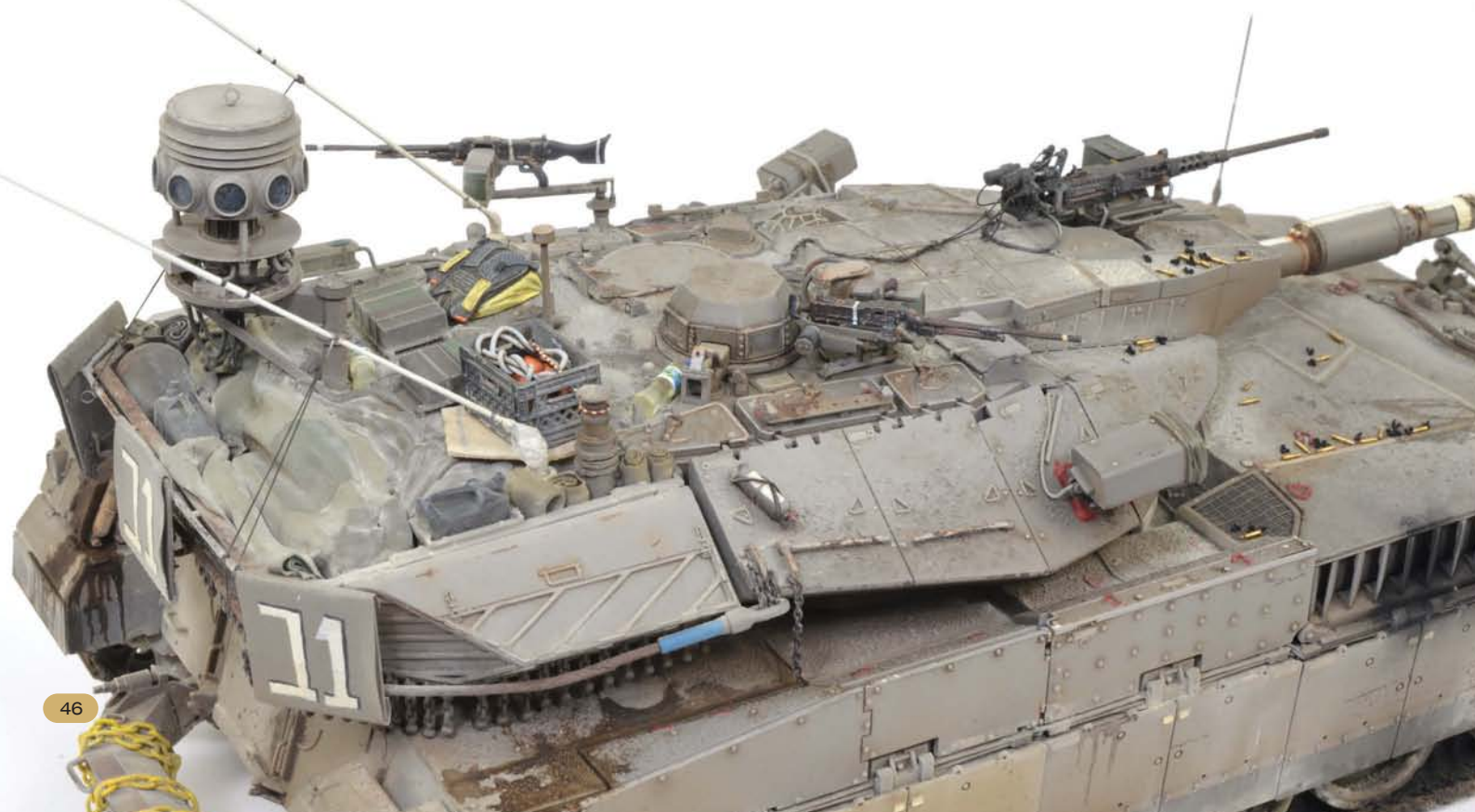
The sides of the hull as well as the horizontal surfaces are dusted with pigment.
