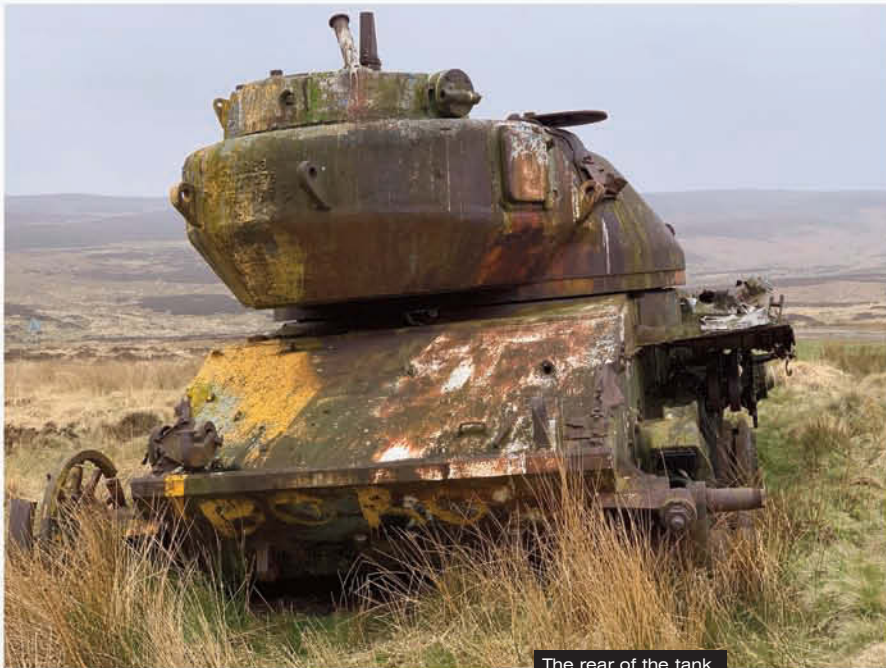
The rear of the tank showing white paint applied over the already rusting hull and bleached with further rust stains
