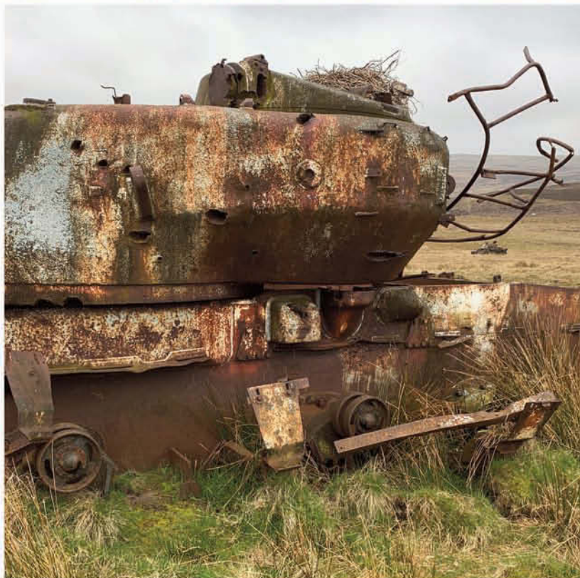
the remains of the engine with various types of material weathering in different ways.
