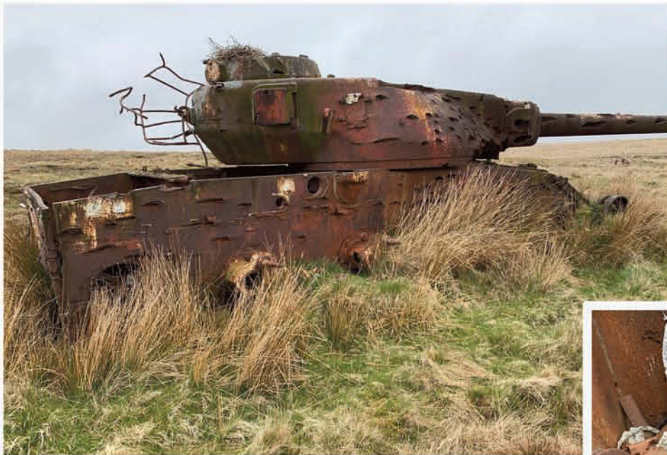
A Conqueror Mk1 Heavy Gun Tank devoid of almost all of its running gear and laying belly down on the peaty soil. The rear turret basket has been mangled from years of attacks. The engine compartment is full of all sorts of debris including the jumbled remains of the gearbox. The tank is one of the few features in the bleak landscape and as such has been made the home of a bird of prey who has nested on the commander's cupola. This is an indication of how seldom this particular target is used.
