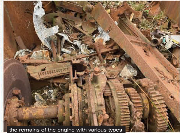
the remains of the engine with various types of material weathering in different ways.
