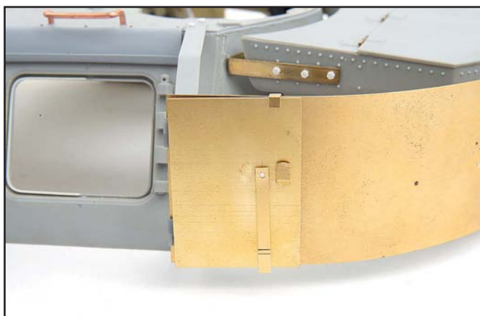
The simple latch system that holds the doors closed was added and detailed with plastic rivets made by pushing the blunt end of a drill bit into plastic card.
