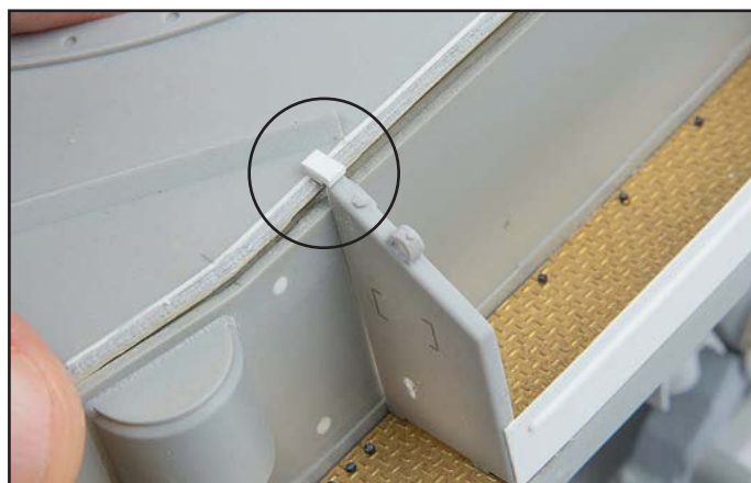
The mounting strap was replaced with plastic strip allowing the hull roof to be removed without affecting the wheel bin.
