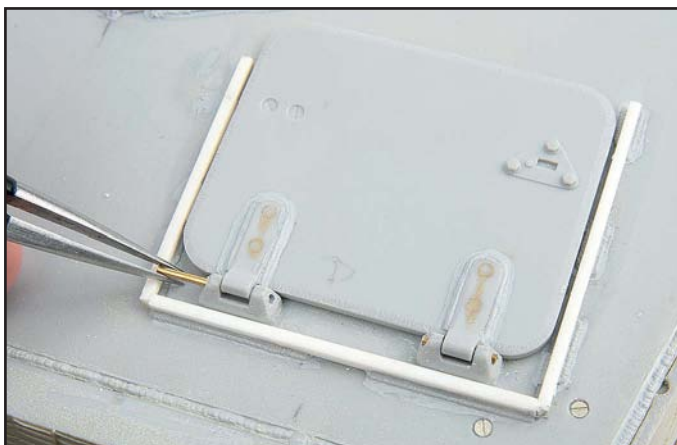
I drilled out the hinges and inserted 0.7mm brass tube into the hinge. I had to make some adjustments to the hinge tolerances to get them to be fully functional.
