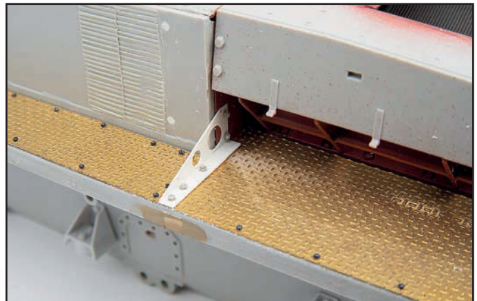
I made new track guard brackets from plastic card and MasterClub resin bolts.
