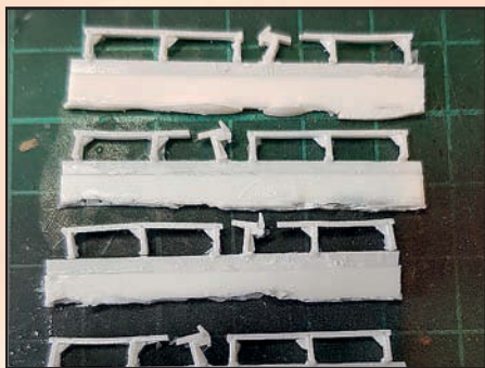
Tube rails and locks. Some warpage although nothing some hot water can't sort out.
