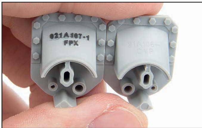
Although the kit bogie housings have moulded casting numbers they are very poorly defined and they do not have the correct numbers for left and right. (106 for left, 107) for right. I used printed numbers to replace the casting numbers for a mix of manufacturers.
