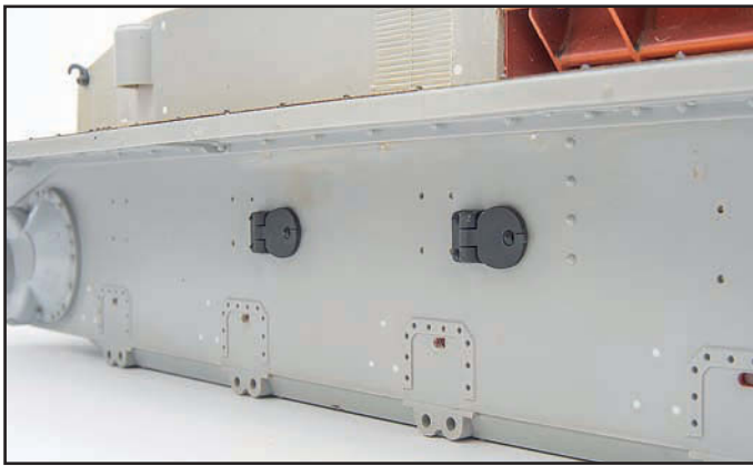
The new printed covers were glued into position on the hull.
