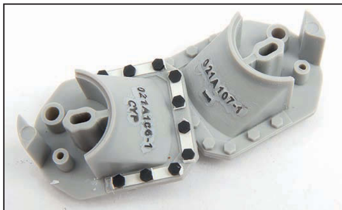
Many preserved bogies show locking tabs used for the fixing bolts so I removed the kit bolts and made locking tabs from 5 thou plastic strip. the bolts were then refitted with printed bolt heads.
