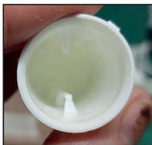
Rails are fitted inside the tubes. The false bottom can be seen here and should be painted black.
