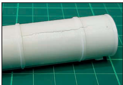
Each launcher tube is made up of 3 parts. Some clean up and sanding is required, although this area will be on the bottom side.
