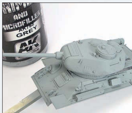
I primed the model with a couple of thinly sprayed coats of AK Fine Grey Surface Primer.
