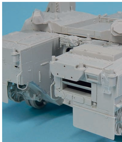
Note the centre position of the access door providing protection for crew dismounting. Clear parts are provided for lamps and optics.
