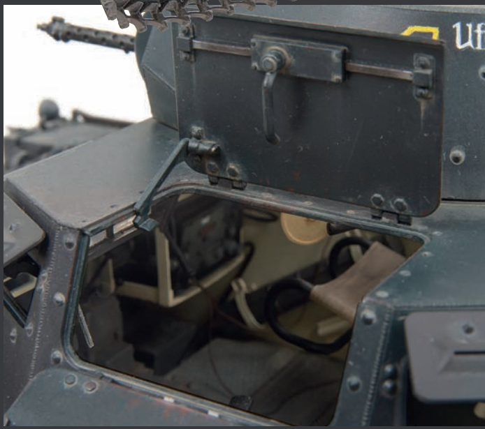
Above The hatch stay is not provided in the kit so I made one from plastic card.
