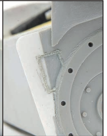
Creating the interlocks was a bit of a challenge. I marked out the shape and cut the outline with a P cutter. I used a motor tool burr to remove the section and then cleaned up the rebate with micro chisels. Finally the welds were added using Magic Sculp.
