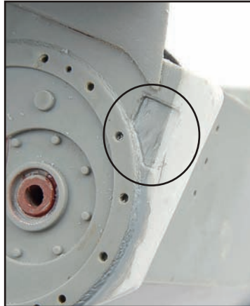
Creating the interlocks was a bit of a challenge. I marked out the shape and cut the outline with a P cutter. I used a motor tool burr to remove the section and then cleaned up the rebate with micro chisels. Finally the welds were added using Magic Sculp.
