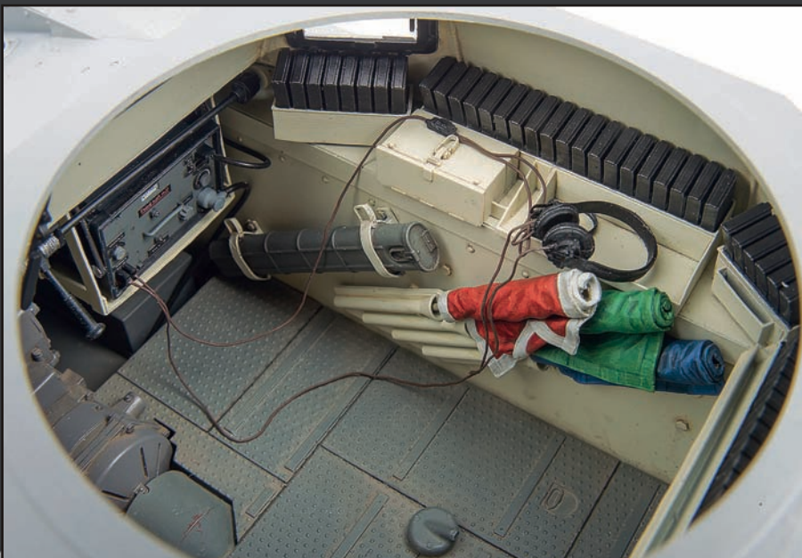
Above Headphones and throat mic were glued into the hull before the top went on but I had to connect them to the radio once the top was in place.
