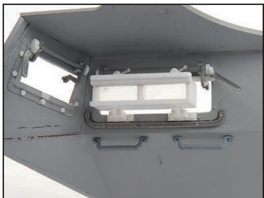
The Driver's vision block is a more elaborate arrangement. I scratchbuilt the vision block using spare clear blocks from my Panzer IV. Again the kit visor hinge was used with additional detailing and lead solder was used to form the curved rubber strip at the bottom.
