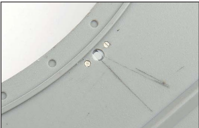
On the outside the hole is squared off and there are two recessed screw heads.
