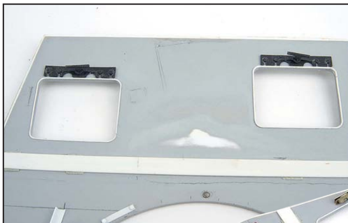
The front hatches have a quick-release system to allow the hatches to be jettisoned in an emergency. I scratchprinted the quick-release brackets
