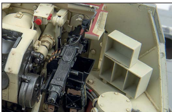
Time to tie up a few loose ends around the interior. The spare vision block rack needed to be completed and had been sized using the Cupola vision blocks as a starting point.
