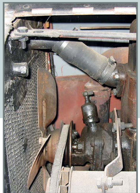
Stoewer's AW2 ohv, 2.0-liter, 50-hp, water-cooled, four-cylinder petrol engine.
