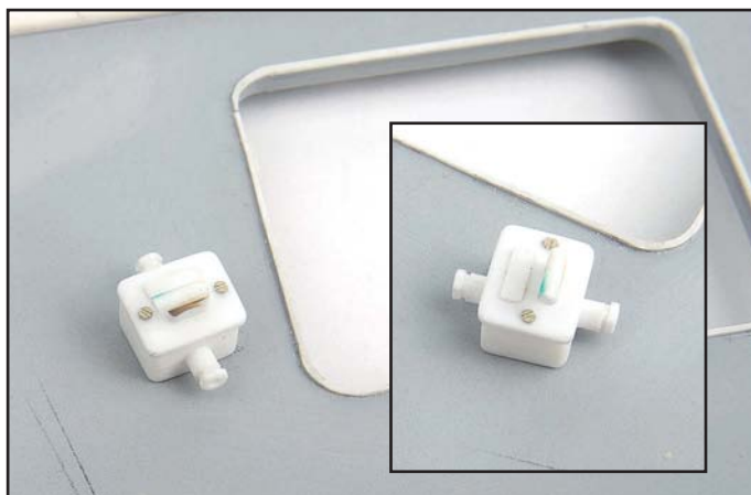
The antenna cable junction box was made from plastic card. It has a socket to plug in the connecting cable if the radio sets are not plugged in which is very useful for the removal of the roof so I added the plug on the front of the box.
