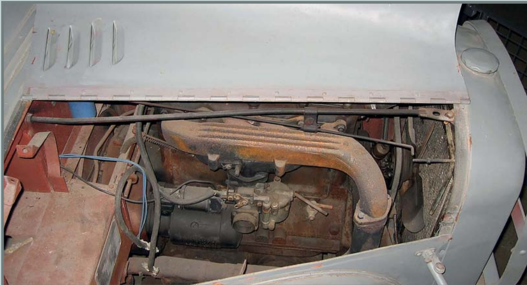
Stoewer's AW2 ohv, 2.0-liter, 50-hp, water-cooled, four-cylinder petrol engine.
