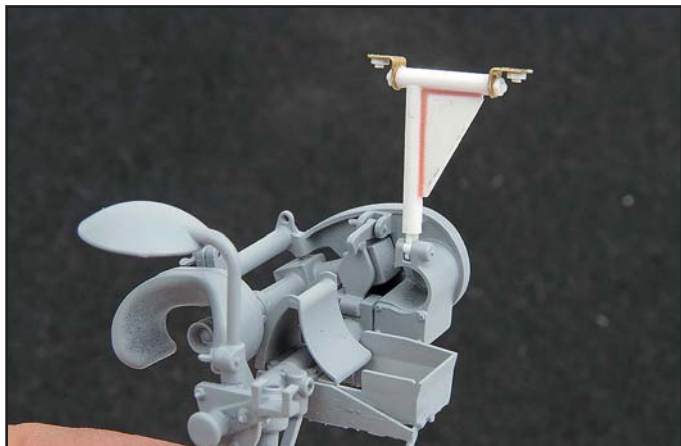
The travel lock for the bow MG was simple enough to construct from plastic rod, card and some brass sheet.
