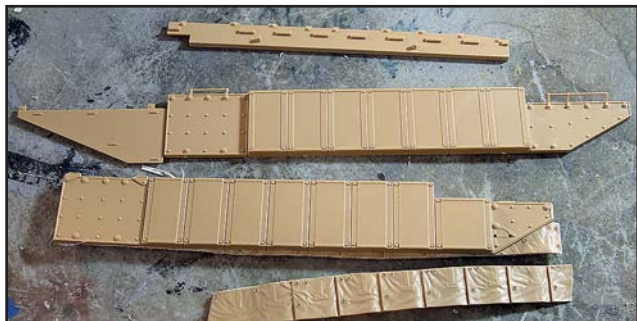
Plastic sheet is used to fill in the portion of the sponsons that will be visible as well has filling in motorization openings.
