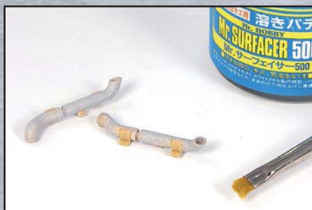
For the exhaust system I created a realistic texture with the help of Mr.Surfacer 500. Before that the plastic was roughened a little and covered with revell glue.
