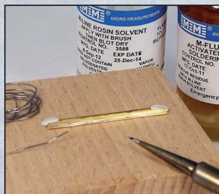
I joined the first etched parts for the front suspension by soldering for strength.
