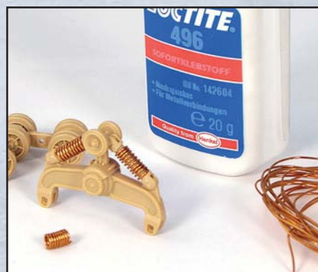
The springs of the suspension have been refined with 0.6 mm thick copper wire.
