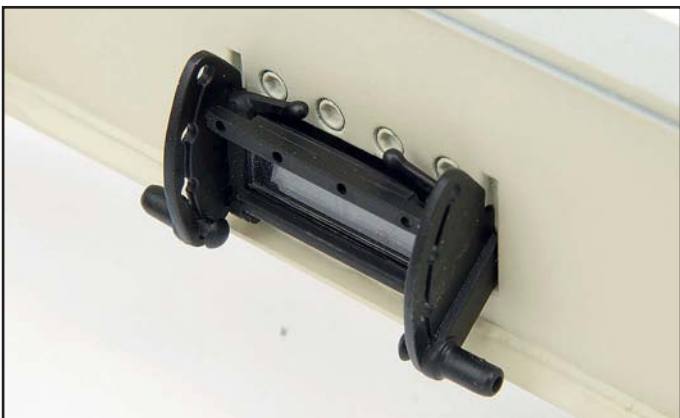
The visor was then glued into place inside the hull.
