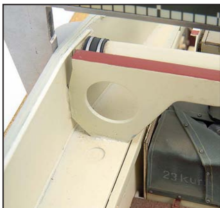
5 minute epoxy doesn't always give the neatest finish but in this case I needed its strength to hold everything in position. I accidentally managed to strip the paint from a patch of the sidewall with a glue laden brush in the
