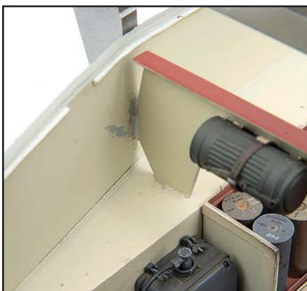
5 minute epoxy doesn't always give the neatest finish but in this case I needed its strength to hold everything in position. I accidentally managed to strip the paint from a patch of the sidewall with a glue laden brush in the
