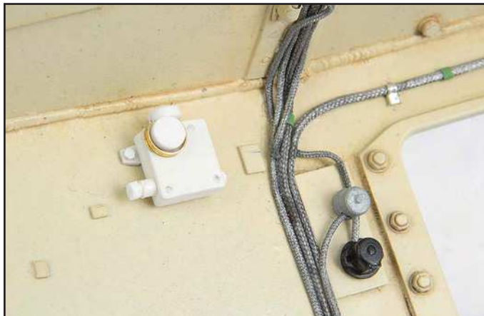
I needed to make the emergency stop button which cuts off the power traverse for the turret. The square shaped box was relatively simple to construct with some scrap photoetch for the circular ring.
