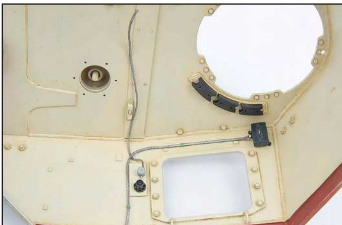
The layout of the cables takes some careful planning as here were the four way connector has been added above the power socket and its cable threaded behind the intercom cable.
