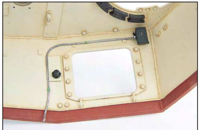
The first of the cables were added using the ANYZ chord with coloured rings added showing green for the intercom system. Note also the power socket added to the left of the hatch.
