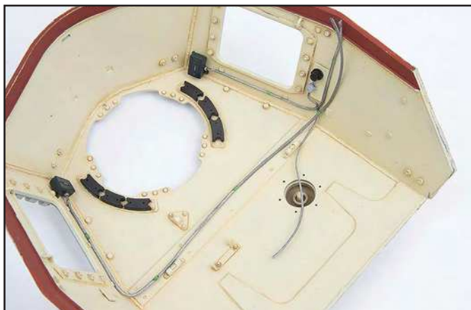
The other intercom cable runs back across the turret roof and is loosely laid in place here.
