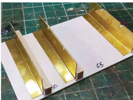
The etched brass brackets are provided in the kit, just glue them at the right lengths to make the chassis jig.
