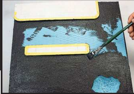
A layer of acrylic resin was applied to simulate the asphalt.
