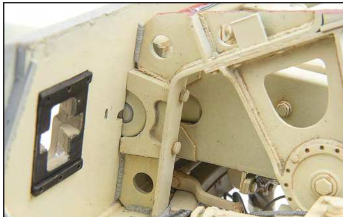
I added the missing welds to the braces which needed to be done before these areas became inaccessible. I used Magic Sculpt to create the welds and they were painted to blend in with the existing weld details/
