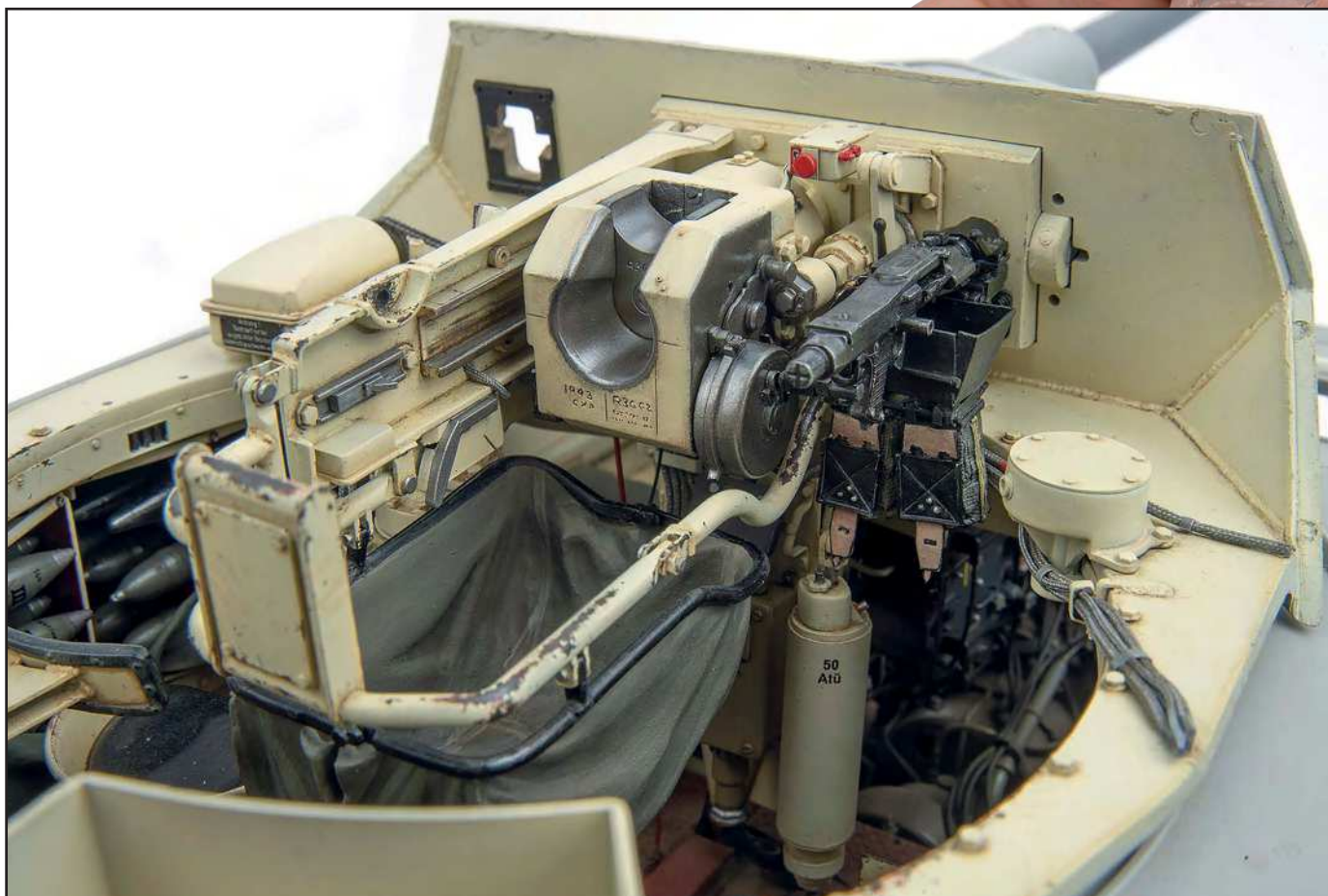
Next the remainder of the co-axial fire control system was added, beginning with the arm 6 onto which I had glued a small piece of Albion Alloys brass tube 7 . I was then able to insert a pre-sized brass rod which connects to the trigger of the gun. All this is almost entirely hidden once the MG is installed so has to be added now. The co-ax assembly is then fitted and the lower buffer 8 glued into position beneath it. From this angle the trigger control rod is just visible behind the buffer mount.
