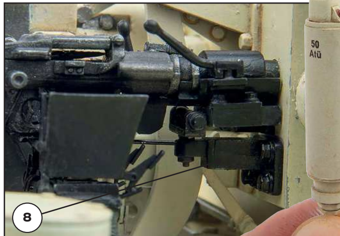
Next the remainder of the co-axial fire control system was added, beginning with the arm 6 onto which I had glued a small piece of Albion Alloys brass tube 7 . I was then able to insert a pre-sized brass rod which connects to the trigger of the gun. All this is almost entirely hidden once the MG is installed so has to be added now. The co-ax assembly is then fitted and the lower buffer 8 glued into position beneath it. From this angle the trigger control rod is just visible behind the buffer mount.
