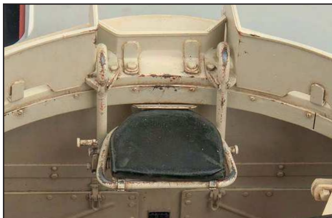
Using the same techniques as before I added some areas of wear to the turret ring below the turret side hatches where the crew would enter the turret. Similarly the Commander's seat was treated in the same way and his seat cushion was given a suitably grubby appearance with an acrylic wash.
