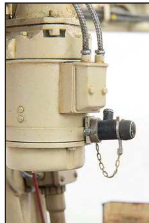
plugs into the end of the existing socket. I used some flexible resin to make the cable as it will sag naturally but a suitable wire would work just as well. The trigger is fitted to the ring on the base of the motor housing. The connection point for the cable has been pre-drilled
