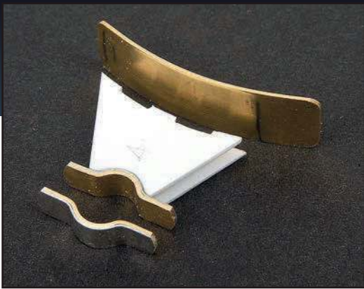
The angled leg of the turret support makes for some complex geometry for the backrest. With no plans I had to judge the shape of the bracket by eye. The backrest is offset and angled when fitted to the bracket.
