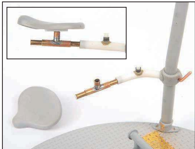
The loader's seat is mounted on one of the turret basket legs. The seat bracket was completely replaced with Albion Alloys slide fit brass tube combined with plastic rod. The seat itself was reshaped with a raisedommel at the front made with Magic Sculp.
