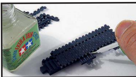
I applied a drop of adhesive to keep them in position. Careful not to overdo it with the glue otherwise you may also bond the links together.
