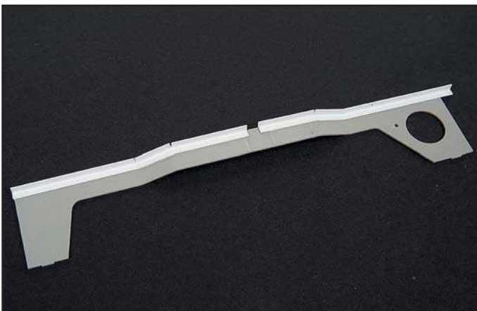
I removed the old centre support and I used 'L' profile strip to add the missing bracket along the top edge of the cross beam.
