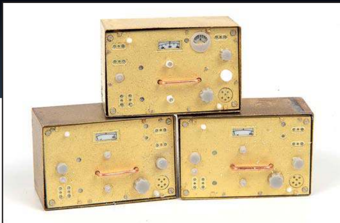
The radio facias were detailed using ABER screw heads and dials shaved off the kit radio sets.
