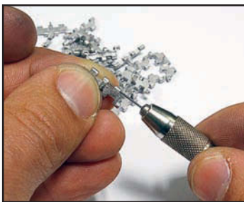
Frills are best treated to a 0.5mm drill run through the pin holes.
