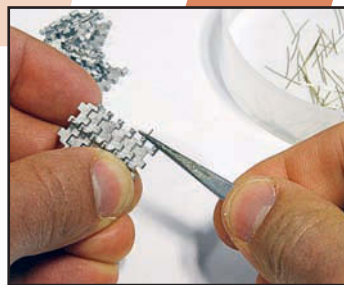
The pins slide easily into place, a dot of CA glue in the hole keeps them in place safely.
