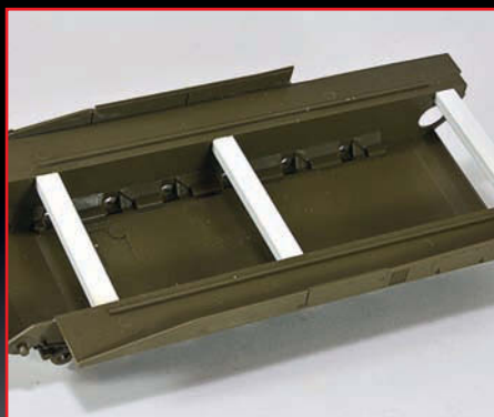
I added reinforcements to the hull because a side of the structure was cut away making the alignment difficult.
