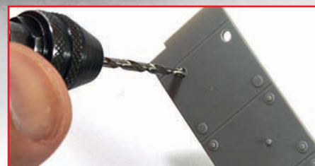
Taking the time to get the details exact I drilled all the raised bolt heads and replaced them with recessed ones
