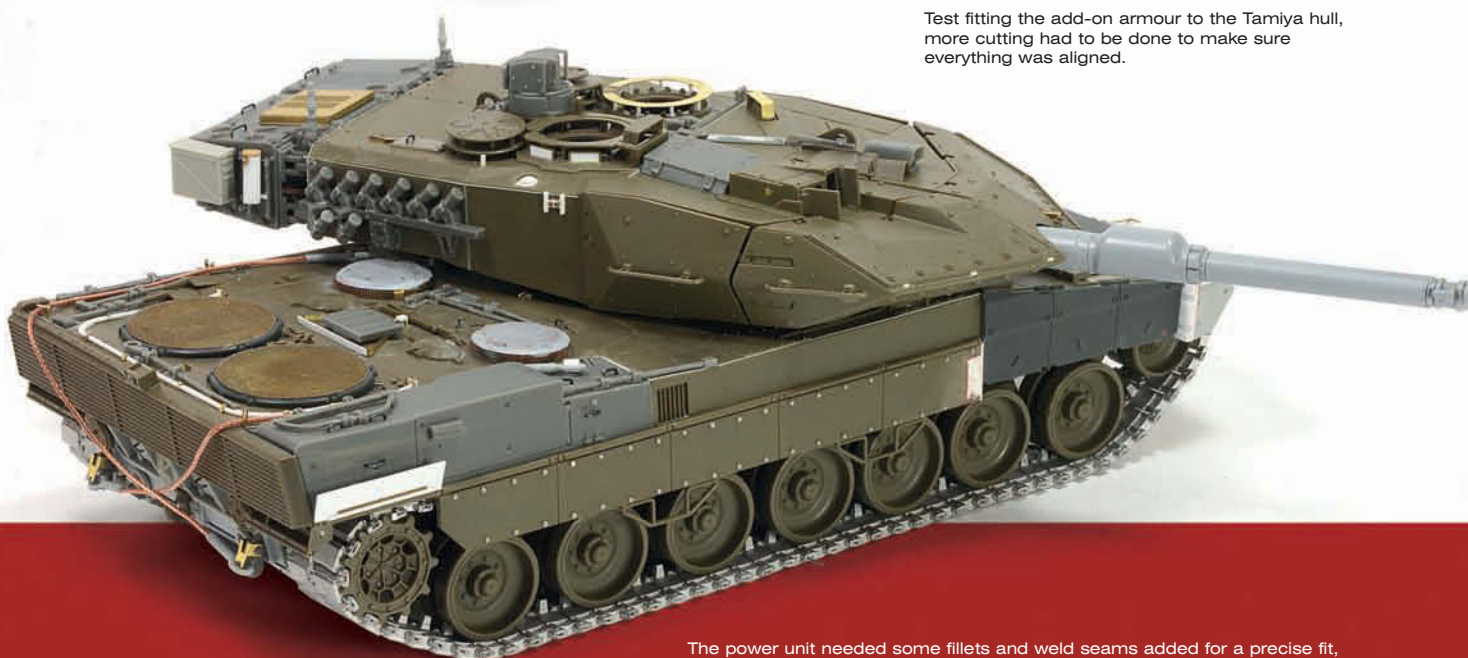
The power unit needed some fillets and weld seams added for a precise fit, once in place it really looked the part.
