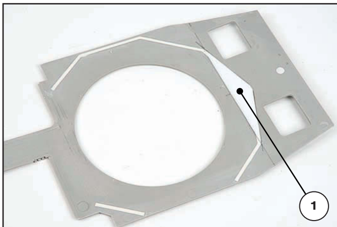
Having cut out the hull roof it was time to tidy this up with the recesses for the splash guards filled with white Milliput. The large void 1 between the front hatches where the splash guard is moulded into the roof was filled with a sloping piece of plastic card.
