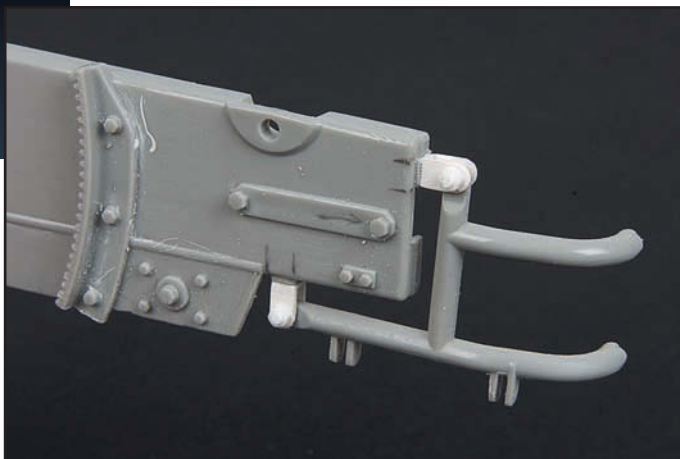
The hinges on the tubular guard were sanded off and the pegs shaped to fit into the new hinges.
