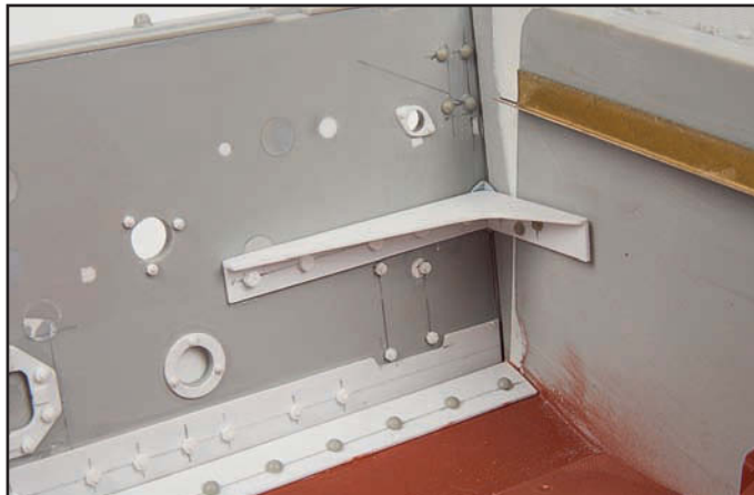
Whilst I was working in this area I made the pair of corner braces which join the hull rear to the sides. The kit parts are rather too thick and not quite the right shape.
