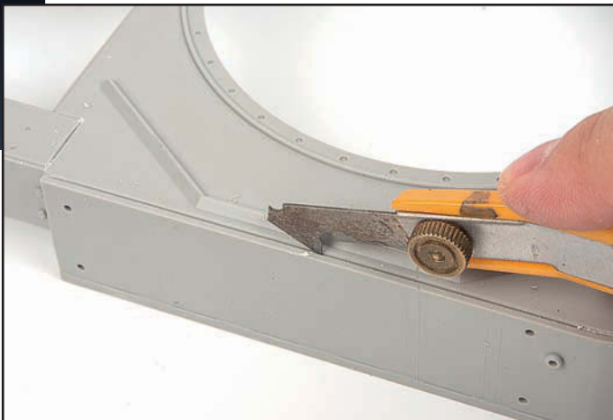
After much consideration and prevarication I decided to cut away the hull roof to provide the maximum access to the completed interior. I used a P Cutter to open up the big front weld beads.
