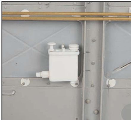
Next on the list of engine bay jobs was the primer pump unit for the cold weather start system which is mounted on the firewall. I could judge the size of the mounting bracket for the pump against the firewall opening but somewhere along the way I neglected to double check my sizes for the pump. I wasn't until I had completed making the pump and then positioned it
