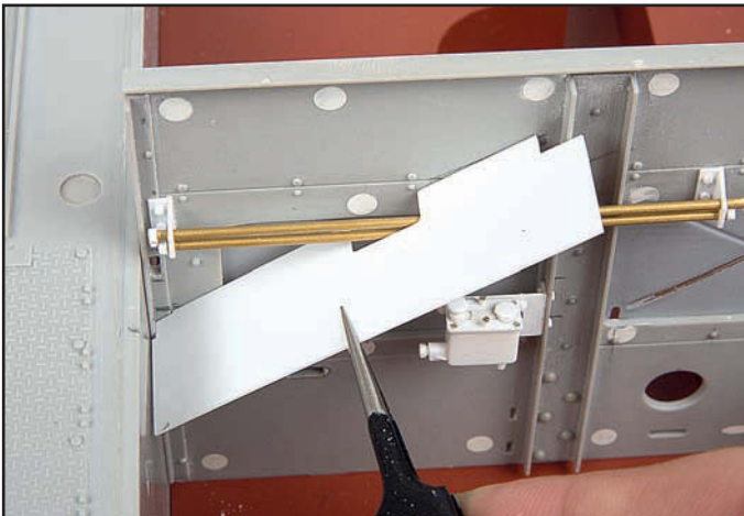
To ensure that the radiators operate efficiently the surrounding areas of the engine bay were sealed off with sheet metal panels. The biggest one is mounted onto the firewall and some trial and error test fitting was needed to establish the size.
