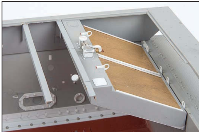
The radiators are test fitted with the new beams to check alignment as accurately as is possible with so many loose dry fitted parts.
