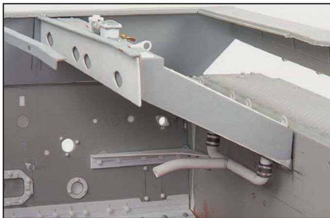
Water pipes run from the base of the radiators across to the water pump on the engine. Most of the space under the radiators is filled by the generator so it is vital to check that everything fits so nothing is fixed yet.
