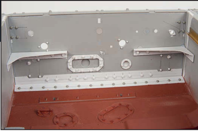
Both corner braces will be fitted later in the project to maintain unrestricted access through the back of the hull when the rear panel is removed.
