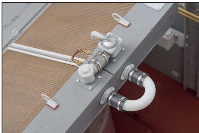
The connecting pipes which join the two radiator units was constructed using plastic rod, heated over a candle flame to bend the rod. Lead foil was then used to make the coupling sleeves.
