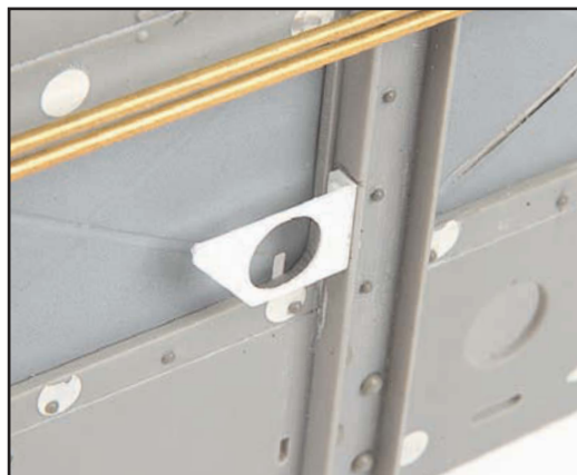
the new version. With the pump completed I made the pleasingly simple mounting frame which bolts onto the central firewall beam.
