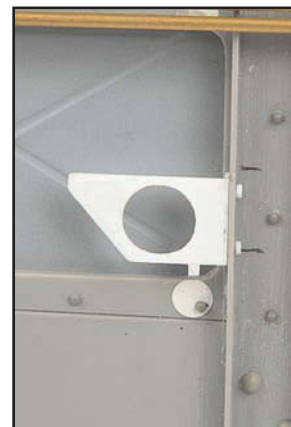
the new version. With the pump completed I made the pleasingly simple mounting frame which bolts onto the central firewall beam.
