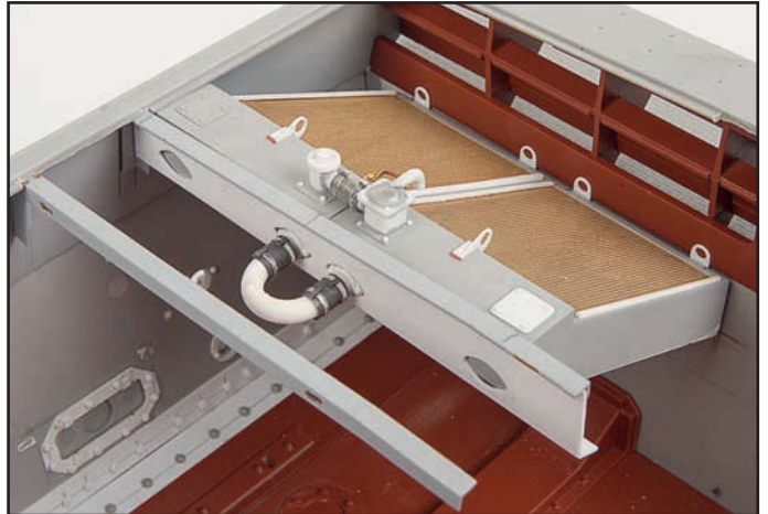
With the radiators dropped into position the connecting 'U' pipe is test fitted through the radiator support frame.
