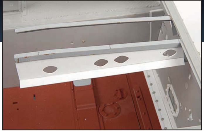
The corresponding upper mount for the radiators was constructed from plastic sheet the diamond-shaped holes are to allow the water pipes to pass through the frame and connect to the radiators.
